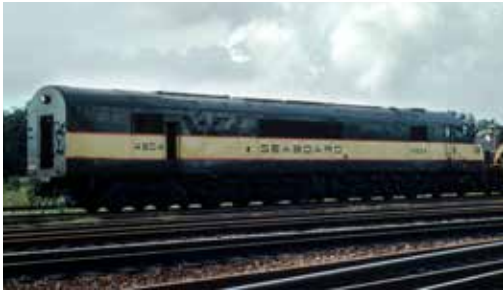
Seaboard Air Line 4504 shows the tapered rear of the Centipede units at Wildwood, Fla., in 1949. W. B. Cox, Krambles-Peterson Archive
