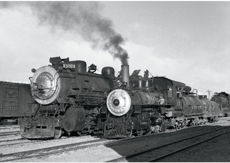
At the point in Owenyo where slim- and standard-gauge rails met, SP No. 3203, a husky 1911 Baldwin 2-8-2, dwarfs narrow-gauge 4-6-0 No. 18. Walter H. Vielbaum
