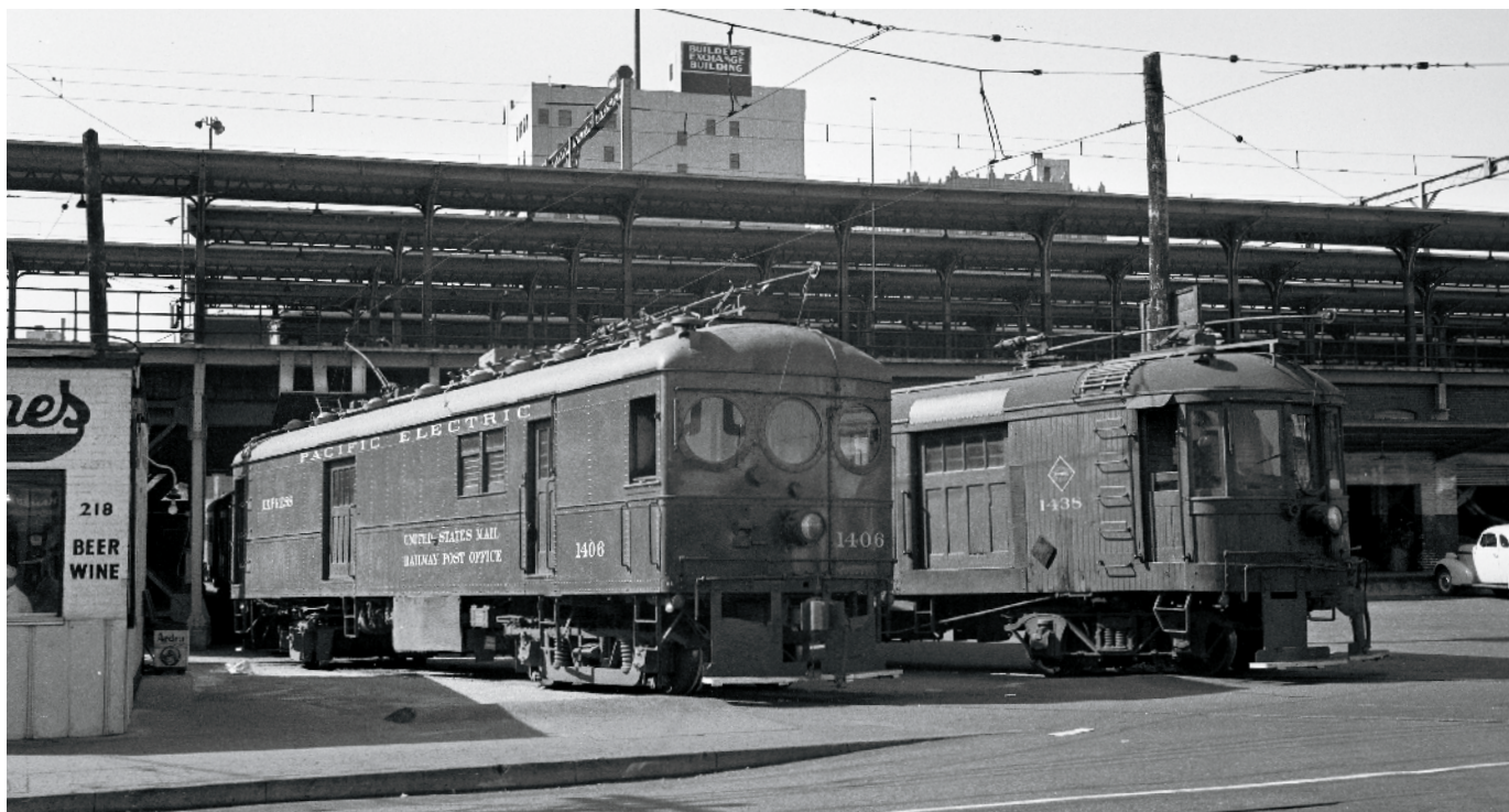
Pacific Electric's diverse roster included all-steel and wooden box motors used in postal and express freight service. Two of the motors pose at the 6th and Main station in Los Angeles. RPO 1406 originally was one of three Brill cars on the Portland, Eugene & Eastern. Walter H. Vielbaum
