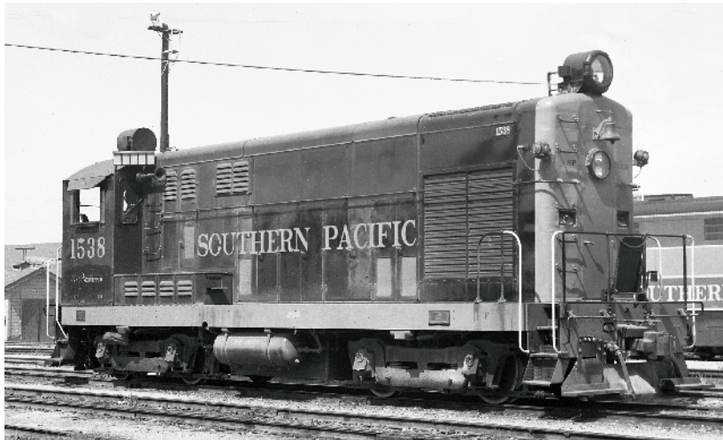
Also on June 10, 1958, black-and-orange Fairbanks Morse H12-44 No. 1538 held down switching assignments at San Luis Obispo. The SP unit was one of 10 such equipped with M.U. gear. Robert P. Townley
