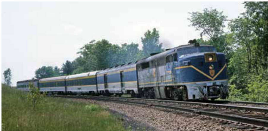
Delaware & Hudson PA16 sweeps along the main line north of Mechanicville, N.Y., with a four-car consist: baggage, buffet-bar, coach, and New York Central parlor.
