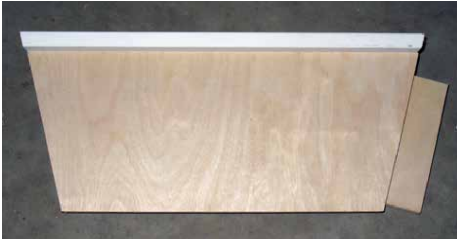
1 Panel components. Each trapezoid panel includes a plywood splice plate and fascia. The fascia extends above and below the benchwork.
