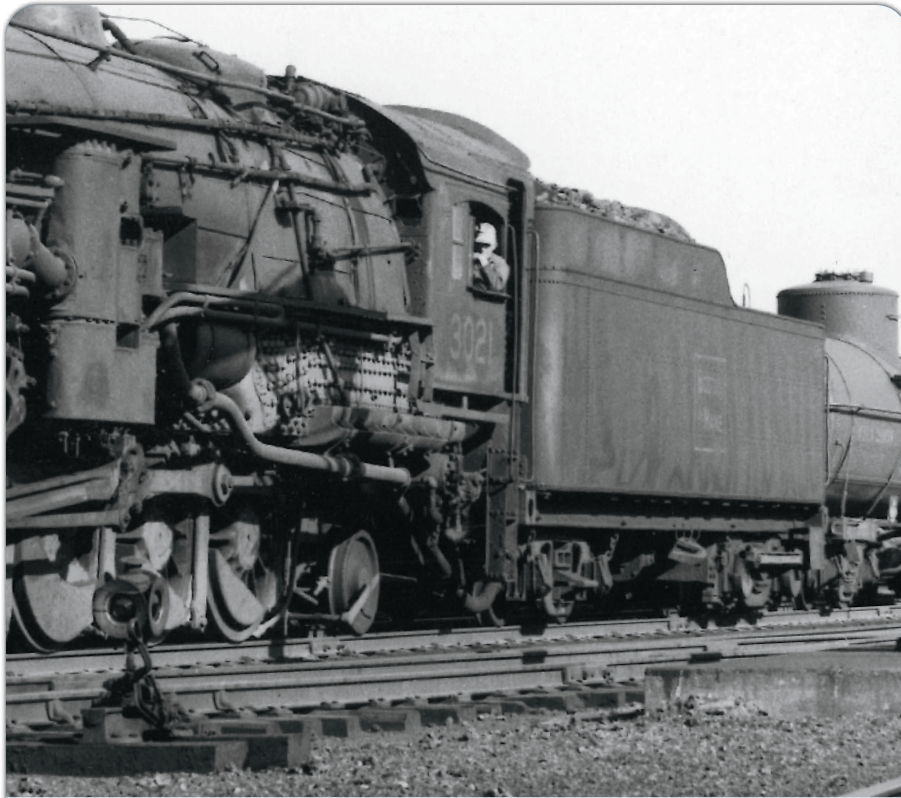
A Boston & Maine 2-10-2 steam locomotive is seen at Worcester, Mass., in an undated photo. The tender's rear truck looks a little different from its front one because it's a booster engine, an auxiliary locomotive designed to turn the main locomotive's excess steam at slow speeds into extra traction to help get the train started. H.F. Harvey photo
