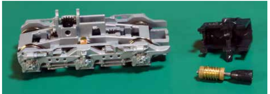
2 Ron removed the gear tower enclosure and the worm gear. He trimmed the plastic gear housing to make room for the motor and DCC decoder.
