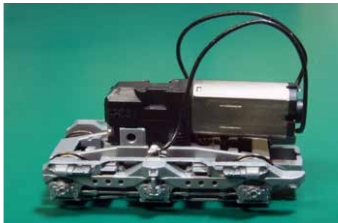
4 After mounting the motor and worm gear to the truck, Ron hooked up the motor leads to the truck's power pickups and tested it with a DC power pack. It ran.
