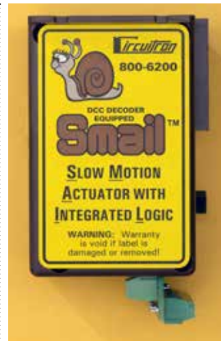
2 The SMAIL circuit board is a little longer than the one on a Tortoise to accommodate a pushbutton, a status LED, and a three-terminal connector.
