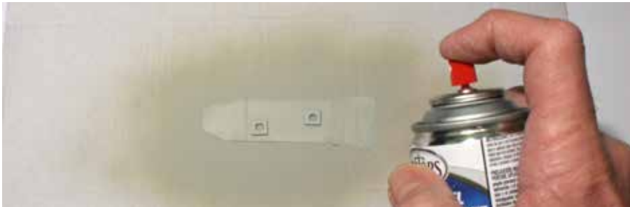
③ Tom cut two pieces of .060" styrene to the same size as the crossing pedestal base. After drilling a \frac{3}{16} " hole in the center of each piece, he spray-painted the styrene with Testor's gray enamel.
