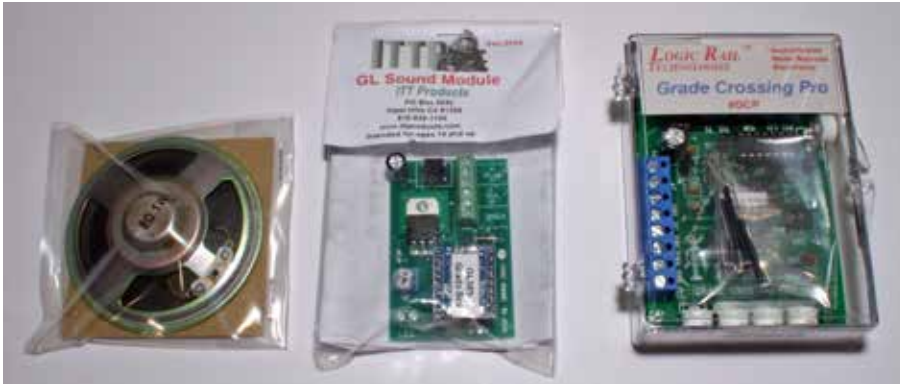
② The Logic Rail Technologies Grade Crossing Pro includes the flasher circuit and train detection system. The ITT Products GL Sound Module activates the bell.
