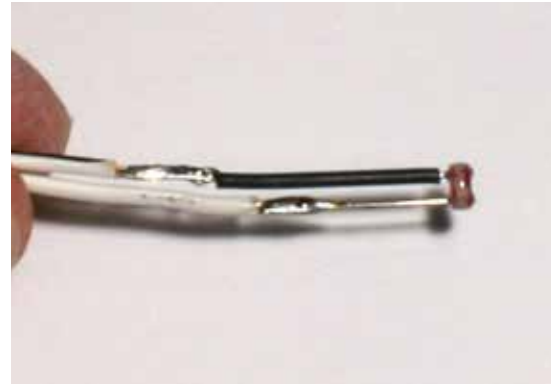
13 To offset the solder points on each leg, Tom attached a length of 22AWG wire. He covered the solder joints to prevent short circuits.
