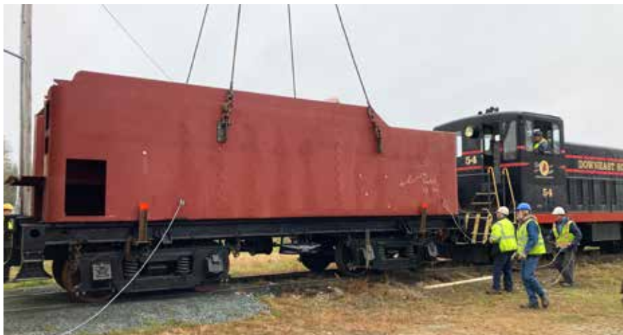
On Nov. 13, 2022, the newly fabricated cistern and coal bunker is lowered onto the original tender frame of the last steam locomotive to operate on the Maine Central. Nonprofit New England Steam Corp. plans to run No. 470 on the Downeast Scenic Railroad.
