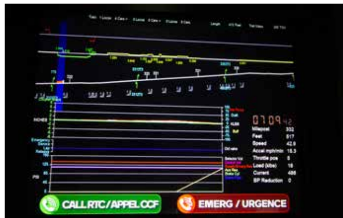
A close-up of the right screen in the image above, which helps qualifying engineers learn route characteristics. This is keyed to the video displayed through the simulator's windshields.
