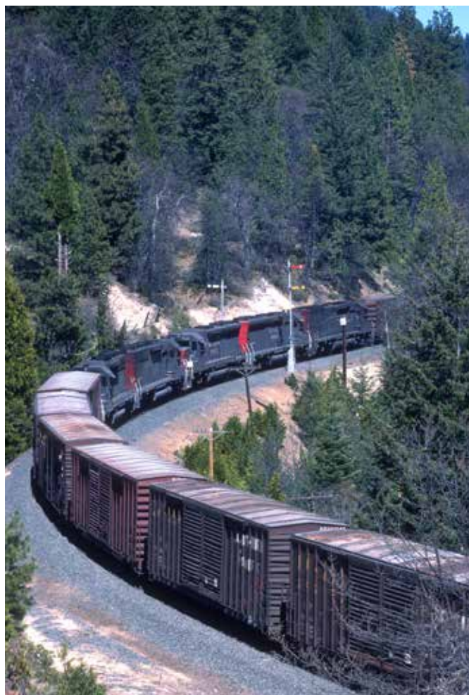
In April 1990, at milepost 409.8, the midtrain helper of SP's MERVM (Medford-Roseville manifest) was in dynamic braking to help control the train's descent of the west slope of Siskiyou Summit. Brian Solomon
