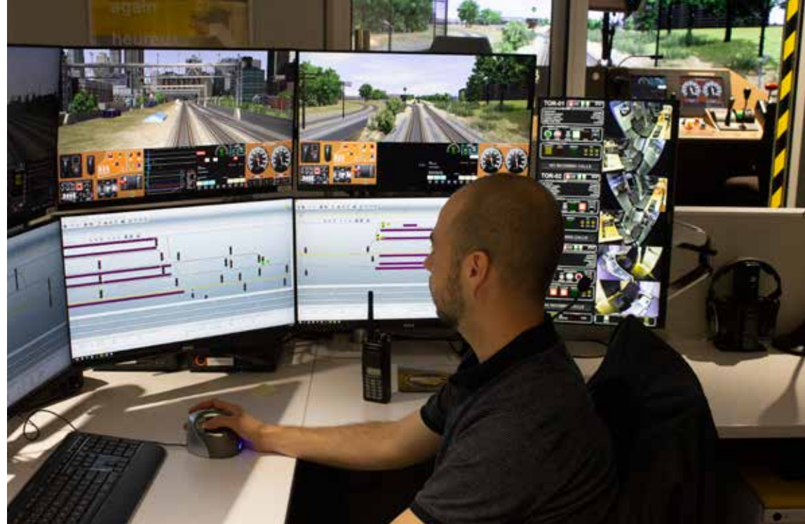
Technician Pablo Larrain at the console where variables are introduced to the locomotive simulator during trainees' operations. Behind the video screens is the hybrid simulator currently configured as an F40.
