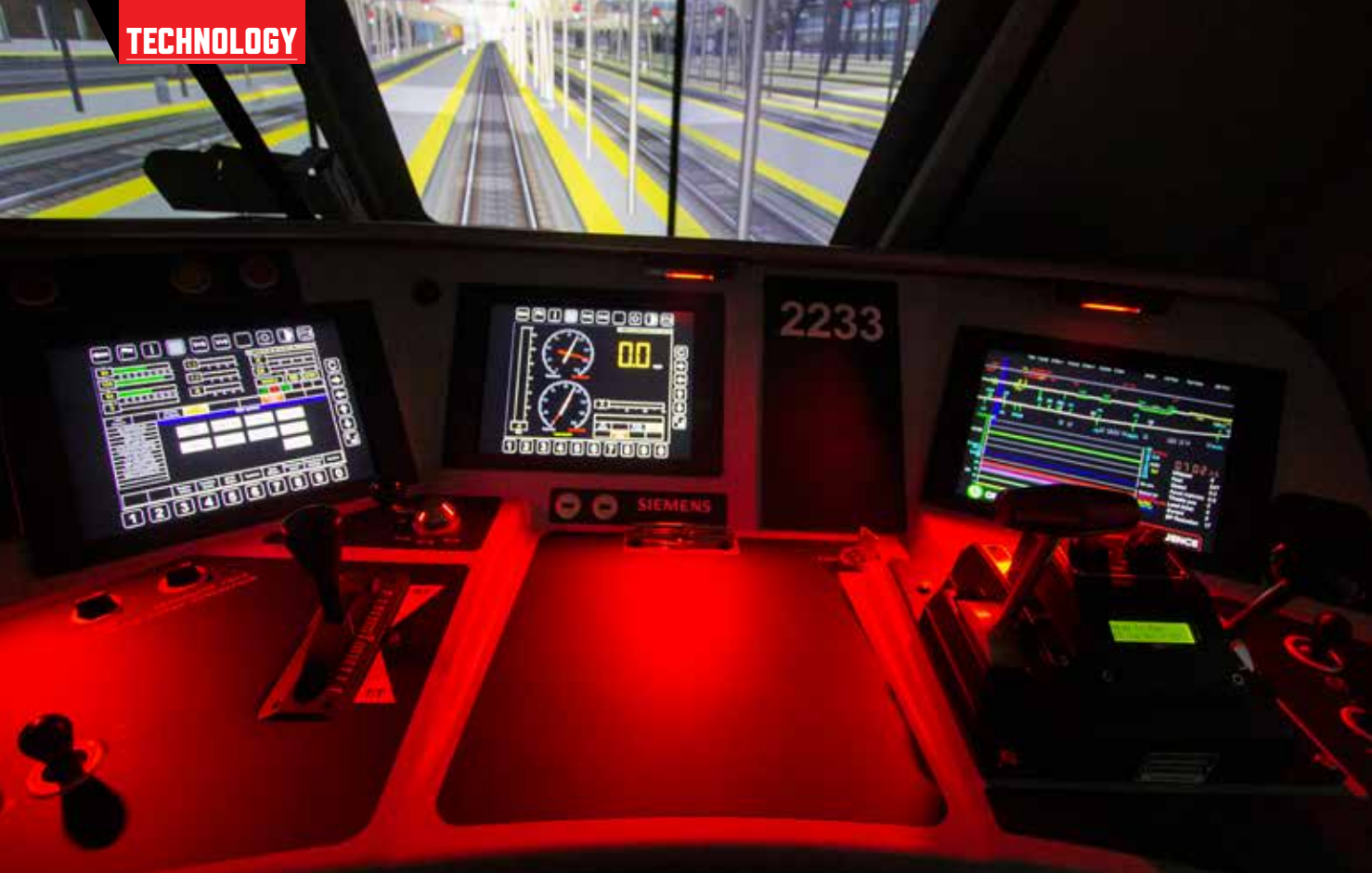
With the cab set for a night view, the simulator shows Toronto Union Station. The left screen monitors locomotive systems; the middle tracks speed, propulsion, and brakes; and the right is a simulator-only representation of grades being portrayed. Three photos, Bob Johnston
