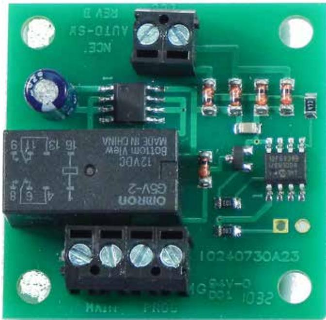
1 The NCE AutoSW combines programming and track power into a single output. Just connect an NCE PowerCab to the terminals shown at the top and you'll have main and programming outputs at the bottom. Allan Gartner photo
