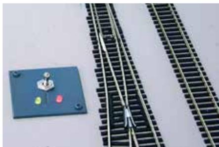
If your model railroad turnouts are controlled with switch motors, it's simple to use an LED to indicate turnout direction. Bob Kingsnorth photo
