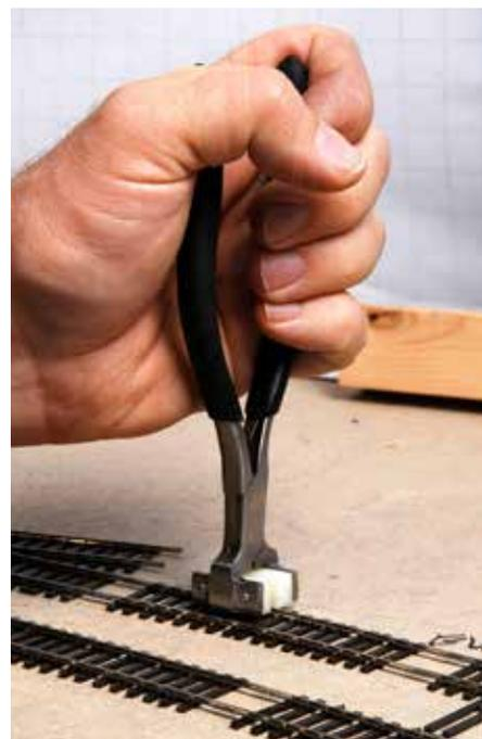
**3** The eyeglass pliers can be used to adjust track that's been laid, provided it's not yet fastened down too snugly. A gentle touch can make some fine-tuning track alignment tweaks.
