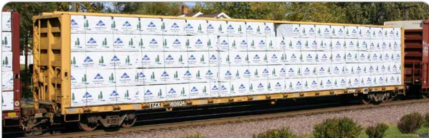
This TTXX 73-foot center-beam flatcar carries a load of wrapped sheet material in 2007. The cables and corner protectors are clearly visible against the white wrapping. This method is favored for most types of lumber today. Jeff Wilson photo
