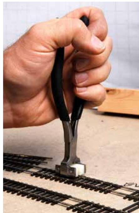
**3** The eyeglass pliers can be used to adjust track that's been laid, provided it's not yet fastened down too snugly. A gentle touch can make some fine-tuning track alignment tweaks.
