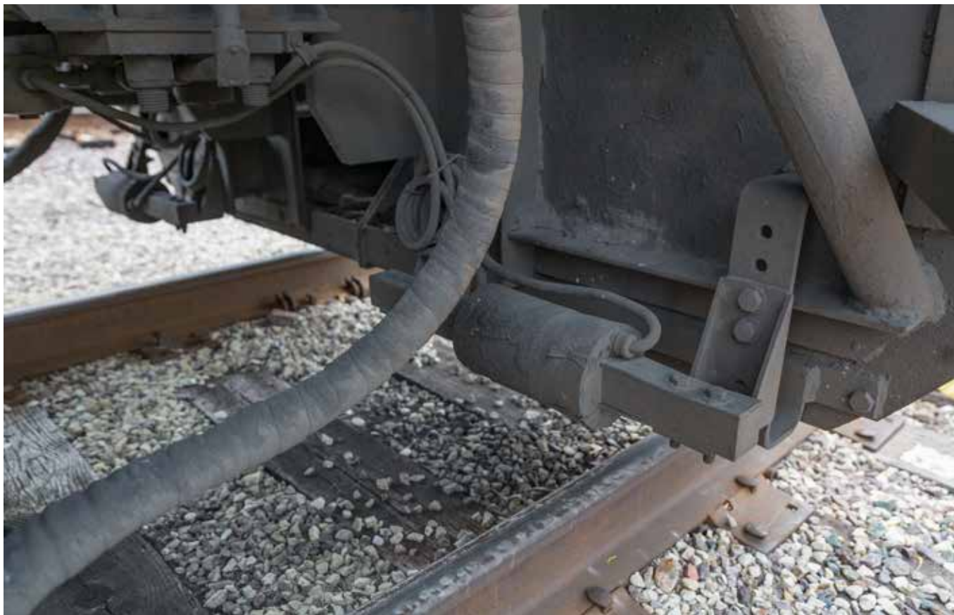
Two cylindrical cab signal antennas mounted above each rail and behind the front pilot of an EMD locomotive. The codes are transmitted through the rails and picked up by the antennas. Chris Guss
