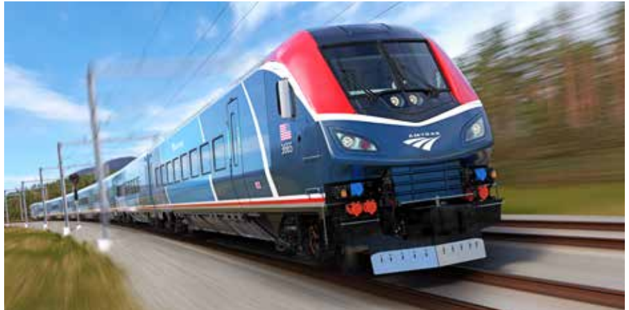
Amtrak's Airo trainsets will include two forms of dual-mode power, semi-permanently coupled equipment, cab cars for bidirectional operation, and an exterior design in keeping with the paint scheme for long-distance Charger diesels. Two images, Amtrak
