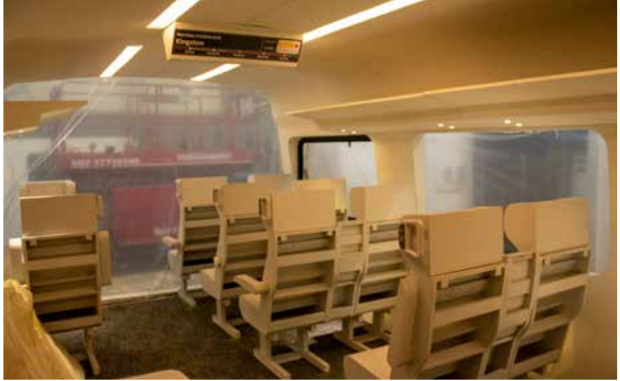
To work out accessibility details for the new equipment, VIA built this wooden mockup of a car interior at its Toronto facility, allowing for seat-spacing adjustments.
