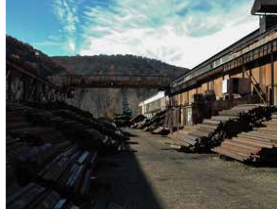
Rail is stored behind the plant — mostly in 39-foot lengths that are broken to 14-foot lengths for rolling. Four photos, Kevin N. Tomasic
