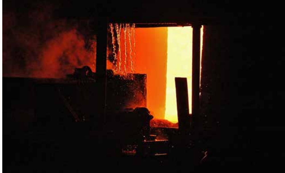
At the discharge end of the furnace, water drips onto the peel bar as it awaits the command to push another rail out of the 2200-degree furnace and into the descaler before rolling. The peel bar repeats this action every 30 seconds. Four photos, Kevin N. Tomasic
