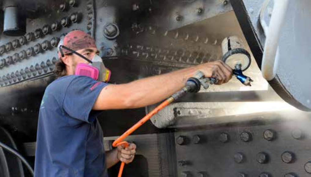
On June 15, 2017, the restoration of No. 3132 is nearing completion. The painting contractor sprays a finishing coat of shiny black DuPont Imron paint beneath the cab and behind the firebox. When done, No. 2132 looked like it was fresh from the South Louisville Shops. Ron Flanary
