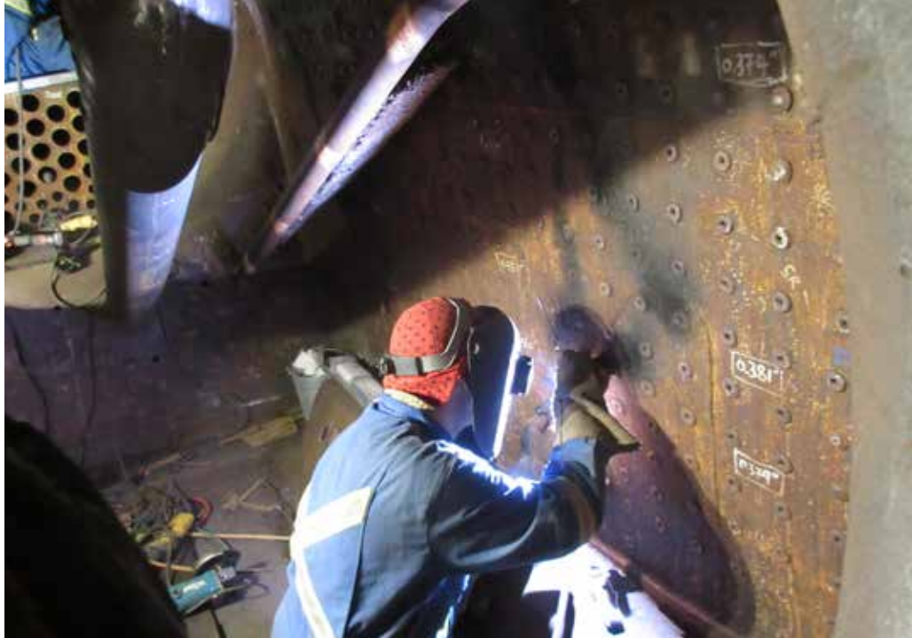
An employee from D.F. Boiler Tube Industries works in the firebox of No. 6060, welding a plug in a test hole. D.F. Boiler is also working on staybolt replacements for the locomotive. Don Totten
