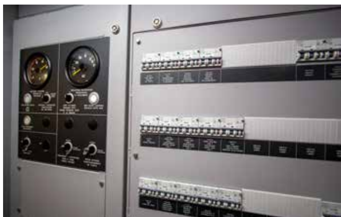
A closer look at the locomotive control panel in the cab car. The basic design for the Canadian equipment will also be used for Siemens trainsets in the United States.
