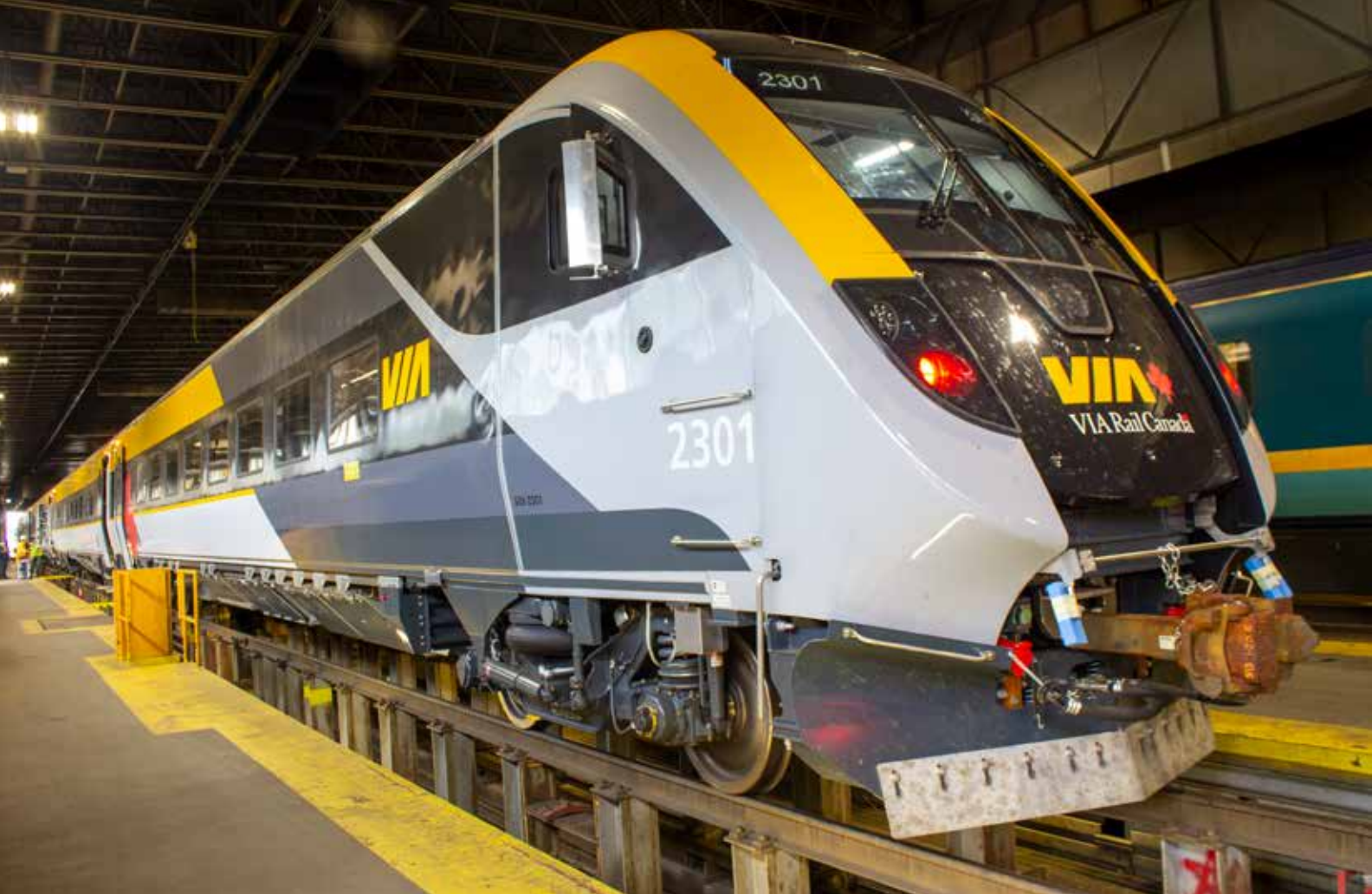
A cab car for one of the VIA Venture trainsets is inspected during testing at the Montreal Maintenance Centre. The first cab cars built for Venture equipment, they will be followed by structurally similar U.S. versions for San Joaquin Venture and Amtrak's Airo trainsets.
