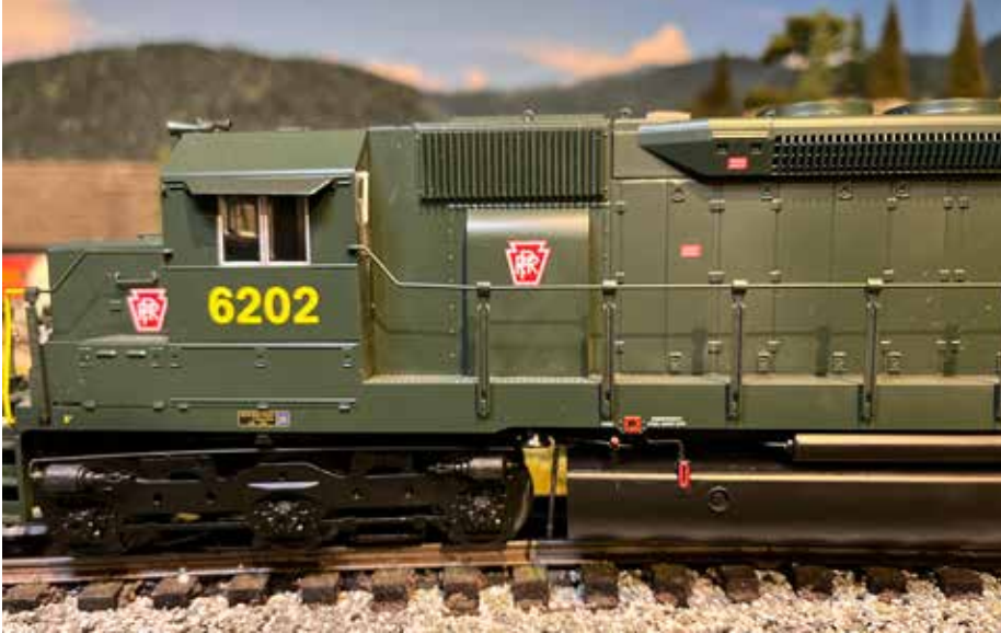
The O gauge model of this high-horsepower 1960s road diesel is loaded with detail. Note the brake piping on the trucks, the bell under the frame, and builder's plate under the cab.
