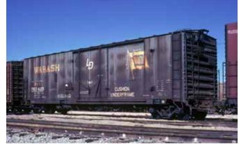
The 40-foot boxcar grew to 50-feet long in the early 1930s. Car doors became larger affording more convenient loading and unloading. The added length increased capacity to 70 tons. L.E. Raby, Tom Kline collection
