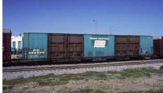
Measuring 86 feet long, Penn Central No. 293936 represents the larger boxcars introduced in the early 1960s. With nearly 10,000 cubic feet of space, these rolling barns are ideal for auto parts.
