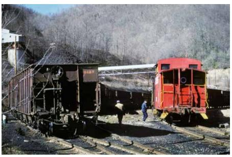
The Interstate Railroad's fourth mine run has arrived at the Roda, Va., load-out on April 12, 1985, with a string of empty hoppers. A swap will ensue between a like number of loaded "yellow ball" 50-and 70-ton hoppers in captive service between mines and transloader.
