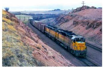
First, EMD built the cabless DD35, second in this consist. Union Pacific asked for an cabbed version, as well. Here DD35A No. 84 leads its train up Wyoming's Sherman Hill on May 12, 1968. Steve Patterson
