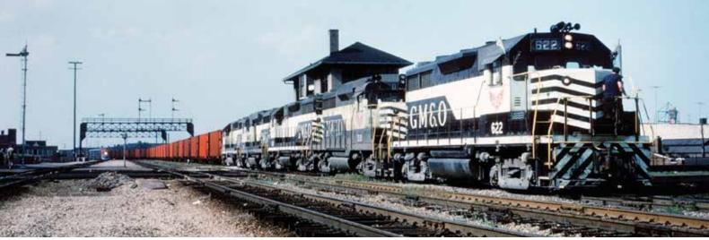
Flying the flags of an extra, new GM&O GP30s and GP35s ease across the Rock Island diamonds at Joliet Union Station in August 1966, handling one of the Gee-Mo's two new coal trains. This is an empty State Line train, the rear end of which is just coming off the Elgin, Joliet & Eastern, which handled the trains between State Line Generating Plant at Hammond, Ind., and Joliet.
