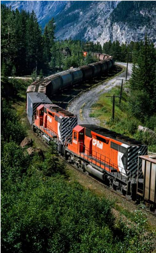
Well before the advent of distributed power, two remote control "slave" locomotives assist a freight train snaking through Yoho, B.C., on Aug. 18, 1974.
