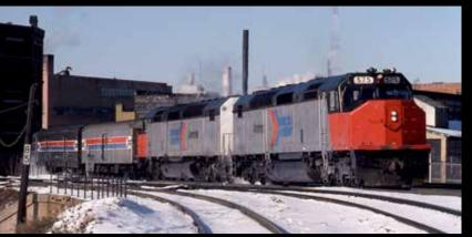
**At the head end** are SDP40F diesels Nos. 575 and 563, built by EMD in May 1974. No. 575 sports the later body style with a flat nose. The train is snaking through the Florida Street S-curves south of the Milwaukee station.
