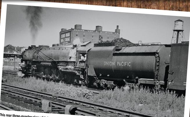
This rear three-quarter view of Union Pacific 4-12-2 No. 9048 shows a tender piled high with coal. The locomotive is one of 25 in the UP-4 class built at Schenectady in 1929 and retired 1953-1956.
