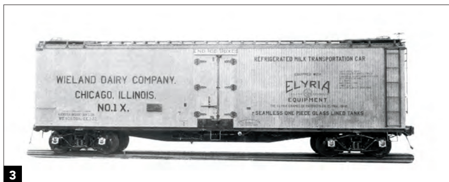
The first production milk tank cars were three General American cars with Elyria glass-lined tanks. Each had twin 3,000-gallon tanks and ice bunkers. They were not equipped for passenger service. General American
