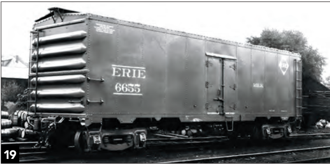
19 Erie's 40-foot milk cars of 1935 and 1937 were the first all-steel milk can cars. They had Buckeye ends, Viking roofs, and trucks from older retired milk cars. Greenville Steel Car
