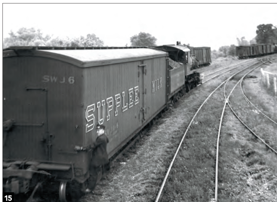
15 Supplee No. 6, a late MDT car built in 1930, has the distinctive separate letters that make the brand's cars stand out. MDT cars lacked the trim boards of the General American wood cars. It's being switched on the Huntington & Broad Top. Al Rung
