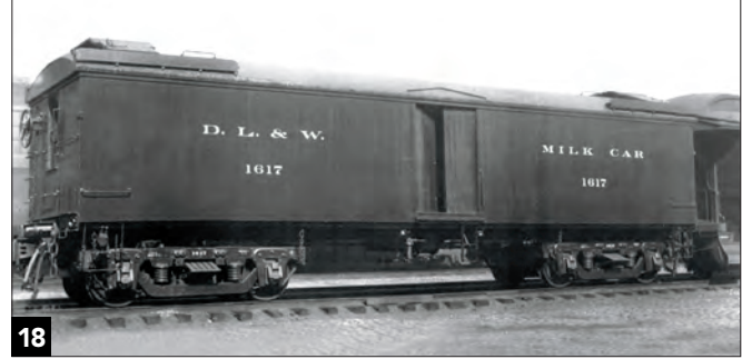
18 The inward-swinging doors are easy to see on Lackawanna 45-footer No. 1617. Cars in this series originally had ice bunkers like this one; many were later rebuilt and had them removed. Bob's Photo
