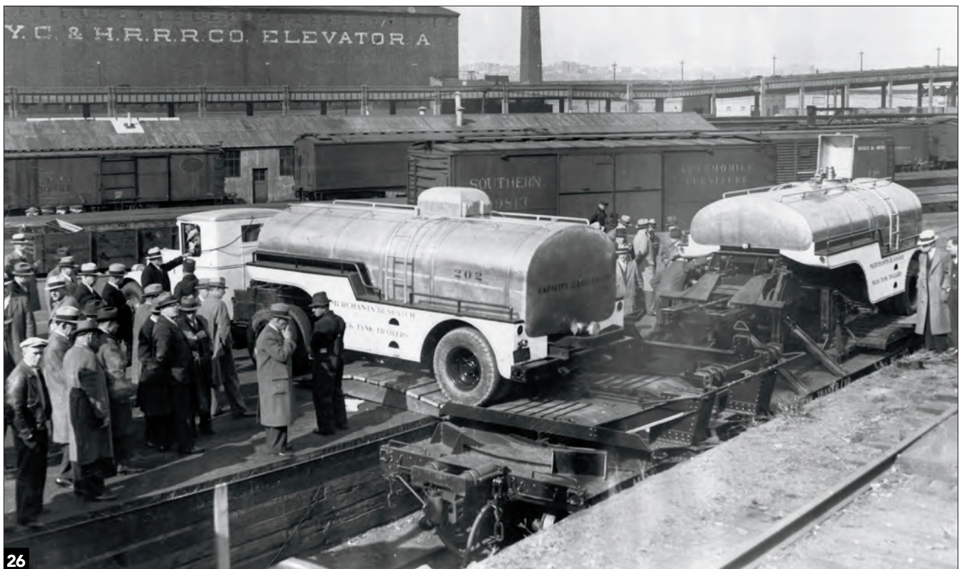
Trailers were backed perpendicular to the car, then rotated on a platform on the car and locked into place. This was a demonstration of the system in New York City on October 30, 1934. Merchants Despatch
