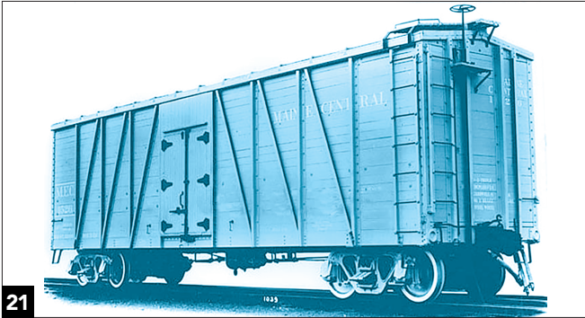
21 Maine Central's milk cars were classified as insulated boxcars, and were unusual in being single-sheathed with swinging doors. Number 1526 is a 40-foot, 40-ton car. Standard Steel Car
