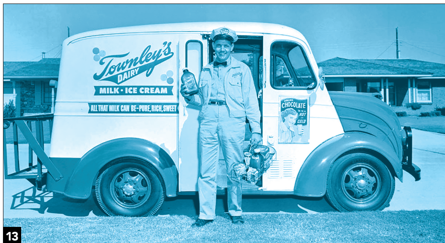
Divco trucks were popular for home-delivery companies, especially dairies. This basic body style with distinctive rounded nose was built starting in 1937; this truck is shown in 1953. Jeff Wilson collection
