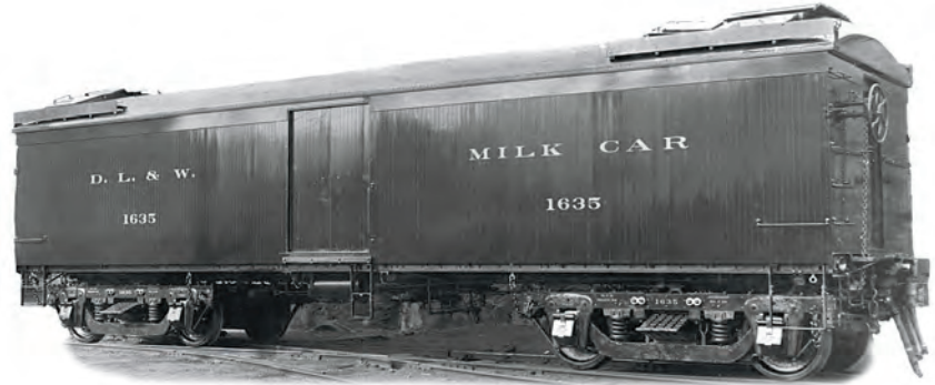
15 Delaware, Lackawanna & Western No. 1635 is a 45-foot wood car for carrying milk in cans. It has high-speed trucks, passenger steam and signal lines, and inward-swinging doors. John Nehrich collection
