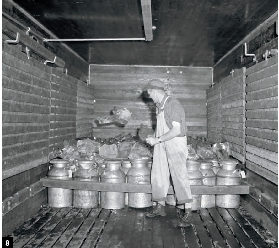
Cans in this car are secured by wood planks placed in notches on the sides. Note the fold-down racks for a second layer of cans. Ice was chopped and shoveled directly on cans in warm weather. Jack Delano, Library of Congress
