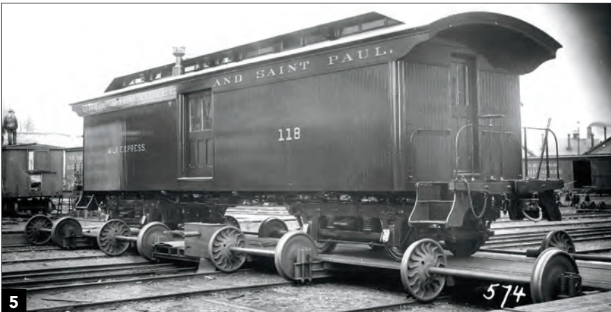
5 Early milk cars often resembled baggage cars, as shown by Milwaukee Road 118 circa 1890. The car has a sliding door, clerestory roof, end platforms, and link-and-pin couplers. Milwaukee Road
