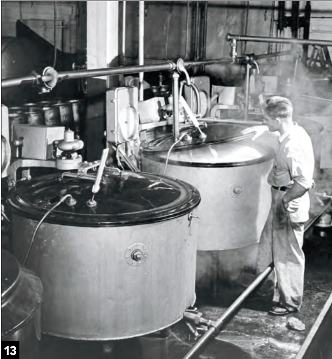
13 Milk is pasteurized before bottling. The creamery at Sheldon Springs, Vt., had multiple pasteurization tanks (each with a temperature recorder above it) in this 1941 view. John Vachon, Library of Congress
