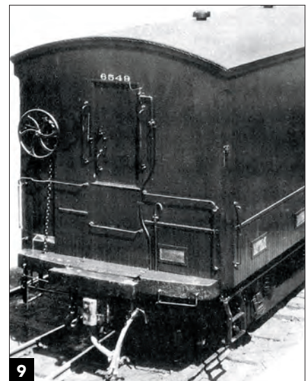
Cars equipped for head-end service have a steam line (curved pipe under coupler), air and signal lines (right of coupler), and buffer (above coupler). This is a New York Central 50-foot milk car. New York Central
