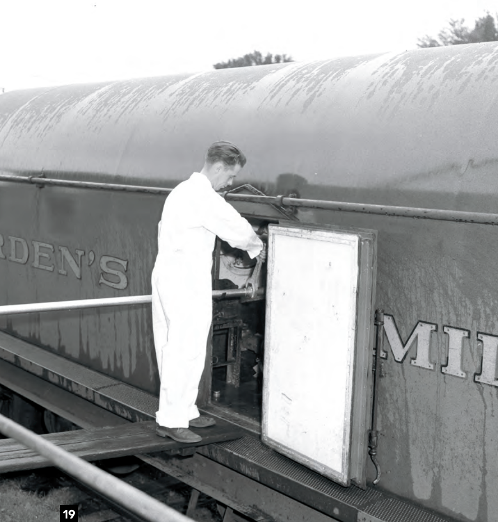
A worker tightens a connection to ready a Borden car for loading at a collection creamery in 1947. Note the heavy insulation on the door, and that the car still has the separate metal letters applied to the hood. Precise spotting of the car is required for alignment of the loading pipe. Both photos: New York Central
