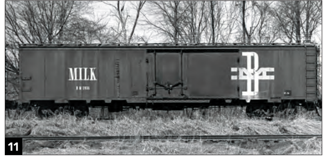
11 Among the last can cars built were 35 all-steel cars for Boston & Maine. Number 1934 is one of 20 single-plug-door, 50-foot insulated cars delivered in 1957. Scott A. Hartley
