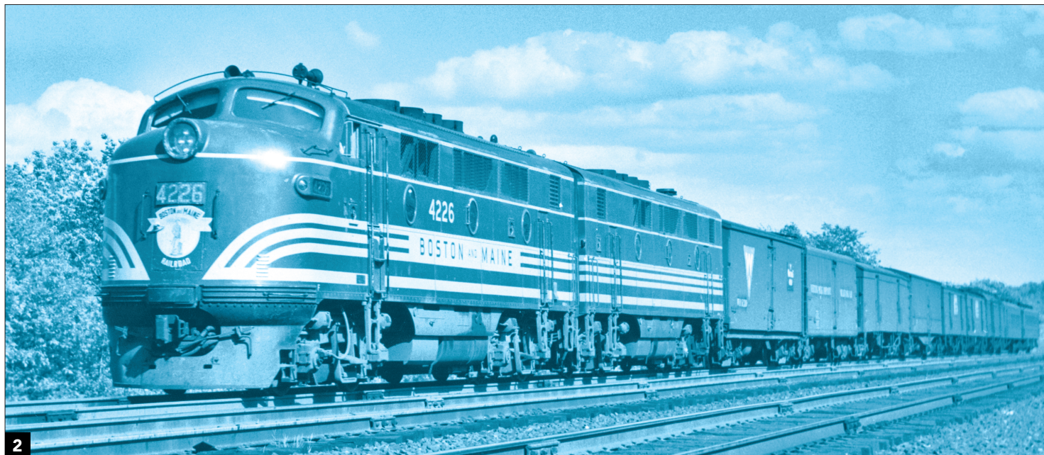
Diesels headed many milk trains from the 1940s onward. An A-B set of EMD F3s leads Boston & Maine train 5507, bringing empty milk cars northward near Fitchburg, Mass., in 1952. George C. Corey
