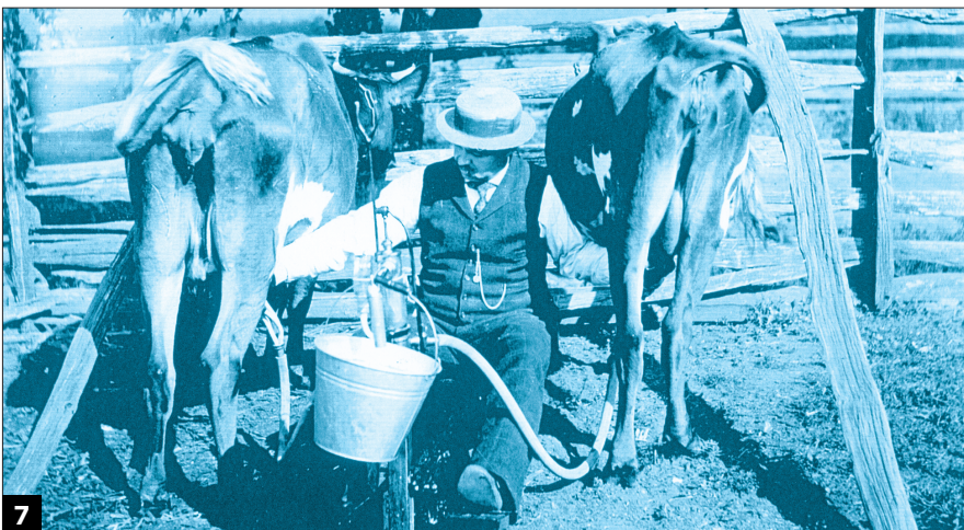
The Mehring milking machine, powered by foot pedals, was among the earliest successful milking devices. It allowed milking two cows at once. More than 3,000 were made from 1892 to 1920. U.S. Department of Agriculture
