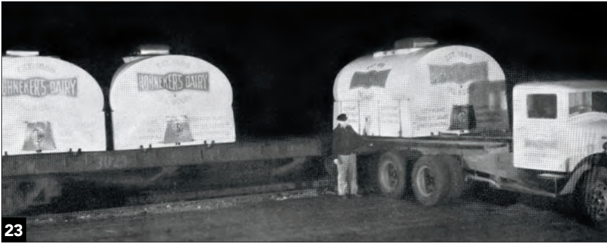
The first milk containers were 8 feet long and mounted transversely on flatcars. These Hohneker's Dairy containers are being unloaded from New York, Ontario & Western flatcar No. 3029. Motor Terminals Inc.
