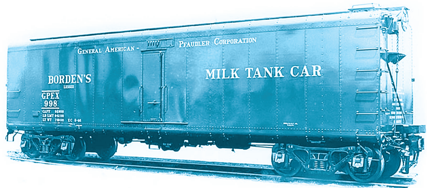
16 This 40-foot steel car, built by General American-Pfaudler in the mid-1940s and leased to Borden, represents the final development in milk tank cars. It has two 3,000-gallon glass-lined tanks. General American
