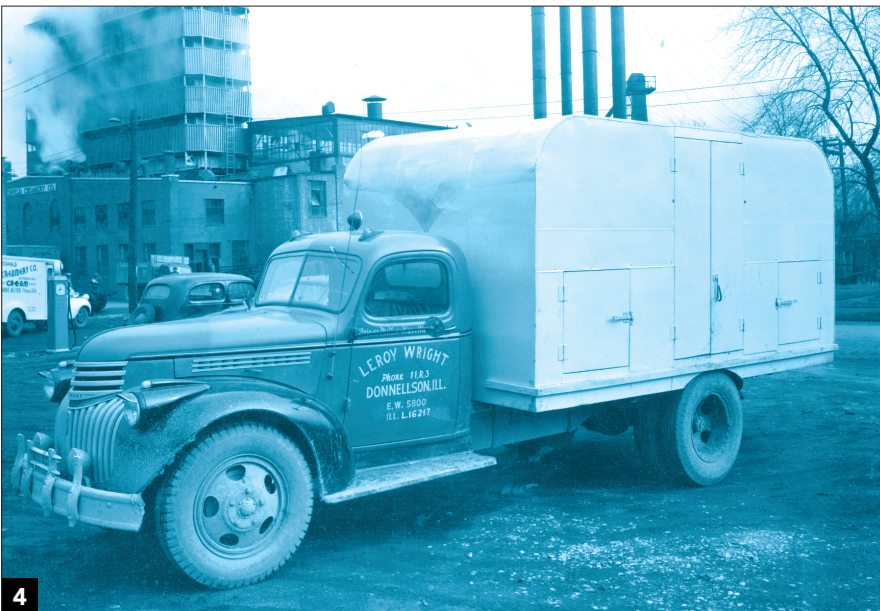
4 Body styles varied, but the most-common can truck from the 1930s through the 1960s was an enclosed body with doors on each side and rear. The rounded front and rear roofs were common. Jeff Wilson collection
