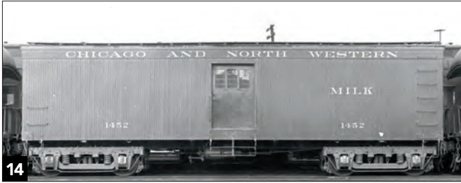
14 The North Western's 1911-built milk cars were 40 feet long with steel underframes and rode on passenger-style (7-foot wheelbase) trucks. The wood bodies had a centered sliding door. Keith Kohlmann collection
