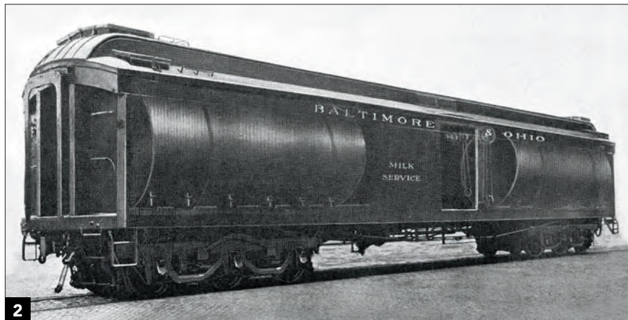
This rendering shows how two Pfaudler tanks were placed inside a Baltimore & Ohio six-axle baggage-cars-turned-express-reefers in 1921. Baltimore & Ohio
