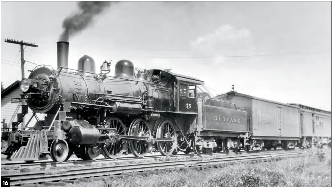
One of Borden's wood-body MDT-built tank cars is tucked behind Rutland 4-6-0 No. 45. Borden began rebuilding these cars into streamlined ("butter dish") cars beginning in 1936. Trains magazine collection
