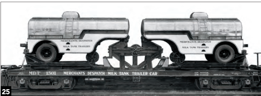
In 1934, MDT demonstrated a pair of 2,100-gallon tank trailers on a customized piggyback flatcar equipped for passenger service. Merchants Despatch
