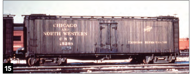
15 The majority of the C&NW's milk cars looked like standard wood reefers riding on high-speed trucks. Some, like 15298, had bunkers. It's shown in 1955 in express reefer service. Keith Kohlmann collection
