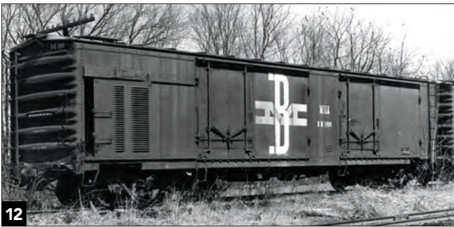
12 Number 1909 is one of 15 mechanically refrigerated milk cars purchased by Boston & Maine in 1958. The 50-foot double-door car was designed to carry refrigerated cases of milk bottles. Scott A. Hartley
