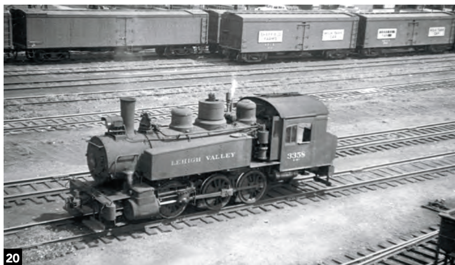
Lehigh Valley had a saddle-tank 0-6-0 switcher at Sayre, Pa., in the 1930s. In the background at left are LV's distinctive wood, archbar-truck milk cars, plus (at right) two first-generation General American milk cars (both owned by Sheffield Farms, SFCX). Frank Snyder
