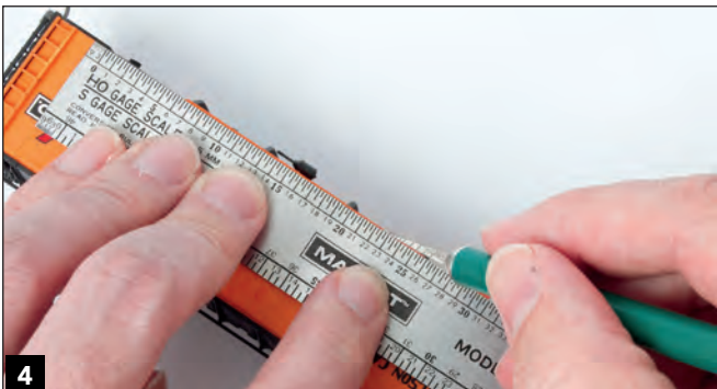
Use a straightedge to guide the knife blade when cutting off the drop-down tab along each side.
