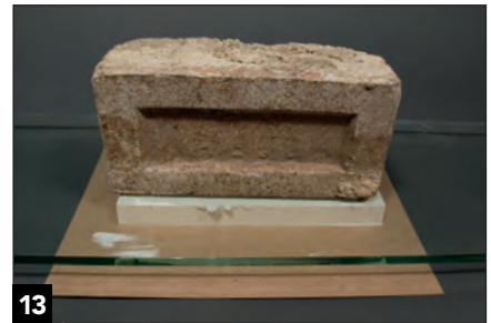
13 I set a piece of plate glass on top of the mold to ensure mating faces of the castings would be flat. If you skip this step, you'll have a lot of sanding to do.
