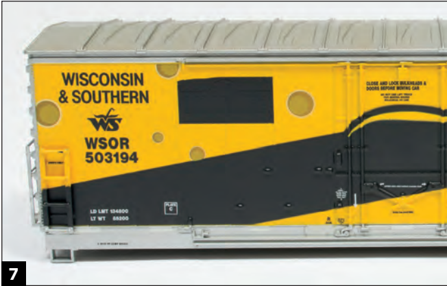
7 Apply a patch over the Plymouth logo. The wavy edge at its upper left is unique to the right side of the car.
