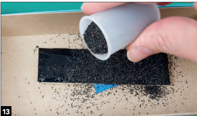
13 While the paint is wet, sprinkle scale coal over the load and press it in place.
