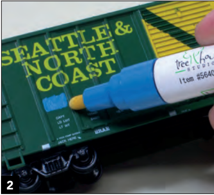
2 When freight cars change ownership, the reporting marks need to be changed to reflect the new owner. The factory-painted reporting marks on this SNCT boxcar is covered with a simple swab of paint.
