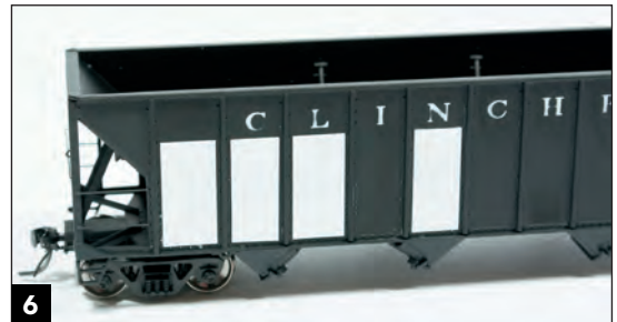
6 I thoroughly washed the model to remove residue from the wet-sanding process. Then I used .010" styrene cut to fit to simulate the repaired body panels. I used medium viscosity CA to attach the styrene to the plastic.
