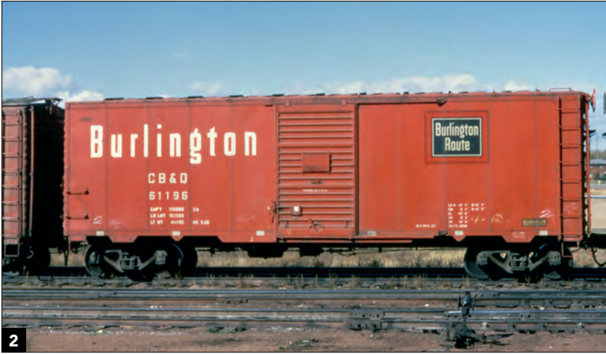
2 This Chicago, Burlington & Quincy boxcar, built in 1953 and photographed in 1967, had been rebuilt just a year earlier. It received a new paint scheme and had its running board removed. Hol Wagner
