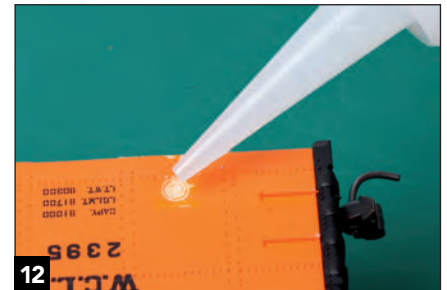
12 CA works well as a body filler. Add a drop of accelerator after applying the CA.
