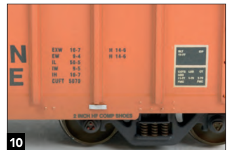
10 Although not a part of the car when first built, the Automatic Identification Tag indicates that this car operates in the modern era. The detail part is offered by A-Line as item no. 29460.
