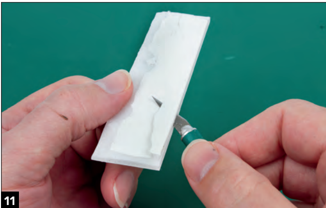
11 Cut a foam piece to fit the car and then carve it so it is raised in the middle to duplicate the center heaping of a prototype coal load.
