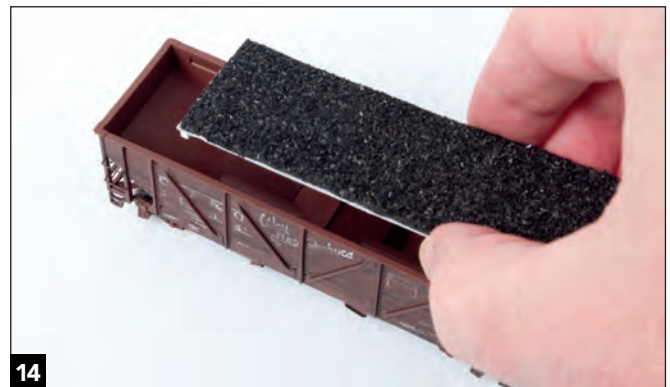
14 Set the load in the car, and glue styrene spacers under each end of the load to raise it to the desired height.
