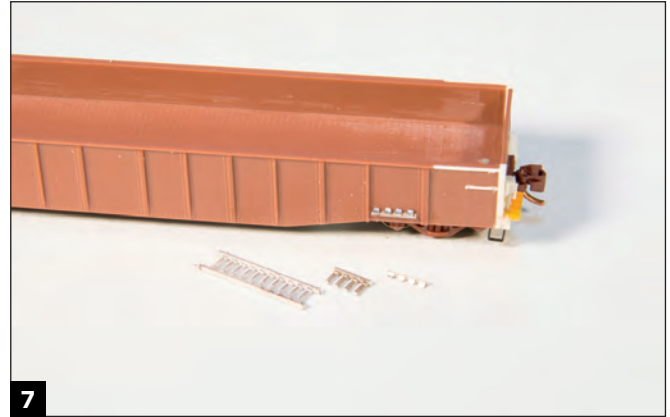
Next, I glued a strip of styrene along the top of the car at the corner. I made the flanged brackets from porch railing.
