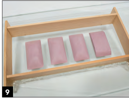
9 A piece of plate glass and wood paint sticks make an easy mold box. I sealed the seams in the box and the edges where the sticks meet the glass with hot glue.
