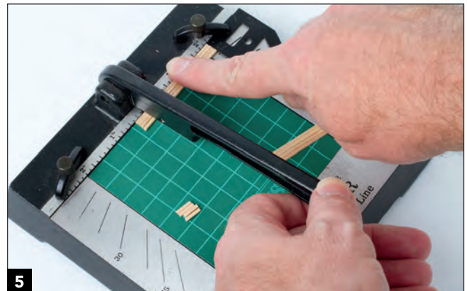
5 Cut the strips to length. A NorthWest Short Line Chopper is a handy tool for this.
