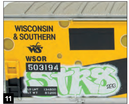
11 Brush on Micro Sol so the film conforms to the irregular surfaces and let the decals rest. Then add the road number, load limit and light weight data, and COTS panel.
