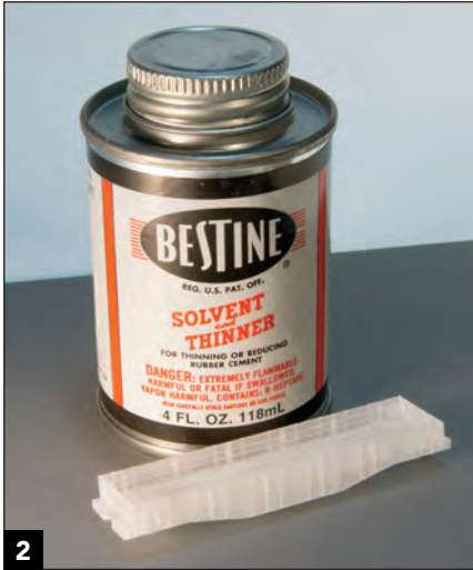
2 Soak the Shapeways 3D printed model in Bestine or Simple Green to melt off the support wax residue.
