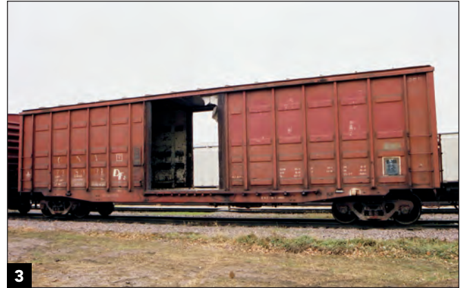
Cars in this service used temporary paper doors to contain the chip load. (You can see a scrap at the top of the opening.) This car has had its steel doors removed.
