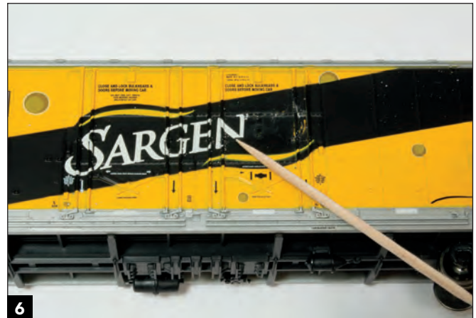
The Micro Sol and tape technique didn't work so well on the SARGENTO lettering. Apply Micro Sol over the lettering and gently scrape it with a round-head toothpick. Even if you're careful, some black paint under the lettering might be damaged.
