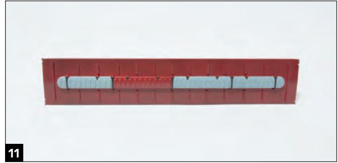
11 To better match the prototype, I brush-painted three of the four hatch covers with Polly Scale new gravel gray. I made the batten bars and hinges stand out by painting them grimy black.
