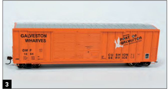
This is how the Athearn Ready-to-Roll car looked straight out of the box. I replaced the plastic couplers with metal knuckle couplers from Kadee.
