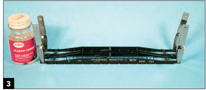
3 Fill the slots behind the side sills in each corner with black .030" styrene. Heat sink clamps hold the styrene in place for gluing. This allows for easier installation of the A-Line metal steps.
