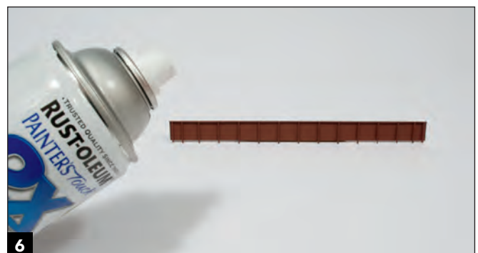
After assembling the sides, I spray-painted them with Rust-Oleum Painter's Touch 2X flat red primer. This plastic-compatible paint provides a great base for simulating rusty metal.
