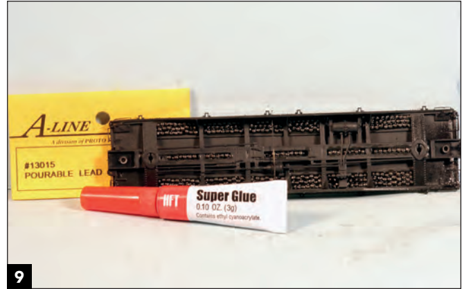
9 Super-gluing lead shot to the underside of the flatcar brings its weight up to 4 ounces, the NMRA standard.
