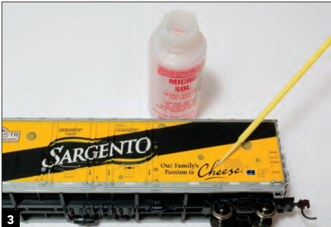
Apply Microscale Micro Sol setting solution to the OUR FAMILY'S PASSION IS CHEESE slogan (but not the underline). Let the setting solution sit until it has almost completely evaporated.
