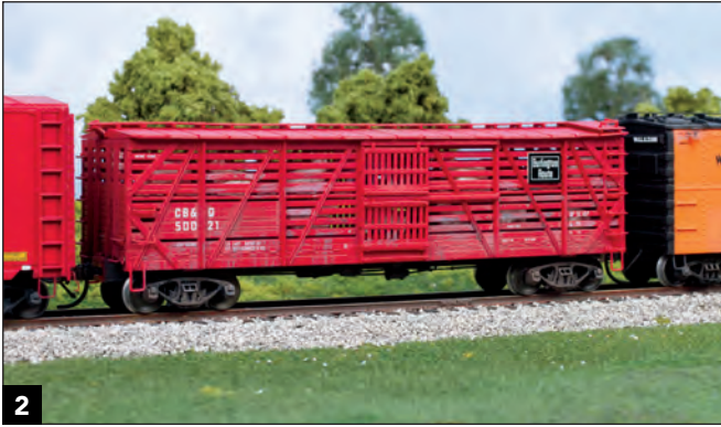
2 This double-deck Proto 2000 Mather stock car received a load of sheep as well as light overall weathering.
