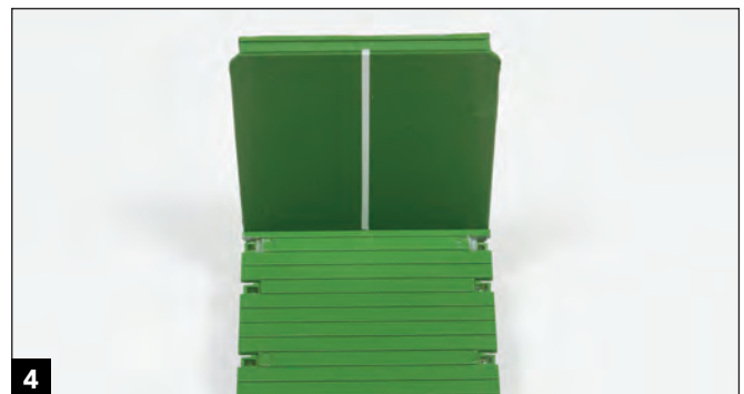
The model needed two extra stake pockets per side. I cut notches in the first full board closest to the bulkhead for the new pockets. I used pockets from a car I damaged in my first attempt at modeling the 621549.
