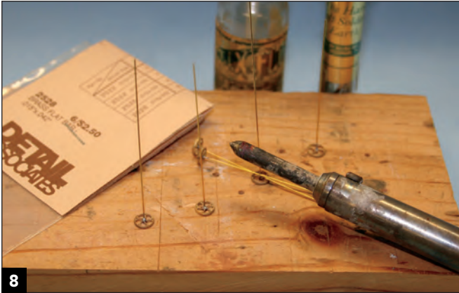
8 Place the brass brake wheel on a wood base, hold the .015" brass staff in place, hold the soldering iron at the joint, and touch the rosin-core solder to the joint until it flows.
