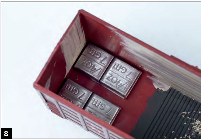
8 A-Line's peel-and-stick lead weights work well, as they can be hidden out of view in each end of the car.
