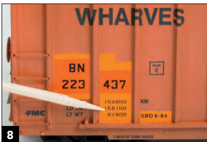
8 After applying decal-setting solution to the trim film and letting it dry, I added the new capacity data from a decal set designed for FMC boxcars. The reweigh date indicates this car spent time on the Seaboard System before coming to the BN.
