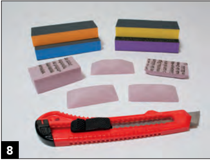
8 I made patterns for the gravel loads using \frac{3}{4} " extruded-foam insulation board.
