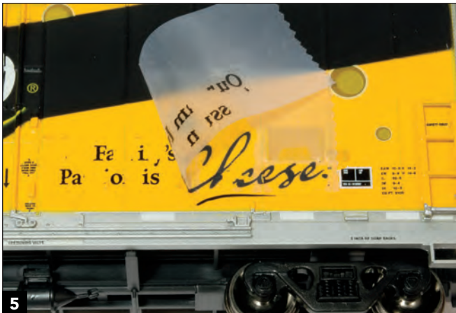
Peel the tape up and away from the model. If not all of the lettering comes off during the first attempt, just repeat the steps until all of the lettering has been removed.
