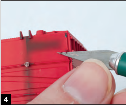
4 Trim off the running board supports at the corners and ends. The mounting hole at the left has been plugged with a scrap piece of sprue glued in place.
