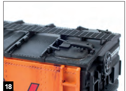
18 The new running board has a slim profile that's much more realistic than the original injection-molded item.
