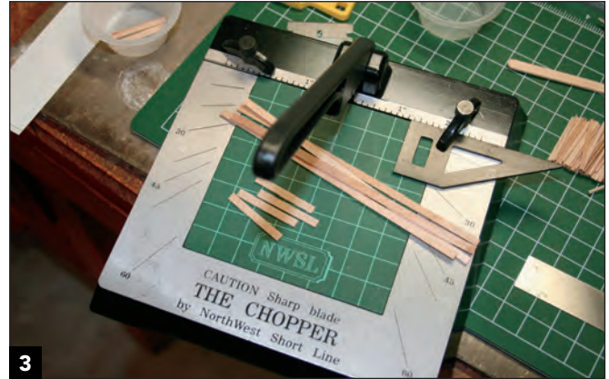
3 Cut the wooden stir sticks into sections the same width as the subfloor. The NorthWest Short Line Chopper makes short work of accurately cutting the stir sticks.
