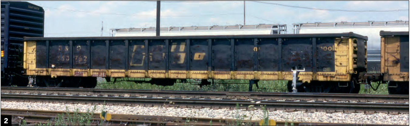
This Railgon car had been in service 13 years in this 1992 photo, but it looks older with its missing and worn lettering, new reporting marks and capacity data, and lots of rust and general wear and tear.
