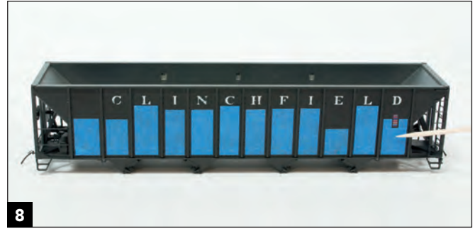
8 Once the engine black paint had dried, I masked those areas with blue painter's tape. Though no longer used, shop forces masked around the Automatic Car Identification panel on the right side of the car.
