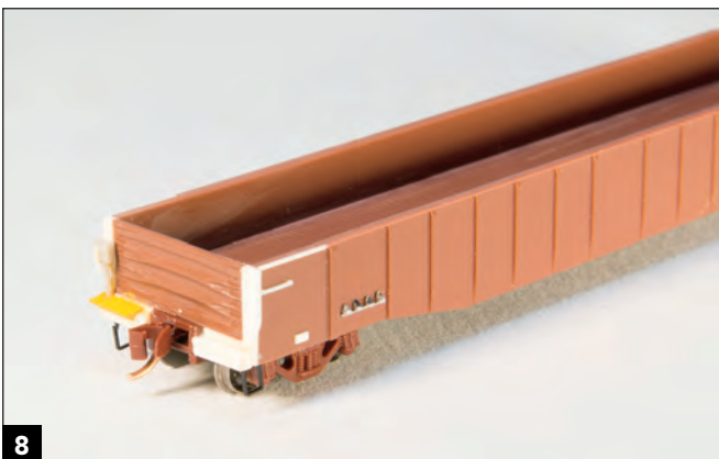
I built up the ends of the car with styrene and glued a handbrake and a step to the corner of the B end.
