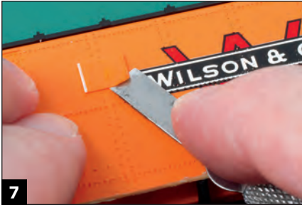
7 Cut away the molded tack board with a chisel-tip hobby knife blade. Work slowly and make multiple passes.
