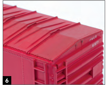
6 A couple of coats of paint help hide the roof plugs and any exposed black plastic from under the old running board.
