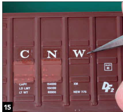
15 Add the new reporting mark and number decals to each side.
