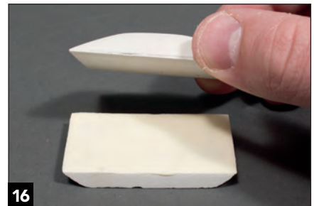
16 I used wood glue to attach the top half of the casting to the bottom. Wipe any glue that oozes out with a damp paper towel.
