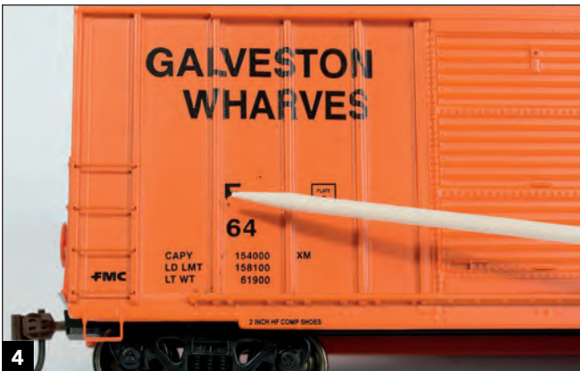
After soaking the reporting marks and road number with Microscale Micro Sol and letting the decal-setting solution evaporate, I used a round-head toothpick to gently scrape off the factory lettering. I also used this technique to remove the car capacity data, built date, and end reporting marks.
