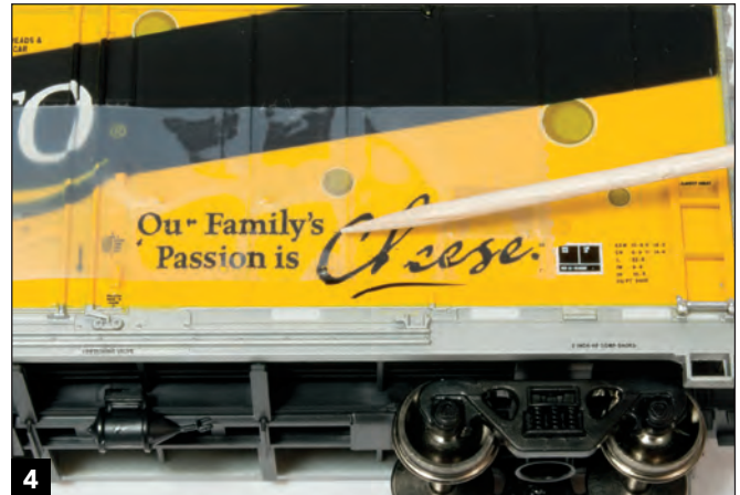
Apply Scotch Magic tape to the slogan area. Burnish it with a toothpick.
