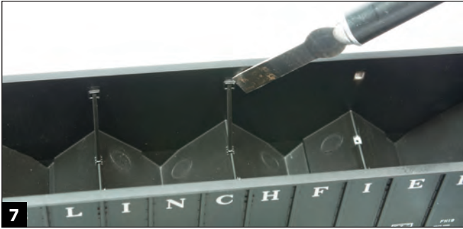
7 To make it easier to reach the ejector-pin marks on the slope sheets, I removed the six interior braces. A gentle rocking motion with a no. 17 blade was all it took to break the glue joint.
