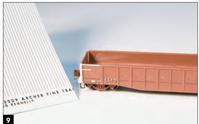
I placed a row of Archer resin rivets at the floor line of the car.
