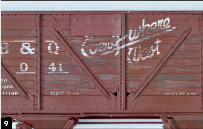
9 Paint the patch boxcar red, test-fit it, and then use super glue to secure it at the top of a side panel.
