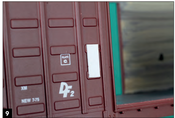
9 A small piece of .010" styrene, cut to fit over two of the side protrusions, will hold the ACI plate decal.
