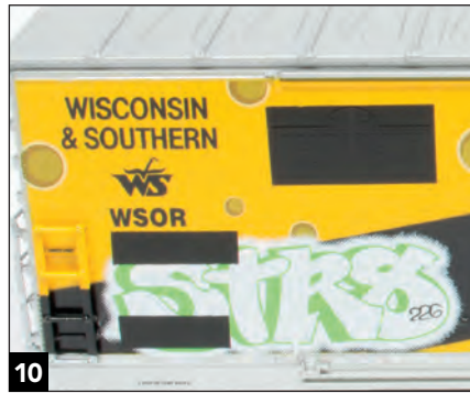
10 After applying Micro Sol to the graffiti and letting the decals rest, add the black trim film patches for the road number ( \frac{9}{16} " x \frac{5}{32} " ), capacity data ( \frac{33}{64} " x \frac{5}{32} " ), and COTS panel ( \frac{21}{64} " x \frac{7}{32} " ).
