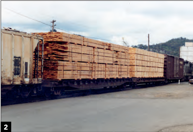
2 By the 1960s, bundled lumber was becoming more common on flatcar loads, replacing the hand-stacked loads common before that period.
