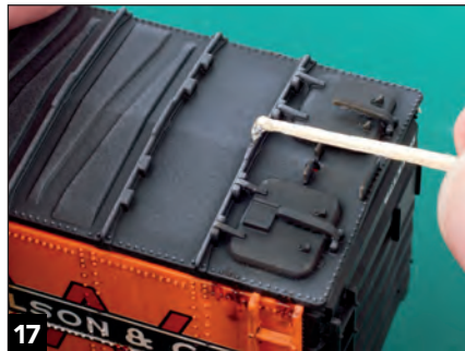
17 Use a toothpick to apply E-6000 adhesive to each running board support and then set the running board in place.
