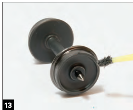
13 Replace the stock wheels with InterMountain 33" metal wheelsets. After cleaning them, paint them with Model Master railroad tie brown, keeping the color off the treads and needlepoint axles.
