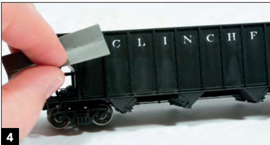
4 Using 600- and 1,500-grit sandpaper, I wet-sanded the car to remove all of the factory lettering except for the CLINCHFIELD lettering, ACI labels, and data on the slope sheets. I used the same technique to weather the CLINCHFIELD lettering.
