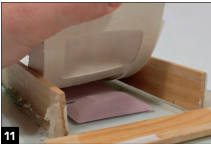
11 After letting the silicone rubber cure for 18 hours, I carefully removed one wall from the mold box and then gently lifted the mold from the box.
