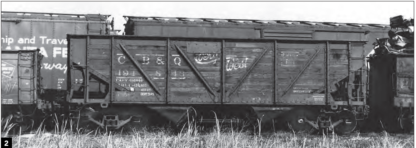
This composite-side war-emergency hopper, built in 1944, shows its age in this mid-1960s photo. The boards show lots of texture, with a significant patch at the top of one side panel. William Raia
