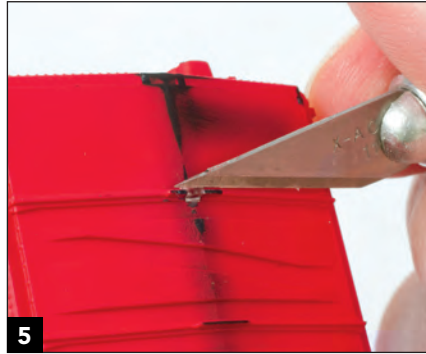
5 Trim the plug to match the existing roof texture. Start with a hobby knife and then use needle files to finish.
