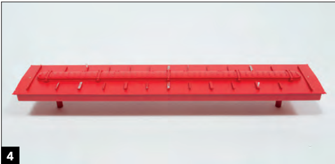
4 I removed the plastic running boards using a screwdriver. Some mounting pins snapped off during the process, which was okay. I filled the remaining holes with .035" styrene rod. I secured the pins and rod with glue and sanded the bracket tops smooth.
