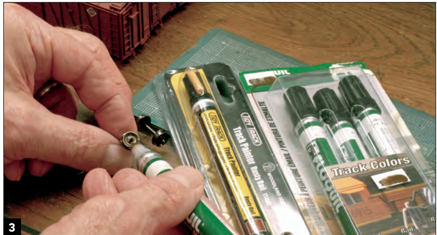
Weathering metal wheels is as easy as wiping around the outer surface with the tip of a rail brown or grimy black weathering pen while holding the wheelset in your hand.
