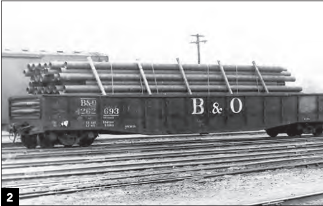
2 The pipe load in this Baltimore & Ohio mill gondola is stacked, held together with bands, and kept in place in the car by vertical posts. Trains magazine collection
