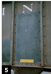
5 This close-up is of a prototype reinforced body panel. William Phalen, Cody Grivno collection
