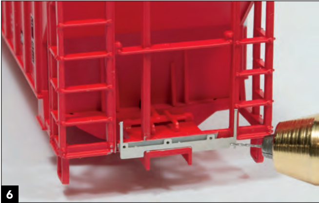
6 I centered the jig for the crossover platform on the draft-gear box and used a pin vise with a no. 78 bit to make holes for the new part. I repeated this process on the B end of the car.
