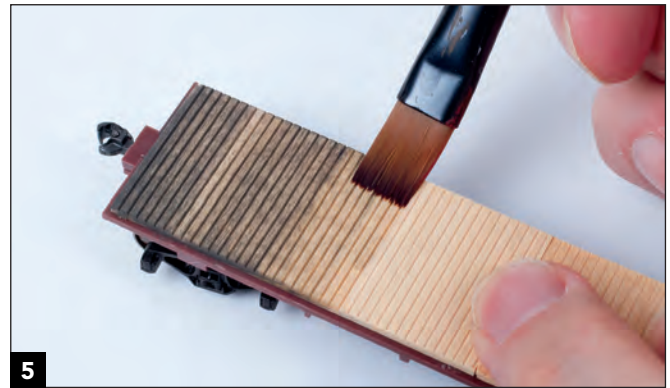
5 The new floor is Northeastern scribed basswood, glued in place with super glue and weathered with a grimy black wash.
