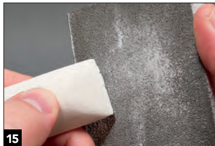
15 Sanding sponges make it easy to clean up rough edges on the castings. Check your work often, as it's easier to remove more material than try to add more.
