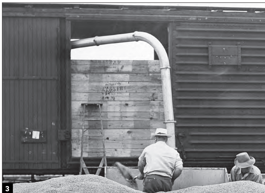
3 Workers load a boxcar with a conveyor in the 1940s. The wood grain doors are stenciled RETURN TO AT&SF. Jeff Wilson collection
