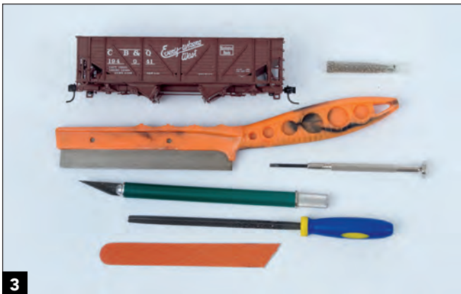
A variety of tools can be used to distress car sides, including a wire brush, razor saw, screwdriver, hobby knife, file, and emery stick.
