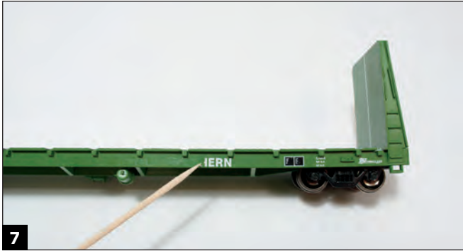
7 I applied Micro Sol over the factory printing. Once the decal-setting solution evaporated, I gently scraped away the lettering with a round-head toothpick.
