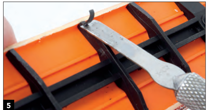
Carefully shave the crossbearers so that the bottom of each end is even with the bottom of the car side.
