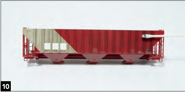
10 A cotton swab dipped in Windex is handy when doing some reverse weathering. Here, I am wiping paint off the faces of the exterior posts. I also used this technique to remove some of the weathering from the body panels (with the masking tape on, of course).
