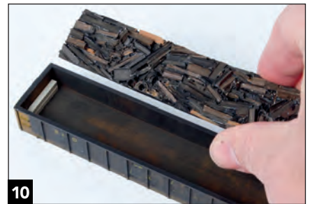
10 Cut the load to fit. Styrene spacers elevate the load to the proper height. Glue the spacers to the load, not the car.
