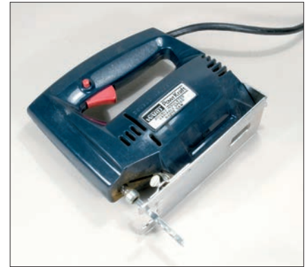
Jig saw. This is a power saw where the blade protrudes downward. This saw is similar to a scroll saw, but it's not as accurate, mainly because you have to move the saw rather than the work piece. It is also more difficult to see the work surface as you are cutting. The jig saw's main advantage is that you do not have to disassemble the saw for interior cuts.
