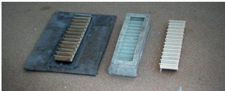
On the left is the master. In the center is the mold made of the master, and on the right is the finished part.
