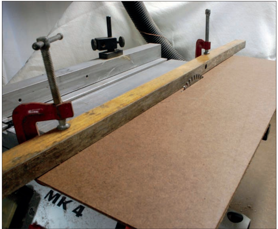
Here's a table saw fitted with a zero-clearance plate in the form of a sheet of Masonite hardboard. The zero-clearance throat prevents the wood from falling down into the saw hole.
