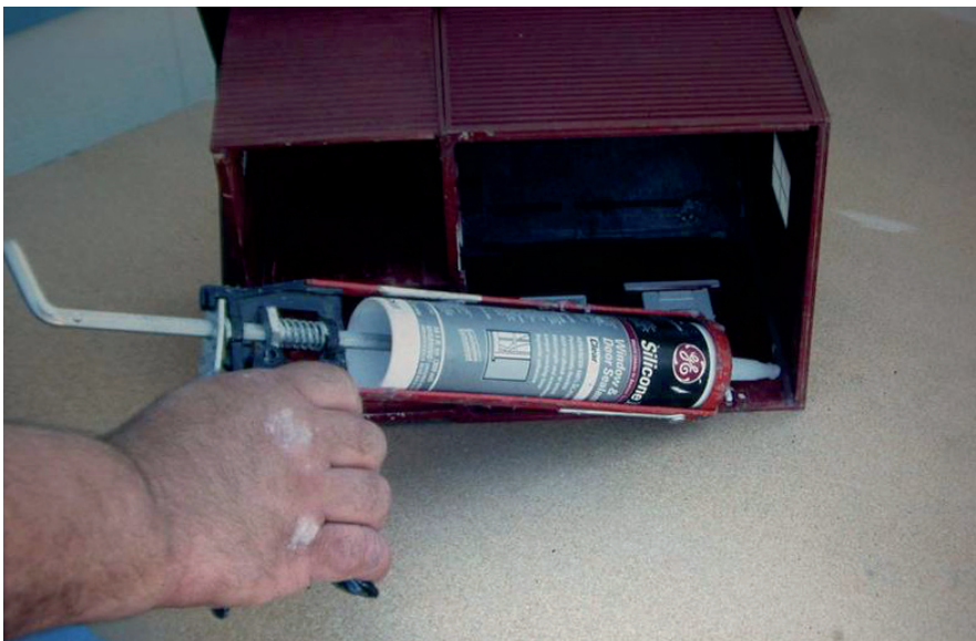
A Pola building receives silicone reinforcement in its joints. Silicone repels water and is tough, yet flexible, when dry.
