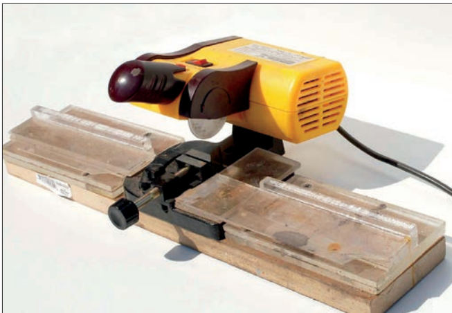
Mini chop saw. A large chop saw (not shown) is useful for cutting larger pieces of wood, but it's dangerous for cutting small strips of wood. A mini chop saw is a great tool for cutting small strip wood. The one shown has a 2" blade. I made my own table extension. This allows me to set up stops for duplicating parts. This saw can cut wood, plastic, and brass.
