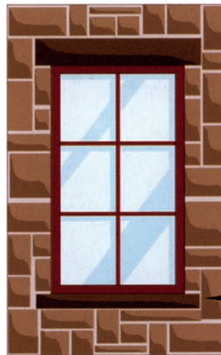
Heavy wood or stone lintel supports rockwork above window
