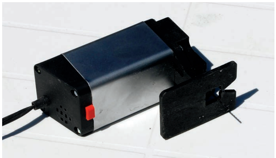
A miniature saber saw is less aggressive than a full size one, and is well suited for cutting out doors, windows, and arches in acrylic.
