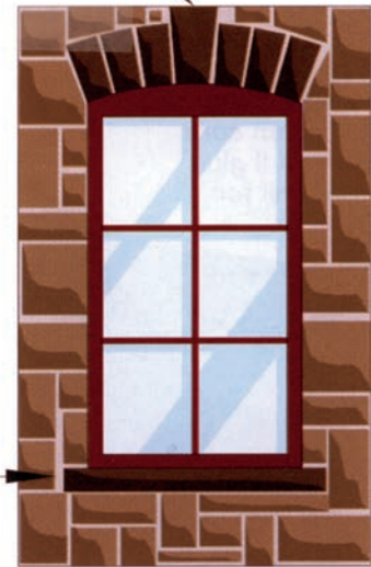
Stone arch supports rockwork above window
