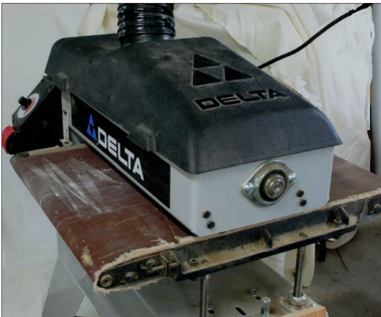
Thickness sander. This tool is designed to sand rough lumber to a specific thickness. Above is an example of a rough-cut "fence board" that has passed through the thickness sander. I also use this machine to finish the backsides of cast resin walls.
