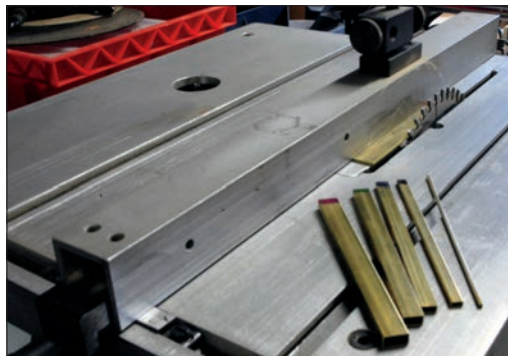
Here's a table saw fitted with a zero-clearance plate in the form of a sheet of Masonite hardboard. The zero-clearance throat prevents the wood from falling down into the saw hole.
