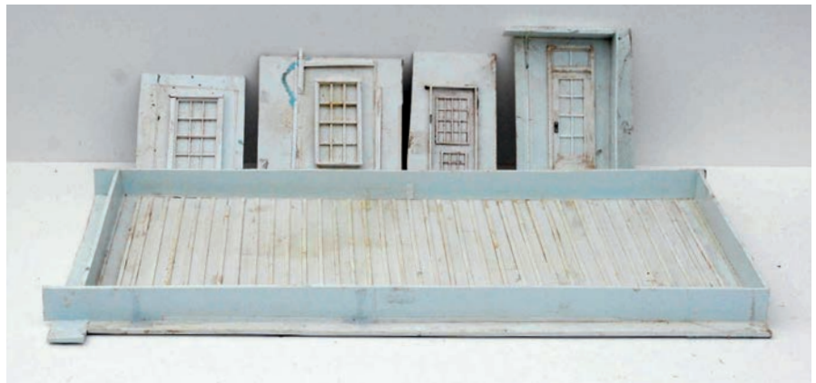
Here are several masters for making molds of windows, doors, and a wall section.
