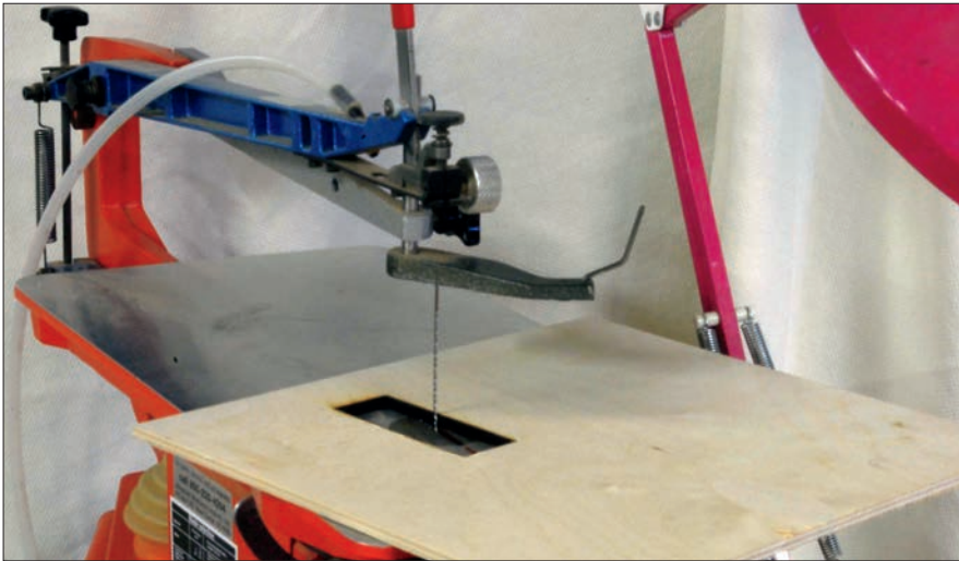
Scroll saw. A scroll saw is basically a powered version of a coping saw. Its advantage is speed. It can cut through materials quickly and accurately. A variety of cutting blades are available. For inside cuts, like windows and doors, drill a hole into the material, disconnect the blade and insert it into the hole, and then re-connect the blade back to the saw. A couple of disadvantages are this tool can vibrate the work piece if it not held down firmly by the operator. The blade moves too fast for cutting styrene so it will melt the plastic, trapping the blade in the work. It is not intended for straight cuts, as it is difficult to control.
