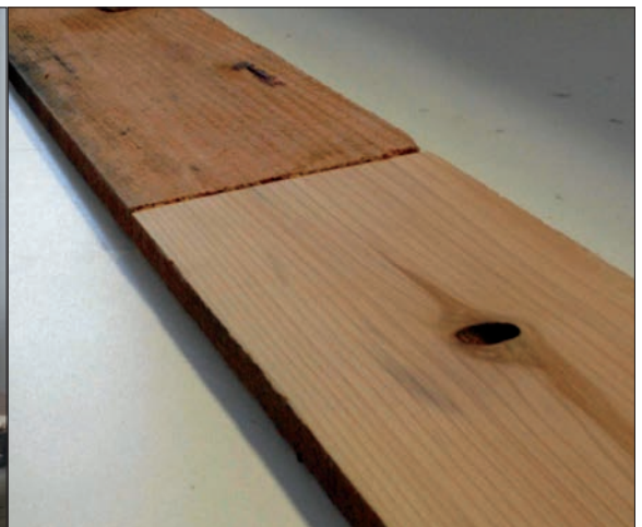
Thickness sander. This tool is designed to sand rough lumber to a specific thickness. Above is an example of a rough-cut "fence board" that has passed through the thickness sander. I also use this machine to finish the backsides of cast resin walls.
