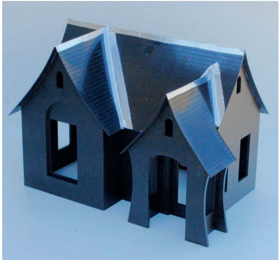
A 1/16"-thick ABS roof is glued in place. Aluminum duct tape is used as flashing.
