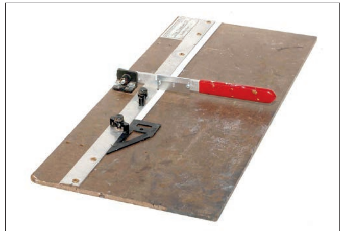
Chopper. The Chopper by NorthWest Short Line is used to cut wood or plastic strip material to length. It is good for making duplicate parts. The cutting arm holds a single-edge razor blade. Materials are placed in position on the table, then the arm is pushed down, cutting the material. A fence and a positioning block hold the material being cut to ensure a straight edge.
