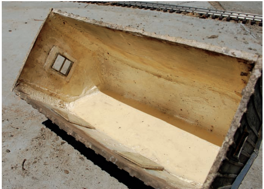
Resin was used to reinforce the joints of this resin structure. The thickening agent Cab-O-Sil was added to prevent the resin from running off while being applied.
