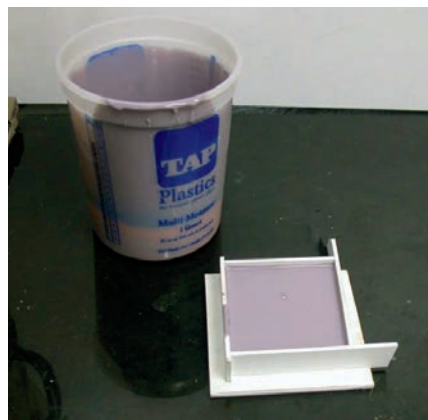
After the rubber is poured, tap the mold box on a hard surface to help remove any trapped air. Set it on a level surface and let it cure.
