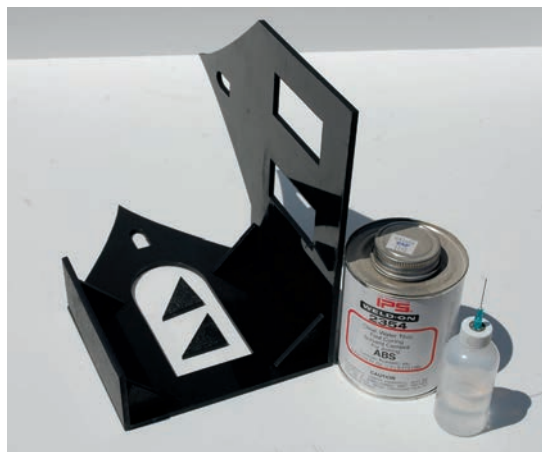
The walls are cemented together using Weld-on 2354, applied with a syringe bottle. Small triangular pieces are used in the corners mainly to keep the wall square. If the proper glue is used, no additional reinforcing is needed.
