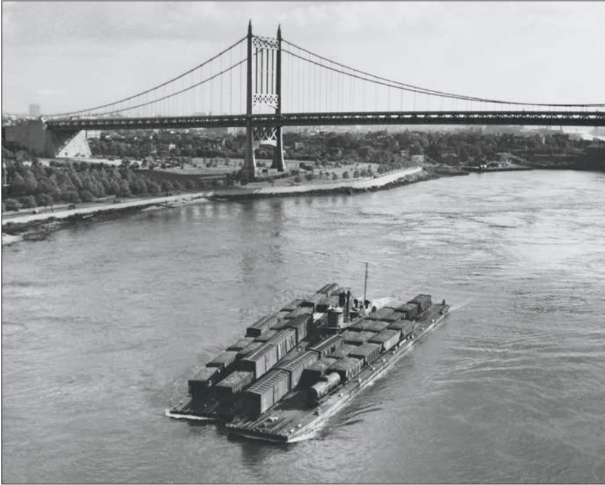
A New Haven tugboat guides two car floats under the Triborough bridge on its way to the docks at Oak Point. Each float could carry about 20 40-foot cars. Alfred F. Tyrill
