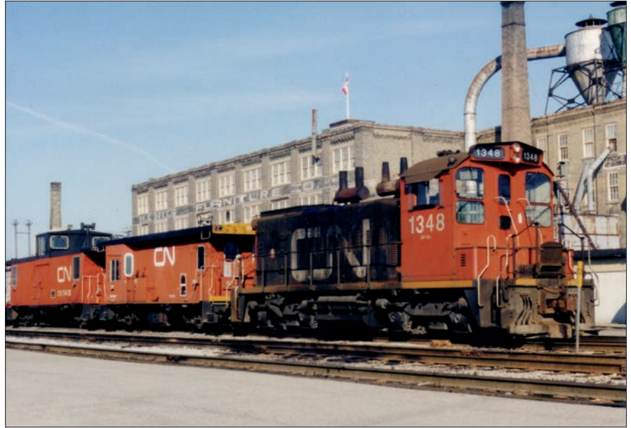
Essential equipment for a switching district includes a switch engine and road- and transfer-service cabooses. A Canadian National SW1200 rests at Kitchener, Ont., in 1987. Andrew Boyd
