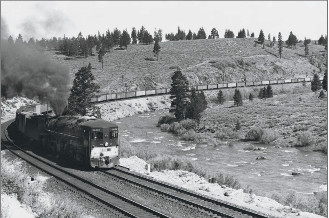
One of Southern Pacific's big Cab-Forwards leads a long string of ice-bunker refrigerator cars. David P. Morgan Library collection
