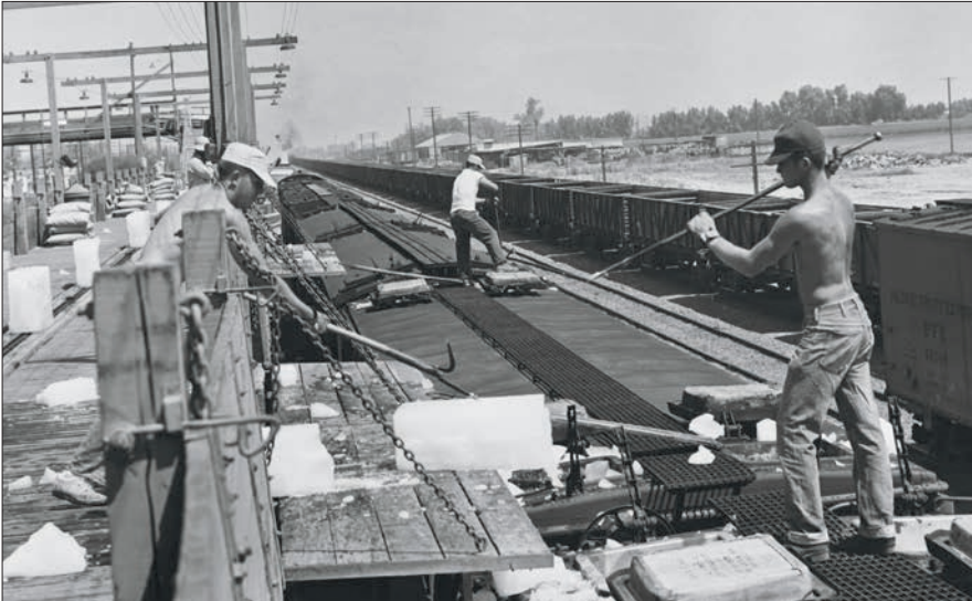
An icing crew skids 300-pound blocks into refrigerator-car bunkers at Coachella, Calif. Note the chain conveyor at left carrying the ice blocks along the platform. Donald Sims
