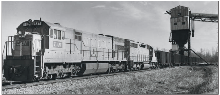
A large silo at the Cimarron Coal Co., near Madisonville, Ky., loads hopper cars as a pair of Louisville & Nashville diesels slowly pull the 70-car train under the tipple. L&N
