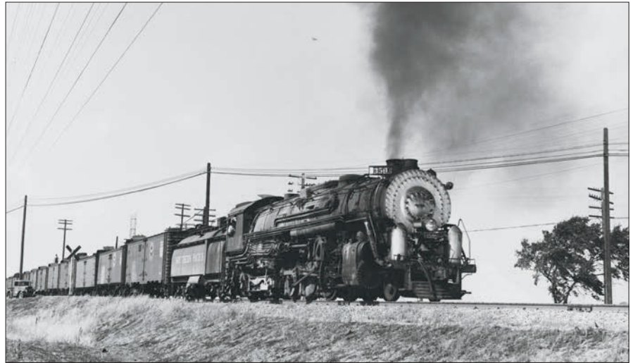
The real business of the San Joaquin Valley route was perishable traffic headed east. Number 3509 is a hefty 2-8-4 that started life on the Boston & Maine. Fred H. Matthews, Jr.
