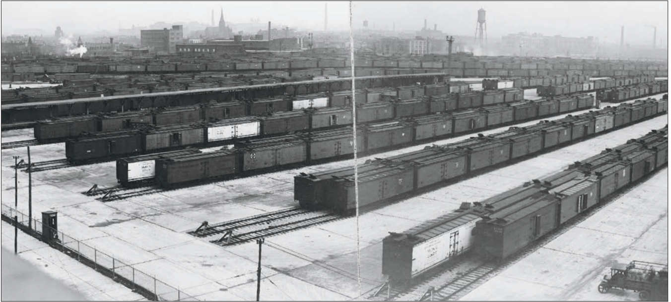
A sea of refrigerator cars await unloading at the Chicago & North Western's Wood Street Yard in Chicago. The yard's many pairs of team tracks allowed trucks to back up directly to the reefers for unloading. C&NW
