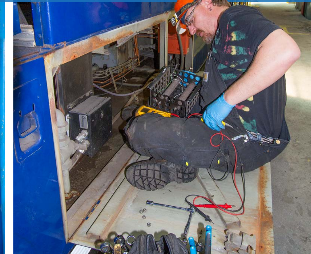
Opposite page: GP9 No. 130 awaits electrical repairs in the running-repair portion of Livingston's shop complex. Left: Shop workers' Blue Flag IDs hang from 130's cab to protect the workers from movement of the locomotive during maintenance. Right: Electrician Dave Marston checks electrical connections beneath the cab of the 56-year-old GP9.
