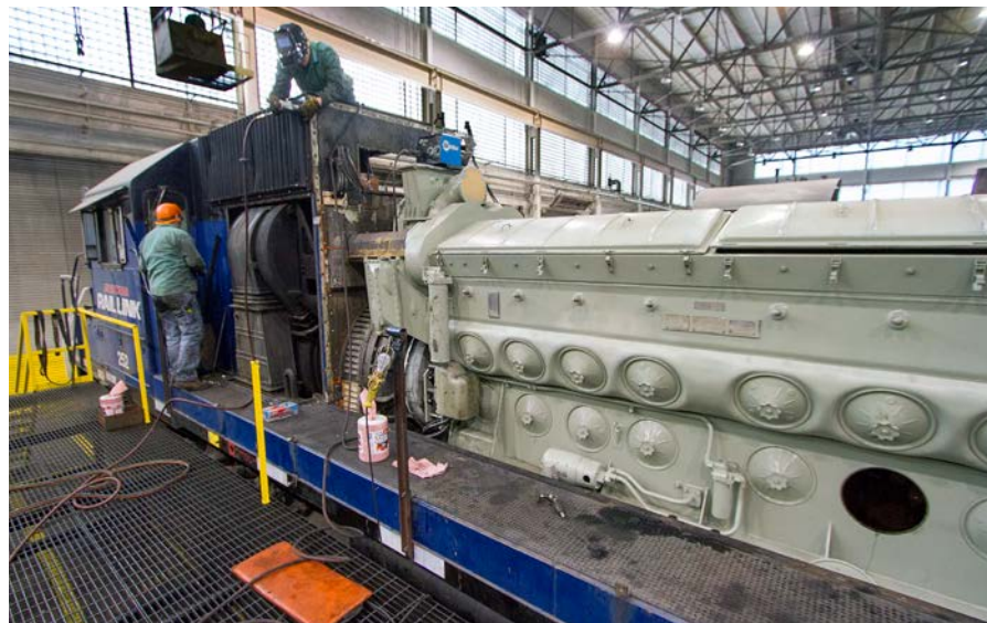
Shop machinists changed out Montana Rail Link SD40-2XR No. 252's prime mover and are now reassembling the locomotive.
