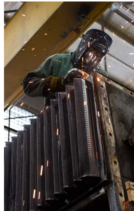
Tyler Verlanic welds on the inertial hatch of SD40-2XR No. 252.
