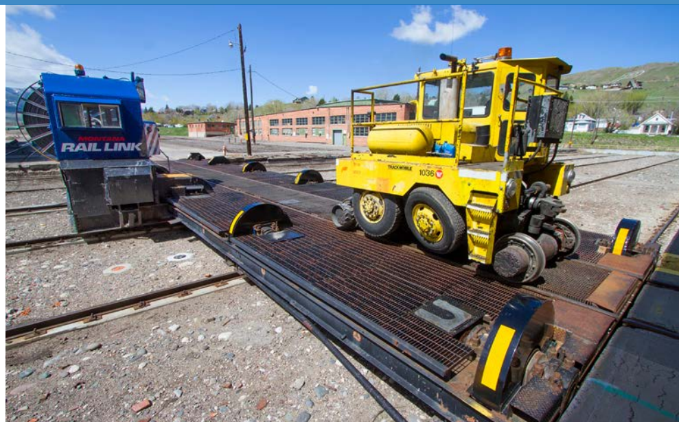
The cable-driven transfer table is lined up, and MRL Trackmobile No. 1036 heads into the main shop building to retrieve GP35 No. 401.
