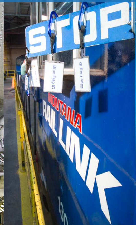
Opposite page: GP9 No. 130 awaits electrical repairs in the running-repair portion of Livingston's shop complex. Left: Shop workers' Blue Flag IDs hang from 130's cab to protect the workers from movement of the locomotive during maintenance. Right: Electrician Dave Marston checks electrical connections beneath the cab of the 56-year-old GP9.
