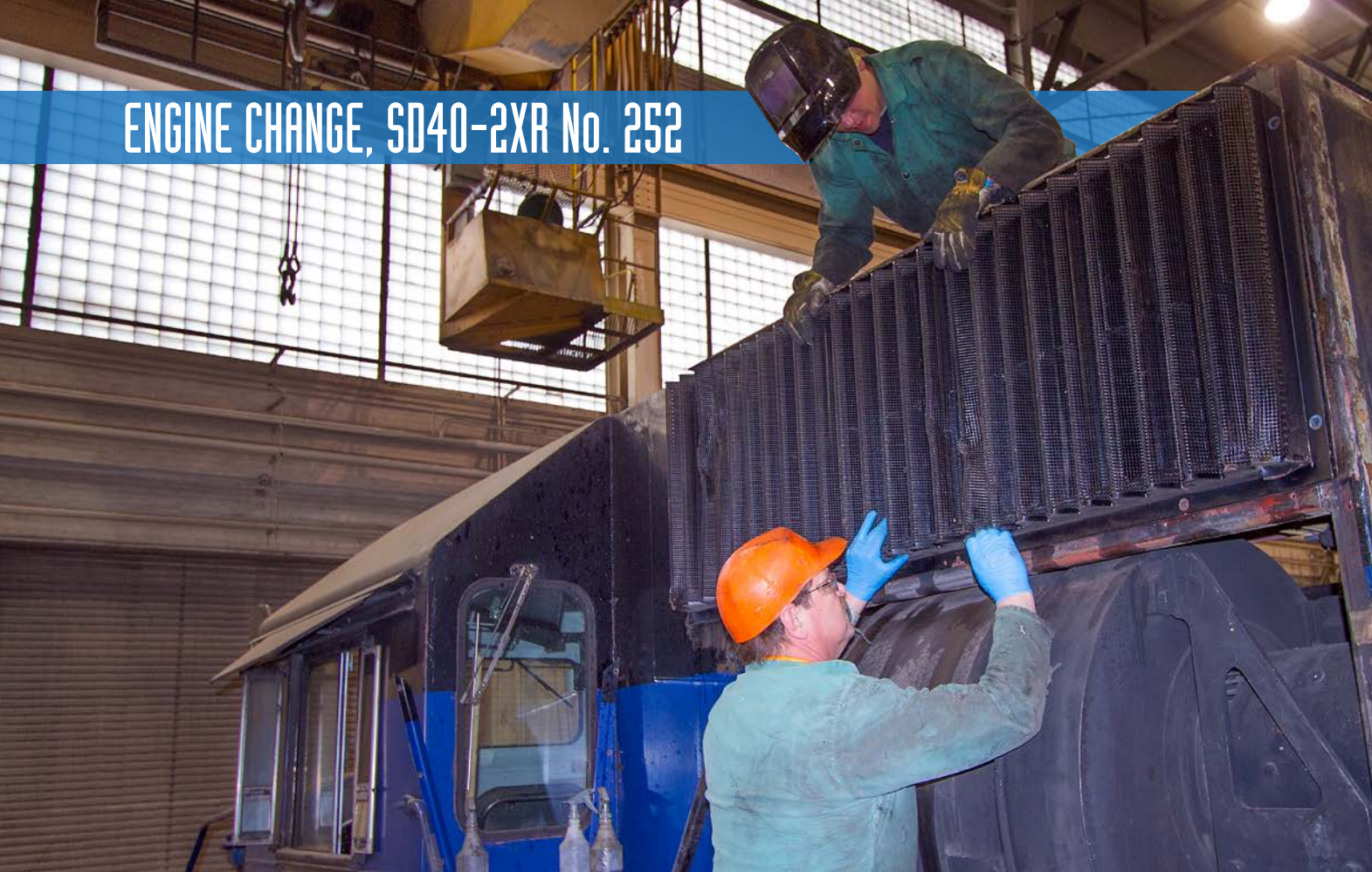
Machinists Tyler Verlanic (top) and Mike Donahue reattach the inertial screen on MRL SD40-2XR No. 252.
