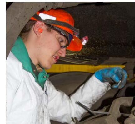
Electrician apprentice Nathan Krause inspects a traction motor brush.
