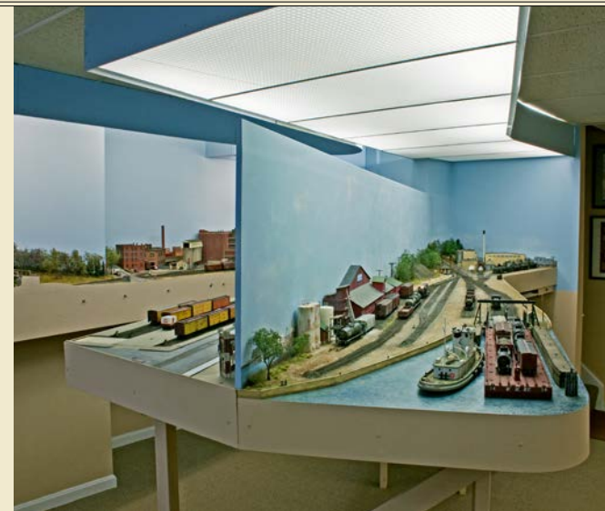
Clean fascia and an uncluttered room enhance the layout's appearance. Also, egg crate lighting diffusers were hung as a lower level suspended ceiling to hide the fluorescent tubes, especially when viewed from the peninsula end.
