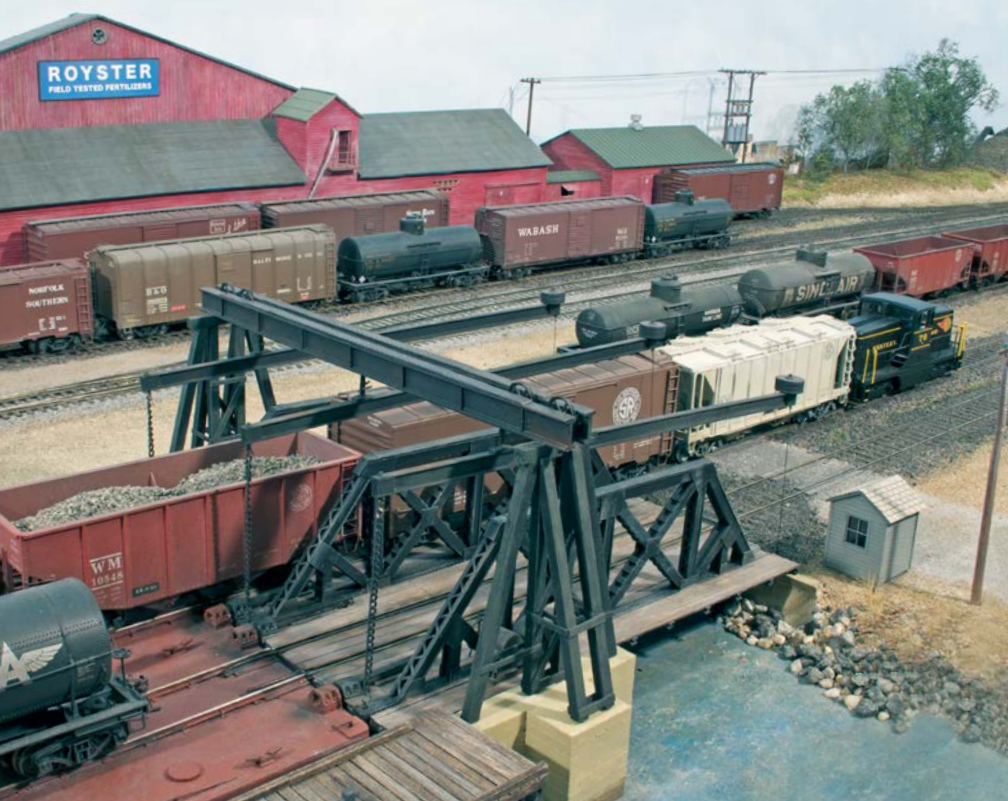
Fig. 5 Mind the gap. In the 1920s the Western Maryland installed unique counterweighted transfer bridges at several locations in Baltimore Harbor to service customers the railroad could not reach by land. Operators must take their time unloading the barge, taking into account the balance of the load.
