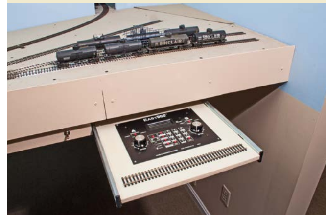
Pull-out shelves mounted on keyboard slide hardware provide a place for paperwork, pencils, coupler picks, and other items. This one does double duty by housing a Digital Command Control programming track and control panel. The shelf easily slides under the layout and out of sight when not in use.
