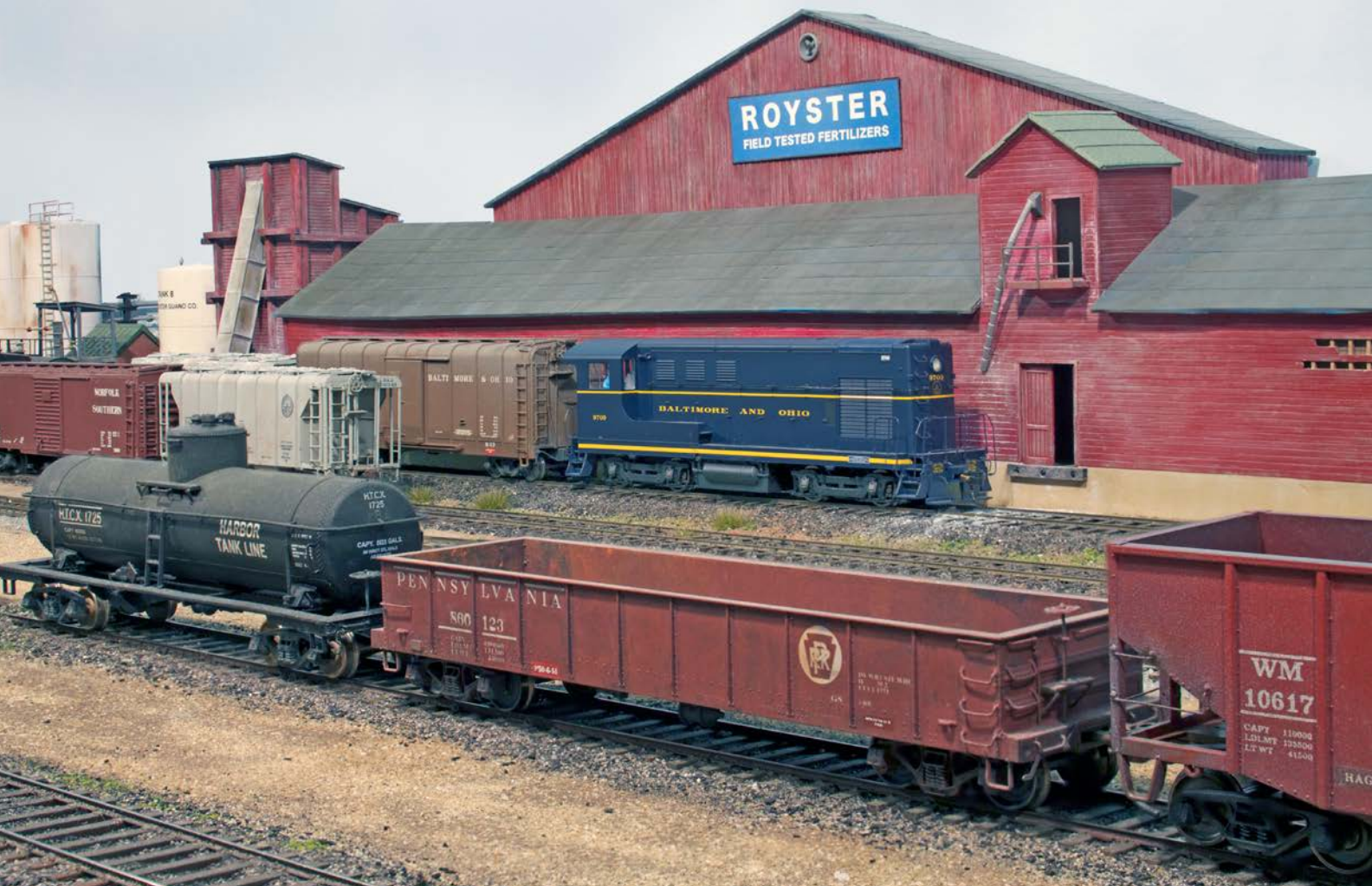
Fig. 4 Subtle changes. Paul used 1/8"-thick foam core board under the Royster fertilizer plant siding to raise the track's elevation. The mostly flat prototype called for modest track and earth height variations.
