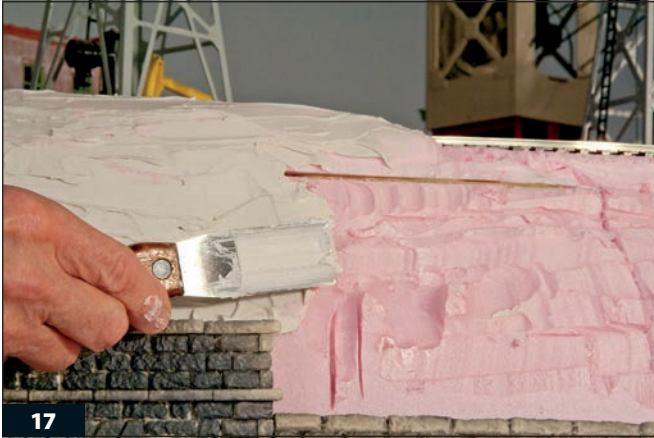
17 Coat the craggy hillside surfaces with drywall compound. Be sure to fill the gaps between the foam and retaining walls.
