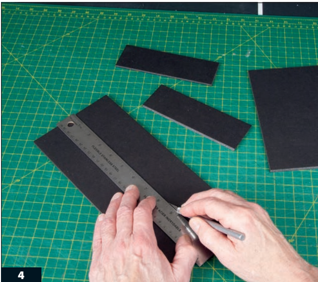
4 Use a sharp hobby knife to cut black foam core board into the pieces needed to build an enclosure for the DVD player.
