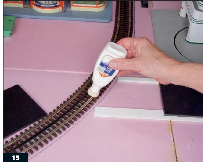
15 To build a grade crossing along a curved section of track, first spread white shoe polish along the rails.
