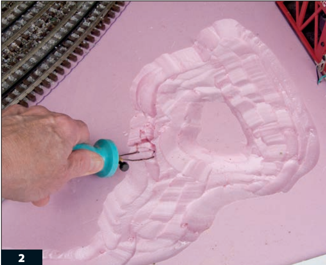
2 A round-tipped blade fitted to a hot wire tool makes it easy to carve out a shallow pond.
