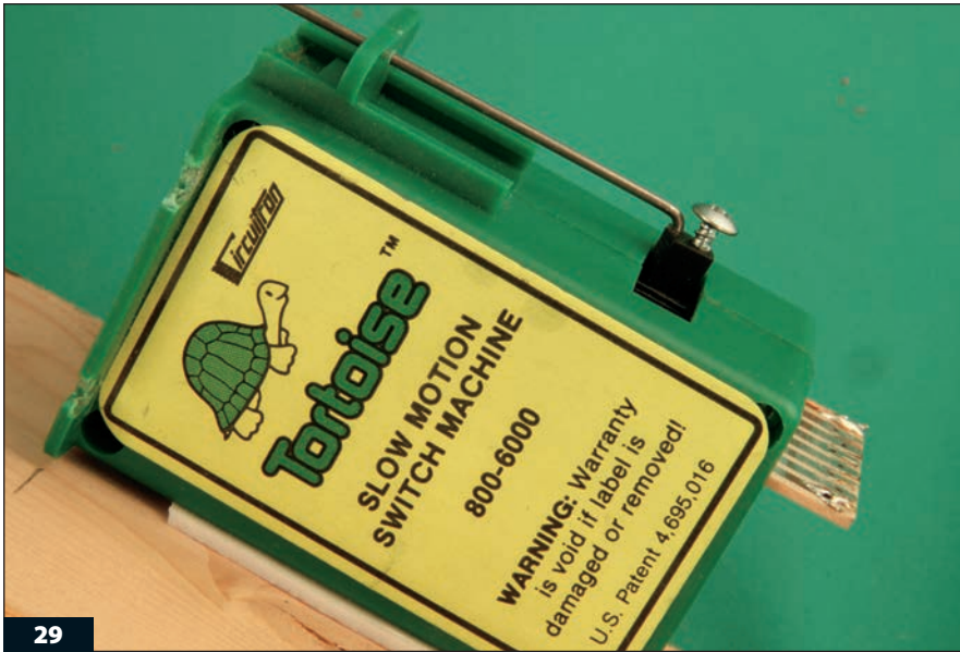
The metal rod supplied with the switch machine is too short to use here. Instead, use piano wire to form a longer rod.
