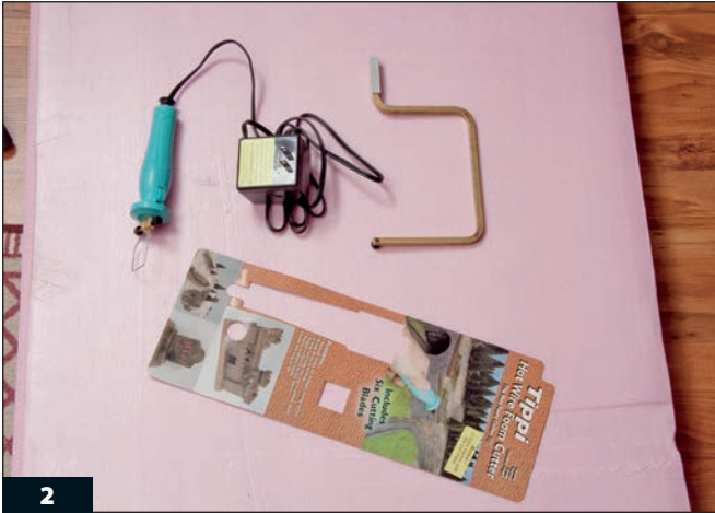
2 Although a knife blade or saw can be used to trim and shape foam board, a hot wire cutter is much easier and cleaner to use.
