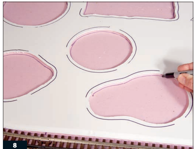
8 Return the foam core to the park area and mark the outline of each opening onto the foam tabletop.
