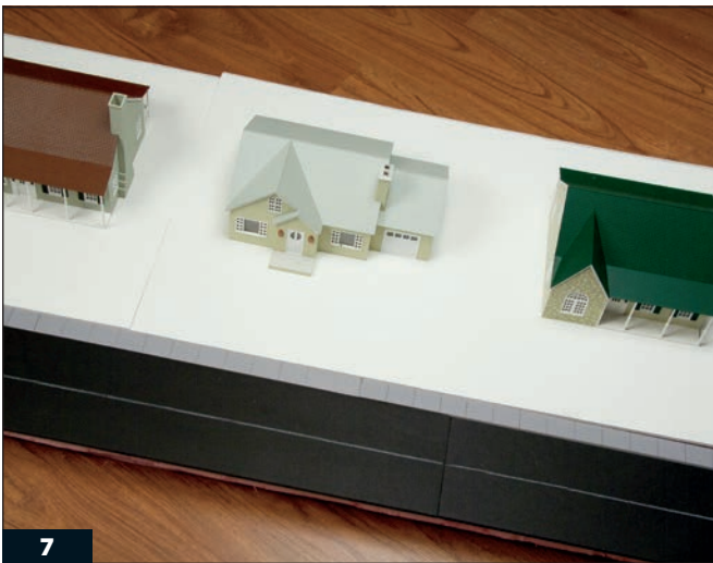
7 Assemble pieces of white illustration board over the hatch. Use this board to test-fit the arrangement of structures, roads, and sidewalks.
