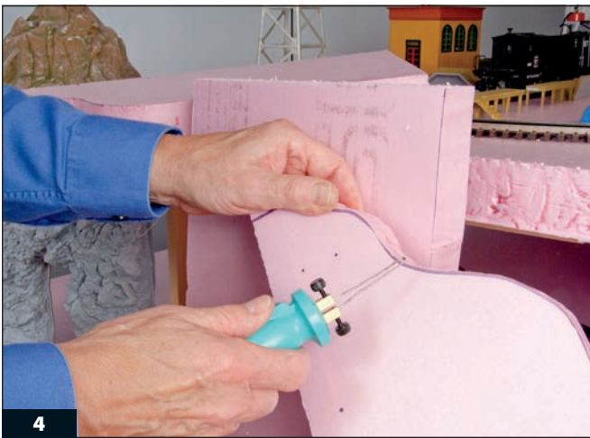
4 Avoid applying force to move the hot wire cutter through straight, curved, or beveled cuts. Always be sure to use the cutter in an area with adequate ventilation.
