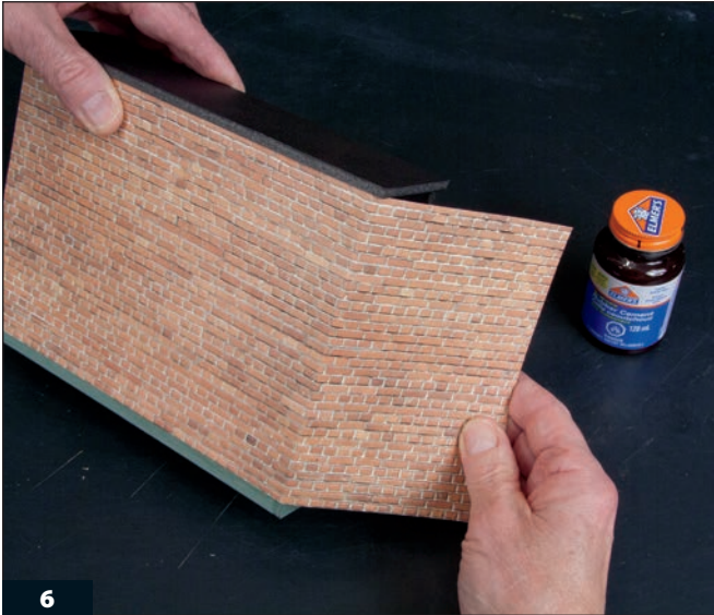
Use brick paper to laminate the walls of the enclosure. Trim the paper to fit between the roof and the painted foundation.
