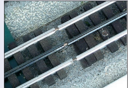
When the bridge is in place, the rails rest on top of the brass rods. The track should fit tightly over the rails.
