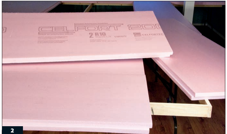
The edges of the foam panels are offset to interlock with one another, which makes them easy to fit together, especially when constructing a tabletop.
