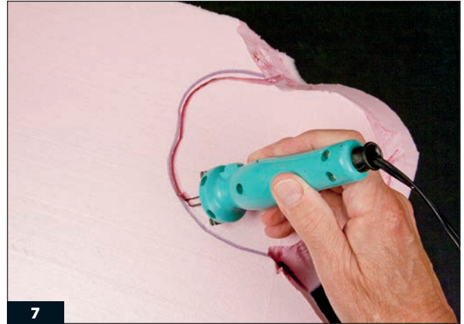
7 Use a hot wire cutter to cut out the second layer with a beveled edge. These rough cuts will be refined later, so don't worry if they don't follow the line precisely.
