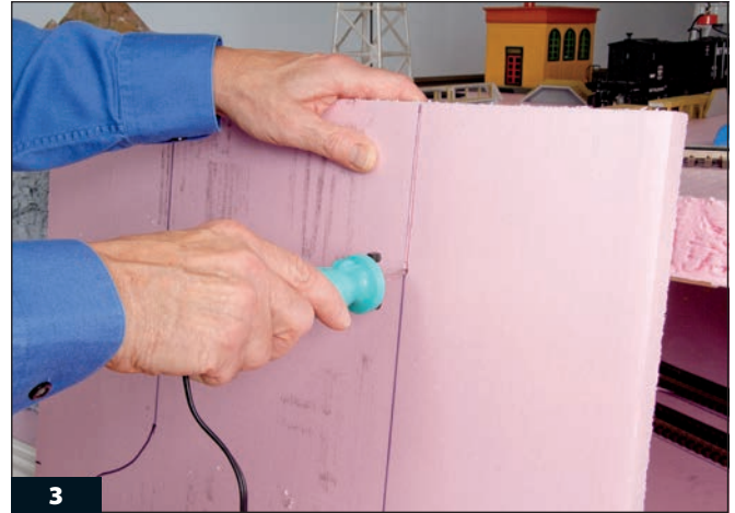
3 After marking cuts on the board surface, touch the tip of the cutter to the foam, activate the cutter, and allow the heat to melt the foam.
