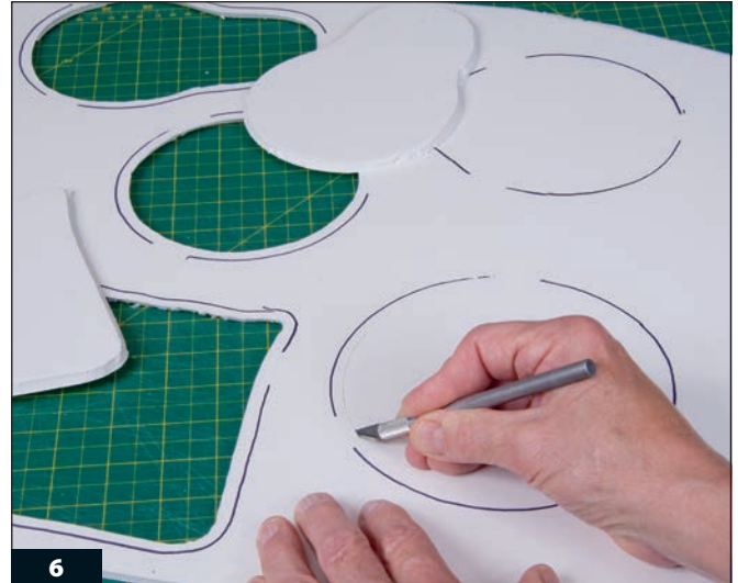
6 Remove the accessories and cut openings about 1/4" inside the marked outlines. Angle the hobby knife to make beveled cuts.
