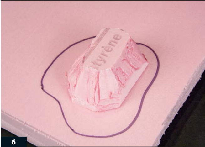
6 Carve the sides of the top section so that the base is wider than the top. Place this section on the next layer of foam and draw a wider outline around it.
