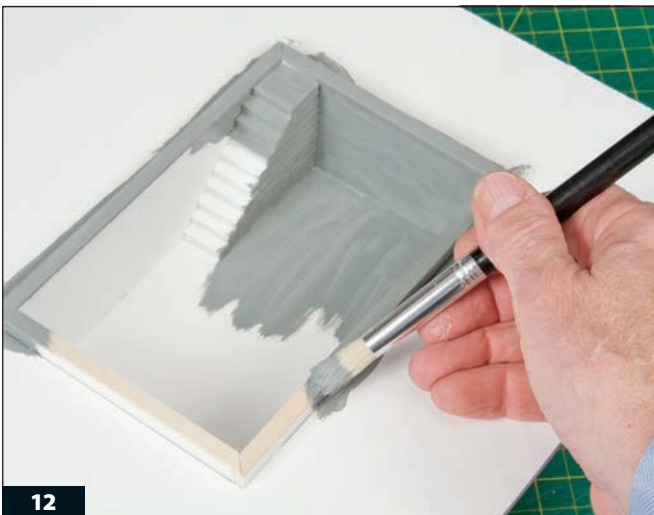
12 Let the glue along the sill pieces dry thoroughly, add a stairway, and then coat the entire foundation with gray, concrete-colored paint.
