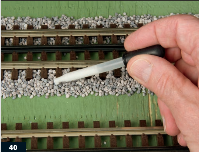
40 Load an eyedropper with matte medium and apply drops along the shoulder.
