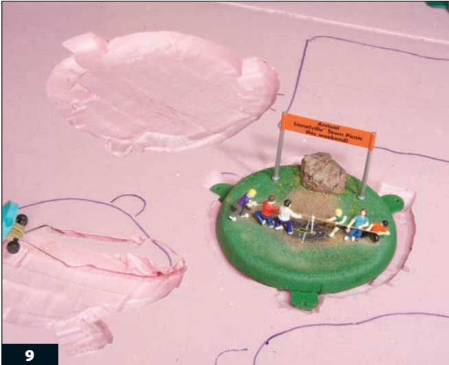
9 Use a hot wire tool to hollow out a shallow space beneath each accessory. Accessories should rise only \frac{3}{16} " above the tabletop.
