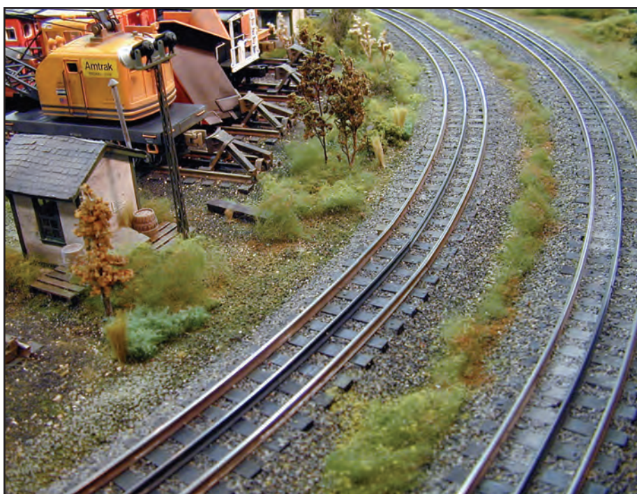
Even hi-rail track looks better when it has been properly ballasted. Ballast on model track serves the same function as on a prototype—it holds the ties and rail in place. Carl Chancey layout
