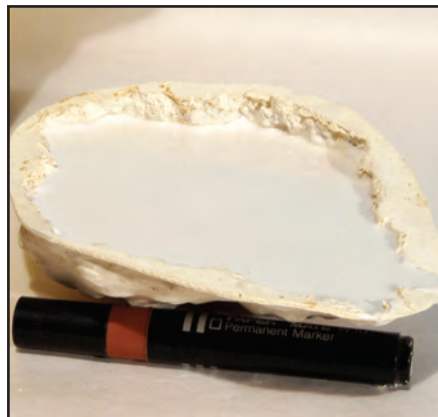
To cast rocks in place on the layout, begin by levelling the rock mold on your workbench and filling it with plaster.
