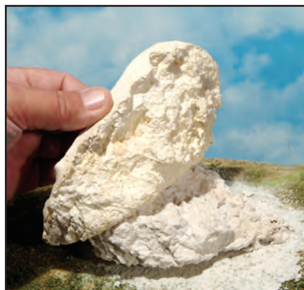
Hold the mold in place for 10 or 15 minutes until it gets warm. Then lift one edge to peek at the casting. The plaster should be hard enough so you can remove the mold without damaging the casting.
