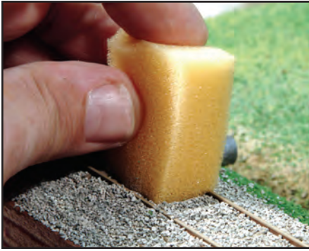
Use a piece of foam packing cut to the width of the rails to spread ballast. The foam will clear excess ballast off the tops of the ties.
