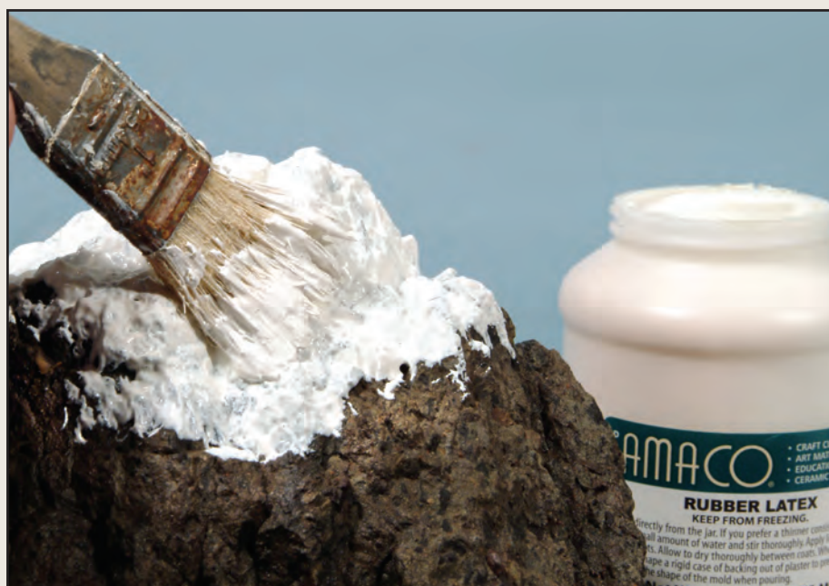
Take your time when applying the first coat of rubber on your rock master. Apply a thick, even coat, making sure to fill all the nooks and crannies of the rock surface. To allow for trimming the completed mold, make the mold about ½" larger all around than the item you want to cast.
