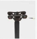
Model Wash (no. 76.521) with a paintbrush. This gives the trucks a slightly warm tone, like that of oxidized metal.
