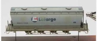
Weathering the cars was a fairly quick process using acrylic paints. I started by spraying the entire model with Vallejo Model Air White Gray (no. 71.119) thinned to a wash with airbrush thinner (no. 71.261), as seen at upper left. This helped tone down the original paint.
