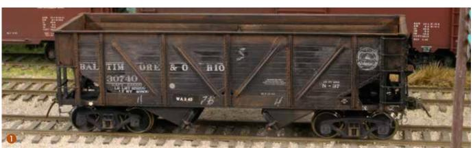
I followed this up with an application of Testor's Dullcote. I added a few drops of black to the Dullcote to help blend the lettering into the car sides.
