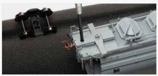
Next, I unscrewed the draft-gear box covers to remove the metal couplers. One end of the uncoupling lever is attached to the cover, so lift it off carefully. After the couplers were removed, I reattached the covers so they'd be weathered with the rest of the car.
