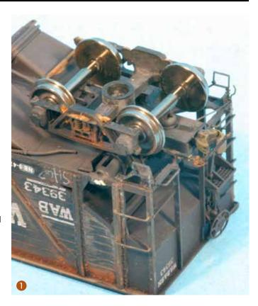
With the brackets in place, I added Hi-Tech Details rubber air hoses. After removing the parts from the sprue, I cut the shank to a long, pointed taper. Then I placed the shank into the brass casting and used tweezers to gently stretch it through. The shank returned to its normal shape, filling the hole without the need for adhesive. All of this can be seen in opposite page.
