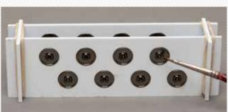
Normally I paint the wheelsets on freight cars with a Microbrush. But with 16 wheelsets to paint, I needed something quicker. I used a Modeler's Choice no. 236 wheelset painting jig [This product is no longer produced. Laser-cut acrylic jigs are available from American Model Builders and MinuteMan Scale Models. – Ed.]
