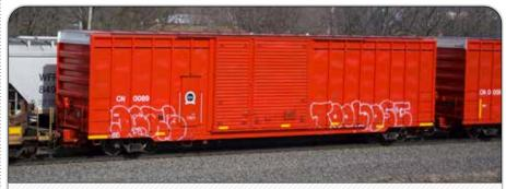
Canadian National distributed braking car 0069 is seen in a southbound intermodal train at Ackerville, Wis., on March 21, 2021. The built-in FRED is visible on the car end, next to the brake wheel. The car and three of its kind were being moved to summer storage. Cody Grivno photo
