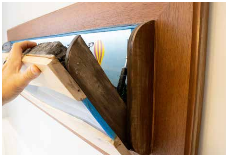
The arms are needed to swing the track (art piece) away from the fixed track (attached to frame) when folded up. If normal hinges were used the track would have folded into itself and not worked.
