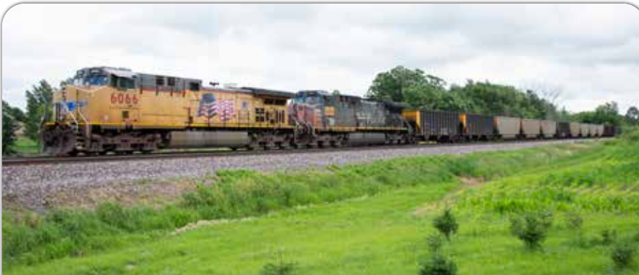
Two Union Pacific General Electric AC4400CW diesel locomotives are on the point of a Wisconsin Public Service unit coal train near Clyman Junction, Wis., on June 29, 2014. Note how the colored (rotary) ends of the coal gondolas all face forward. Cody Grivno photo
