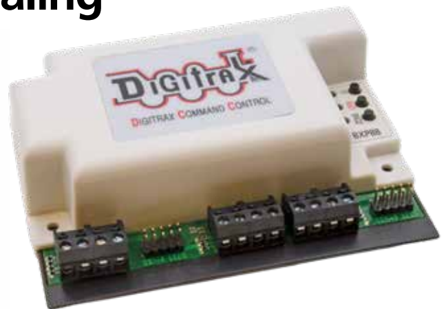
❷ Digitrax BXP88 eight-zone block detector. This device features a proprietary circuit that's very sensitive. The BXP88 detects transponders in locomotives and rolling stock.
