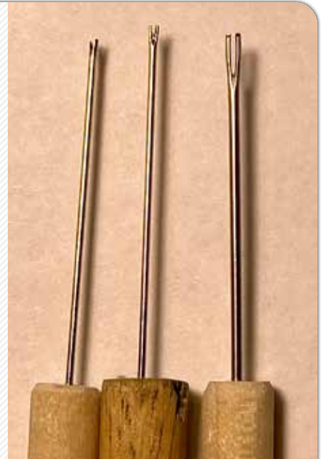
David Varholy cut off the ends of the eyes of three sewing needles and inserted them into dowels to make precision applicators. David Varholy photo
