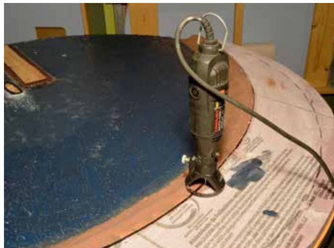
10 Mike used a motor tool with a router bit to cut a slot for the tempered hardboard backdrop to seat down into foam board before securing it to the vertical supports.
