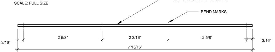
TRUSS ROD - CUT LENGTH AND BEND MARKS SCALE: FULL SIZE
