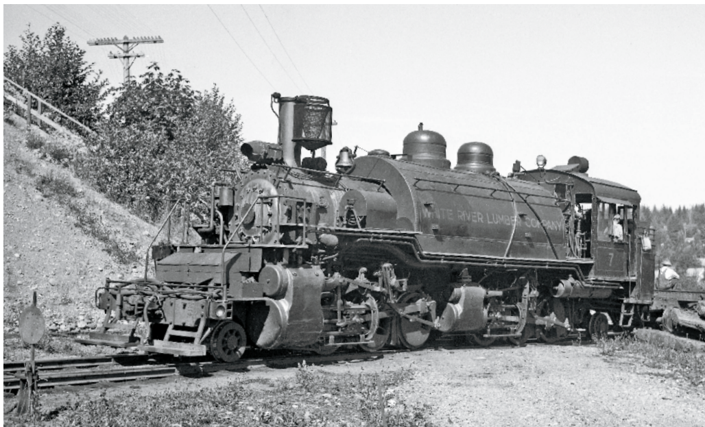
White River Lumber Co. 2-6-6-2T No. 7 shows off its full saddle tank at Enumclaw, Wash., on Sept. 10, 1946. No. 7 came from Saginaw Timber Co. of Aberdeen, Wash. Al Farrow, Martin E. Hansen collection
