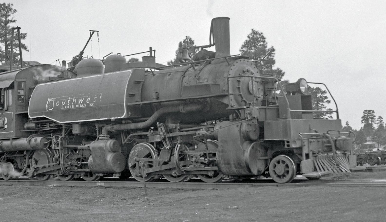
Southwest Lumber Mills 2-6-6-2 No. 12 displays a second configuration at Flagstaff, Ariz. The engine still sports saddle tanks but has lost its oil bunker and has acquired a rectangular tender. Ted Wurm, Martin E. Hansen collection
