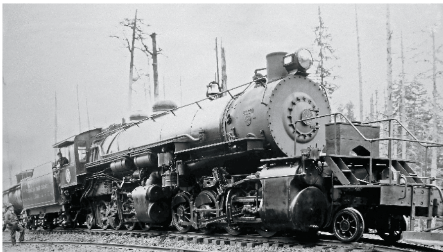
A true giant of the woods was Weyerhaeuser's 2-8-8-2 No. 200. Built by Baldwin in 1929, this and 1933 sister No. 201 were the largest logging locomotives built. Clark Kinsey, Martin E. Hansen collection
