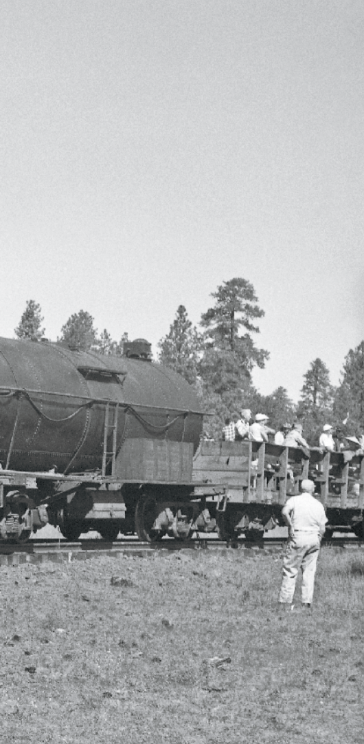
Southwest Lumber Mills No. 12 is shown soon after arriving in Arizona. The engine still has factory saddle tanks and oil bunker, with simply a round tank car added to provide more range. Martin E. Hansen collection
