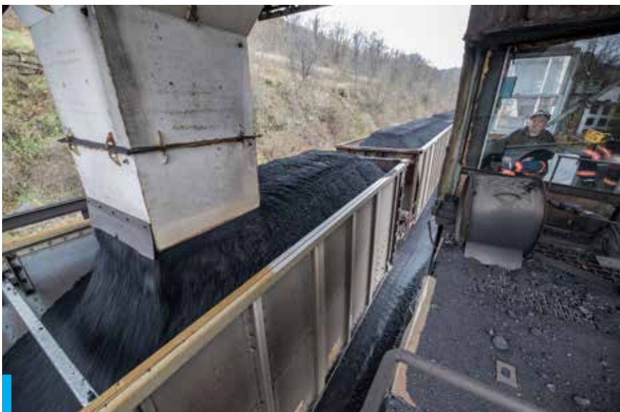
A Contura transportation employee carefully watches as the coal loader's loading shoot lowers and pours a smooth, even load into a slowly moving hopper. The crack of this car's springs groan as the load spreads like flowing water throughout the inside.
