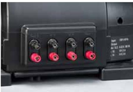
layouts what the classic Lionel ZW was to postwar layouts. The first modern, high-powered model railroad transformer to attain the Underwriter's Laboratory seal of approval, the Z-4000 helped hobbyists move away from 40-year-old ZWs. When first released in the late 1990s, it was in a class by itself, featuring built-in volt and amp meters, 400 watts of power, and the then-new banana plug.
