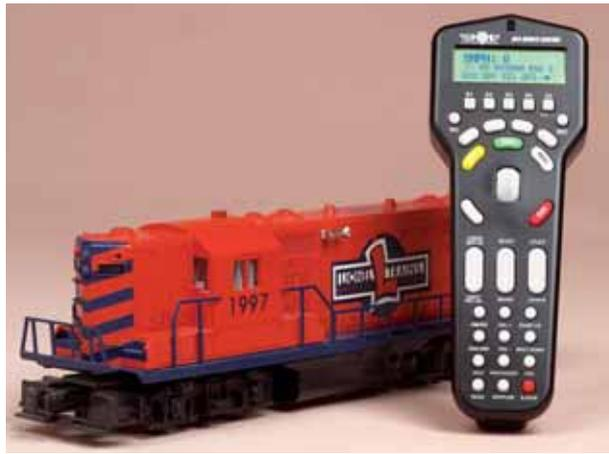
In addition to native ProtoSound 2.0 locomotives, MTH's DCS can operate any locomotive equipped with Lionel's TrainMaster Command Control in command mode. You can use the DCS hand-held controller or your Lionel CAB 1 controller.
