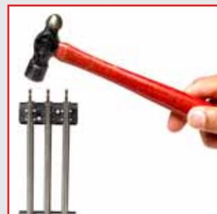
(about ¼ inch) so it breaks free of the rail crimp that grips the notch found on each end of a metal pin. Finally, grab hold of the pin with a pair of pliers, and you'll find it comes out easily, without deforming the end of the rail.
