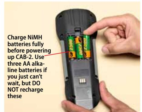
Charge NiMH batteries fully before powering up CAB-2. Use three AA alkaline batteries if you just can't wait, but DO NOT recharge these
