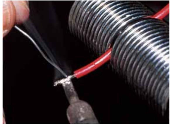
Fig. 3. To tin wire, first secure it facing down so gravity will draw off excess solder. Then place a drop of solder on the tip of your iron to conduct heat to the wire. Place the iron beneath the wire and additional solder above. As the new solder melts, pull the iron and solder down and off the wire.
