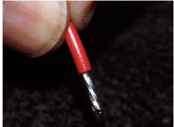
Fig. 4. When you have finished, the solder should saturate the wires yet leave the strands visible.
