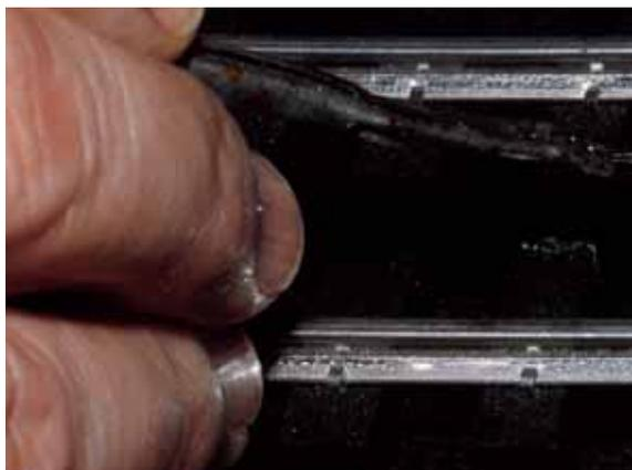
Fig. 5. Soldering a wire to track requires that you first remove any black oxide finish on the center rail. Then apply a coating of rosin-core flux on the rail.
