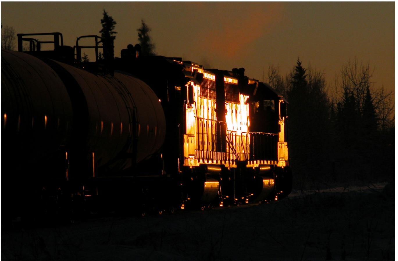
On cold days, locomotives idle in notch 3 to keep enough heat in the engines. Two GP40-2s hold at Chapados siding on Dec. 27, 2003.
