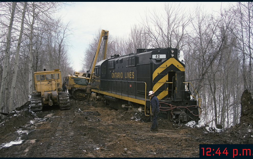
As Marv Winter directs, lifting his hands like a conductor, the winching begins (top). With the power of two bulldozers and two side booms, No. 40 begins to right, and a loud cheer goes up from the recovery crews and the railroaders (middle). Tears of joy streamed down one Ontario Midland employee's face. Finally, No. 40 is swung toward the center of the right-of-way (bottom) so the relatively uncomplicated re-railing process can begin.
