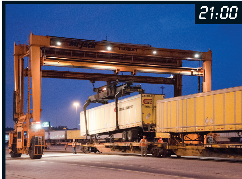
The last trailer is hoisted aboard the "San Bern." Fifteen minutes later the cars would depart the yard to back onto the rear cut a track over.
