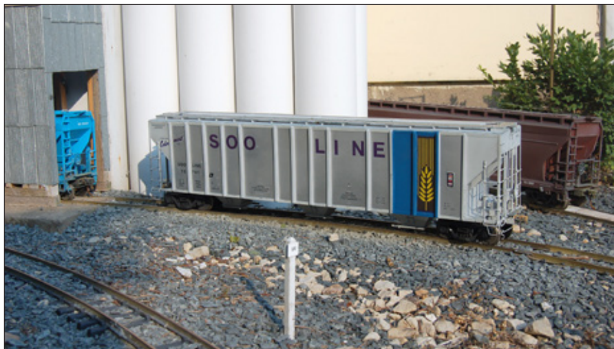
This scratchbuilt Soo Line aluminum Magor car, the pride of the author's fleet, was constructed by him from styrene and K&S structural parts. In 1970 the car would definitely be very clean. A boxwood tree graces the right side of the yard.
