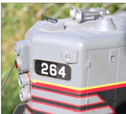
The Mars light on this locomotive (and others on the railroad) was scratchbuilt by the author. It is illuminated by the Sierra lighting circuit on the engine.
