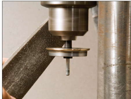
6. If you need to alter the profile of your wheels, nothing beats a lathe as the tool of choice (left). However, many people don't have lathes in their workshops. A drill press (center) makes a pretty good substitute. It's not as accurate but, in most cases, you can do a decent job of turning down the flanges. The end result is shown on the right. The left wheel has been turned down; the right is original.
