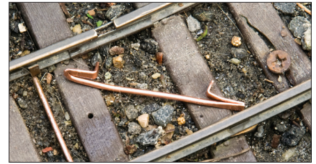
8. Sometimes, the gauge of your track will be too wide or narrow as a result of damage or other environmental factors. Here, the author used a copper gauge bar to hold kinked rails in gauge. If you're using track power, you'll need to use an insulator between the gauge bar and the rail, or use plastic or other non-conductive material for the bar itself.
