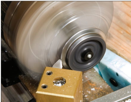
6. If you need to alter the profile of your wheels, nothing beats a lathe as the tool of choice (left). However, many people don't have lathes in their workshops. A drill press (center) makes a pretty good substitute. It's not as accurate but, in most cases, you can do a decent job of turning down the flanges. The end result is shown on the right. The left wheel has been turned down; the right is original.
