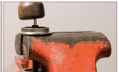
2. While there may be more elegant ways of adjusting the gauge of your wheels, a hammer and a vise provide a rudimentary-yet-effective means of doing so. On the left, tapping the end of the axle will result in the gauge being narrowed. On the right, the gauge will be widened.
