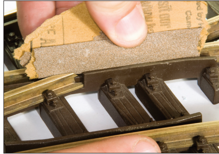
11. You may find that the back-to-back spacing of some of your equipment cannot be altered but is less than the span between the guard rails on your switches. You can remove a little material from the guard rail next to the frog in that case.
