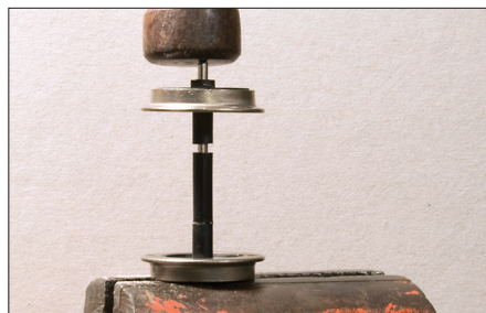
2. While there may be more elegant ways of adjusting the gauge of your wheels, a hammer and a vise provide a rudimentary-yet-effective means of doing so. On the left, tapping the end of the axle will result in the gauge being narrowed. On the right, the gauge will be widened.
