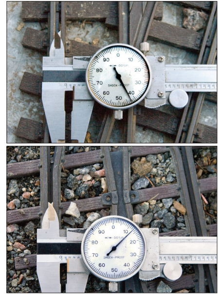
2. The clearance on switches varies greatly, depending on the manufacturer. Above, a Piko switch has fairly wide flangeways, measuring 0.142" (wider than "standard"). Below, a Sunset Valley switch flangeway measures 0.113", which is within G1MRA and NMRA standards.
