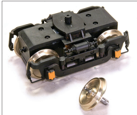
7. Replacement wheels for rolling stock are relatively easy to come by in a variety of diameters and materials (left). Replacements for locomotives are harder to find (right). These are from Northwest ShortLine, made for USA Trains and Aristo-Craft diesels.
