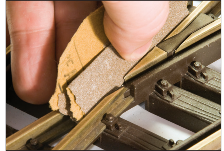
12. If your wheels have deep flanges or your switches have shallow flangeways, you may find it necessary to deepen the flangeway on the frog. A little sandpaper or a grinding wheel in your Dremel tool makes it so things don't go "bump" as often.
