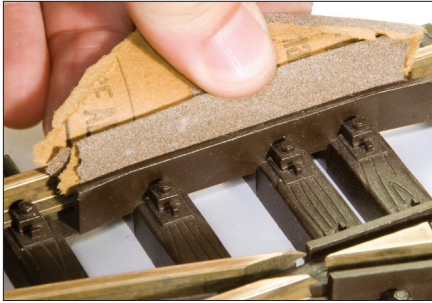
10. If the flangeway between the stock rail and the guard rail is too narrow, a little sanding can create more clearance.
