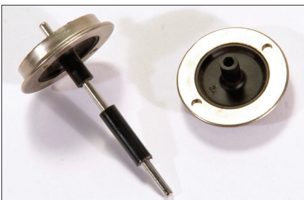
1. Many large-scale plastic wheels are simply pressed onto steel axles, which makes adjusting the gauge fairly simple.
