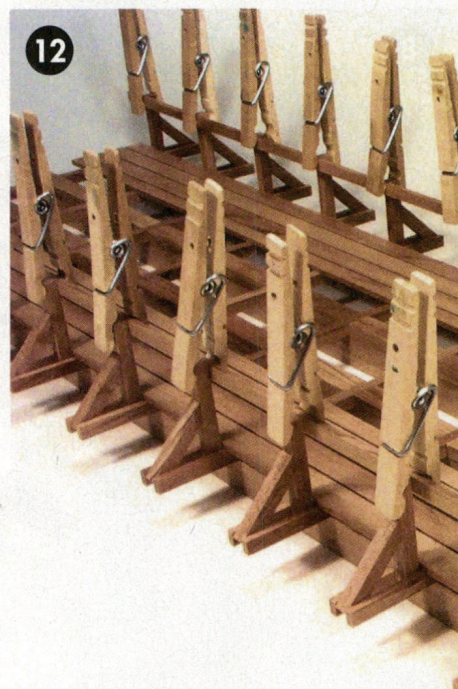
Top rails have been glued and clamped. The inside decking
