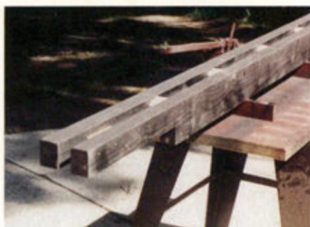
When the sides have been attached to each other, no screw heads show from the outside.
