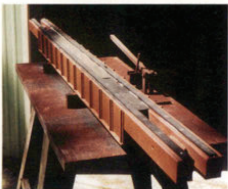
Track supports have been added to the top of the primed bridge. Only the side aprons remain.
