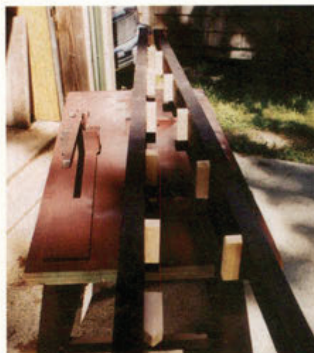
The wooden side plates have been painted black, but the spacer blocks were left natural for now for ease of construction. The blocks' top edges have been beveled for attachment with screws.
