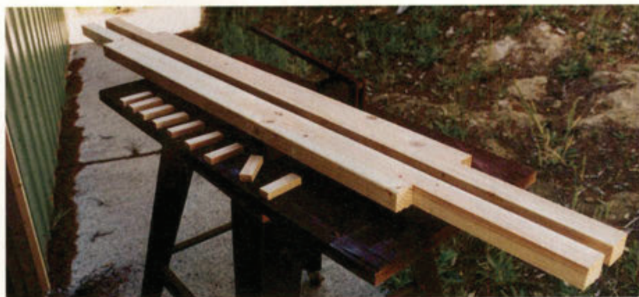
Two 2 x 4s have been trimmed and cut to shape. The spacer blocks (left) will be used between them to provide proper separation.
