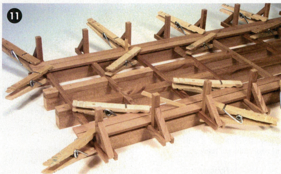
The decking is glued in place with the aid of clothespins. I put a little space between the pieces for looks.
