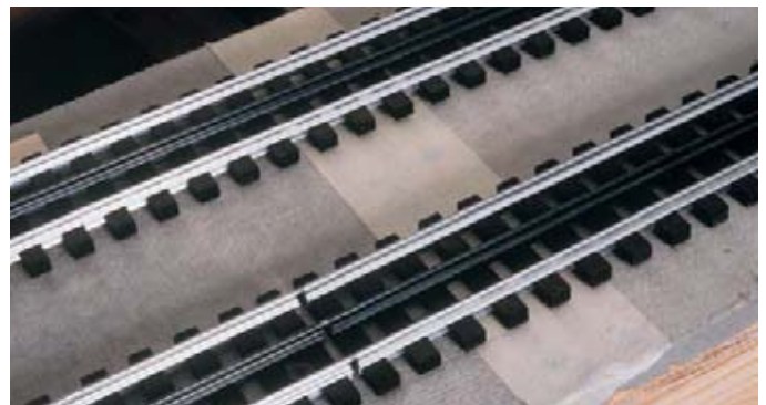
1. You can use Homasote for a solid base beneath your trackwork. Cover the seams between panels with masking tape.
