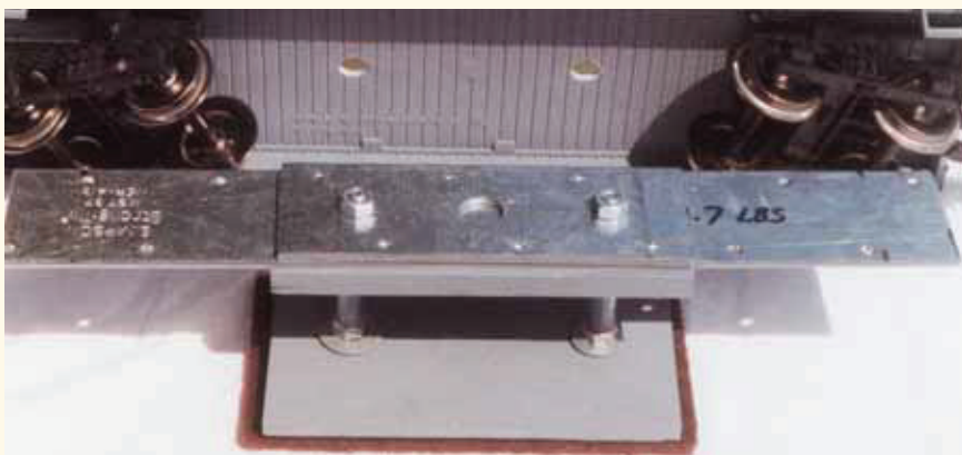
The cleaning assembly, assembled, outside of the car (for easier viewing). All detail has been removed from the bottom of the reefer.
