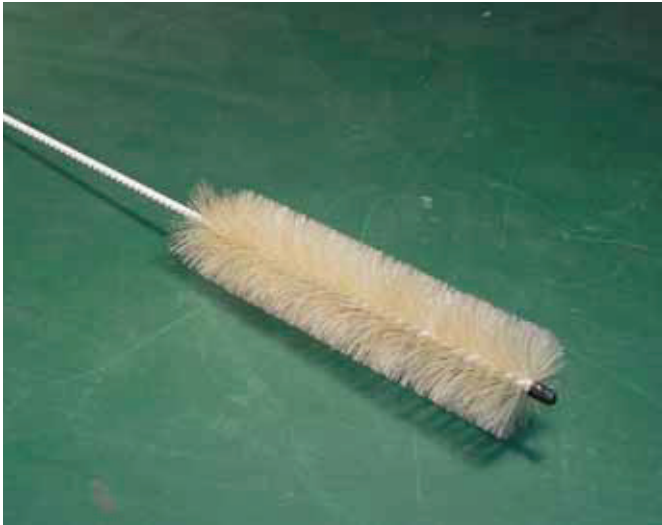
This brush, typically sold for cleaning bottles and pipes, forms the cleaning mechanism of the car.
