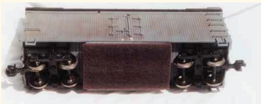
Make the cleaning area as large as possible without interfering with truck operation.
