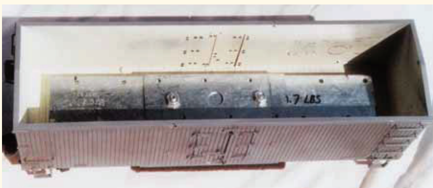
To assemble, insert the bolts from the bottom of the floor, then add the weight platform to the top side of the floor.
