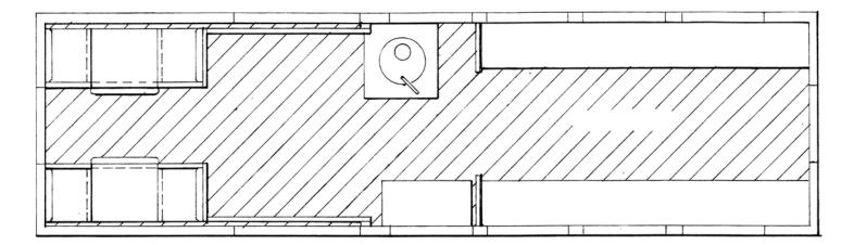
his drawing shows the interior layout that was in the SR&RL N° 556/557 caboose, with the exception that this car is wider than the original. Maine two-foot equipment was about 6' wide in the interior. Given that, gauge-1 track scales out to about 39" between railheads in 1:22.5 scale, instead of 24". We have widened the car so that it looks correct on gauge-1 track (or 0-gauge track, for that matter). With that in mind, shown here is a typical, double-
