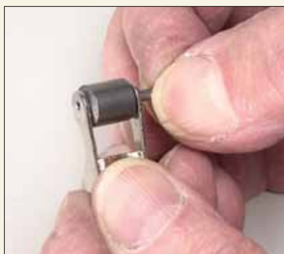
Fig. 9. With the new roller in position, push the new pin through the side of the arm that has the larger hole and then into the smaller hole.
