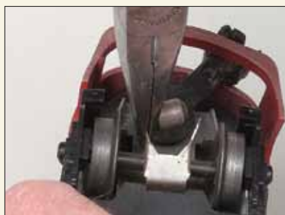
Fig. 5. With pliers, outwardly bend the side of the bracket that has the larger hole. Then do the same to the other side of the bracket.
