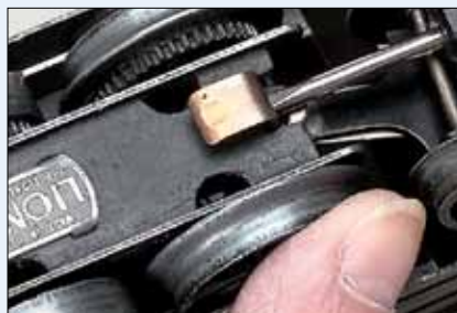
Fig. 3. To replace shoes, slide a screwdriver under the fiber bottom plate and between the shank of the shoe and the leaf spring clip until you feel the hook at the end of the shank.
