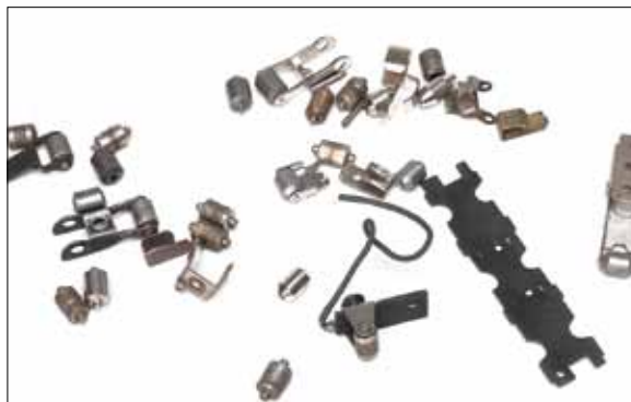
Rollers were made in many shapes and configurations. When replacing rollers, use the old one as a guide.
