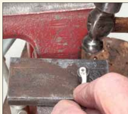
Fig. 10. Using a ball-peen hammer and an anvil, carefully tap the small-hole end of the roller pin until the pin is riveted in place.
