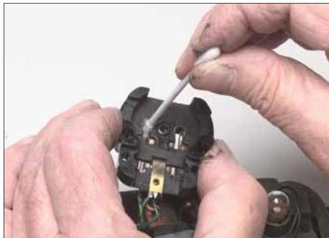
After removing the brushes, remove dirt from the brush wells with a cotton swab and a cleaning solvent.
