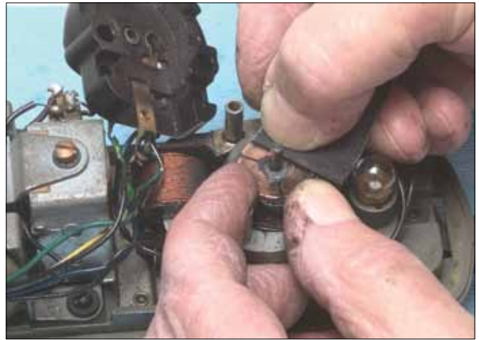
With an emery cloth, smooth and dress the commutator until all pits and grooves are gone.
