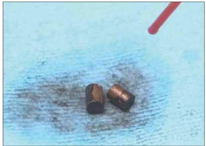
Clean the brushes thoroughly with a solvent and gently file the contact points, if needed.
