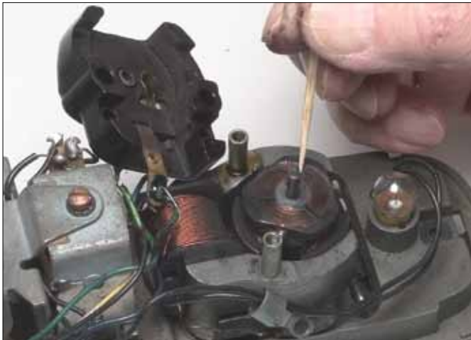
Use a toothpick to clean the gunk out of the gaps between the poles of the commutator.
