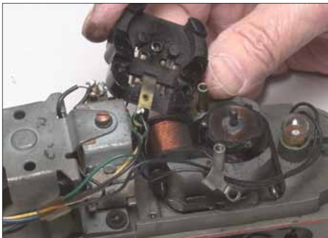
On diesels, the brush plate assembly must be removed to gain access to the commutator for cleaning. On some steamers, the commutator face is visible.
