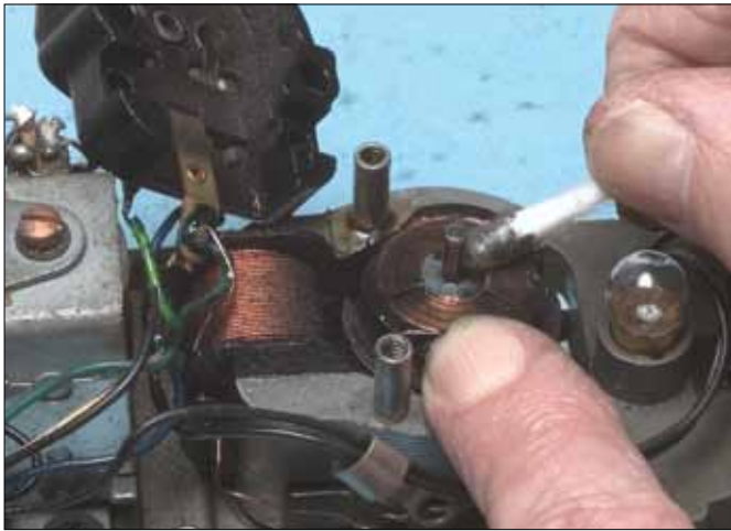
Remove the loosened dirt on and around the commutator surface with a cotton swab.
