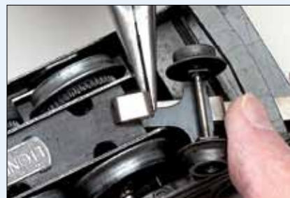
Fig. 4. Slide a new pickup shoe into position and listen for the click to confirm the pickup shoe has snapped into place properly.
