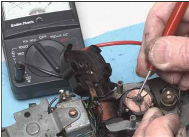
Use a volt-ohm meter to test the continuity between the segments of the commutator face.
