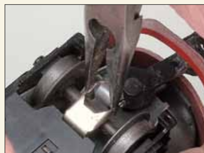
Fig. 6. Once you've installed the old pin and new roller, squeeze the bracket shut again, making sure the roller is able to turn freely.
