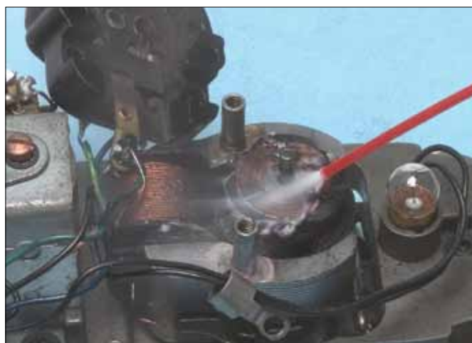
Clean the commutator surface with an aerosol cleaner/lubricant spray, such as LPS-1.
