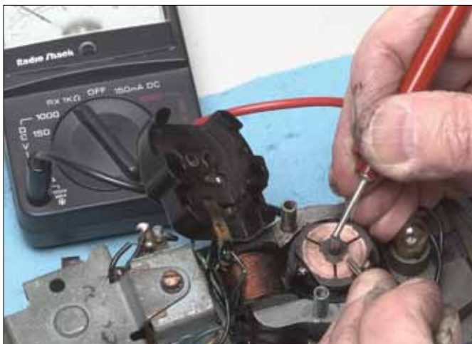
Also make sure there is no continuity between the commutator segments and the armature shaft.
