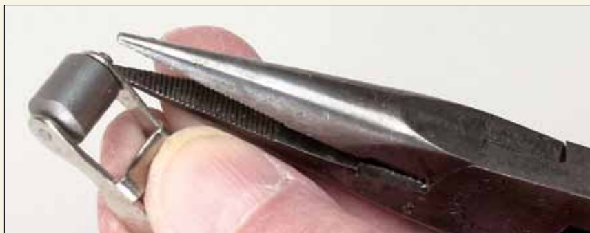
Fig. 8. When you've removed enough metal, use needle-nose pliers to remove the roller pin to release the old roller from the arm.
