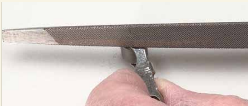
Fig. 7. After detaching the collector-arm assembly from the locomotive, file or grind off the end of the roller pin.
