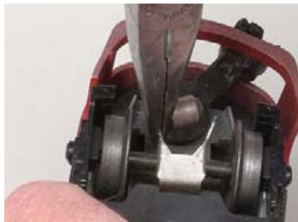
Fig. 5 – With pliers, outwardly bend the side of the bracket that has the larger hole, then do the same to the other side.
