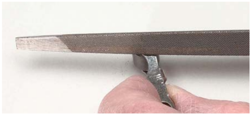
Fig. 7 – After detaching the collector arm assembly, file or grind off the end of the roller pin.
