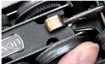
Fig. 3 – To replace shoes, slide a screwdriver under the fiber bottom plate and between the shank of the shoe and the leaf spring clip until you feel the hook at the end of the shank.
