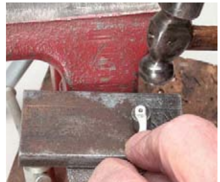
Fig. 10 – Using a ball-peen hammer and an anvil, tap the small-hole end of the roller pin until the pin is riveted in place.
