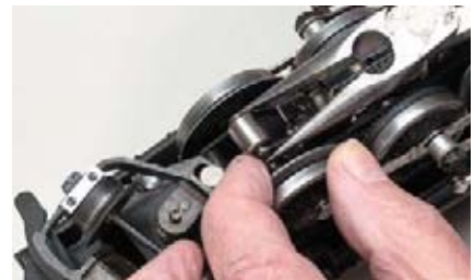
Fig. 2 – Use a pair of pliers to bend the collector arms back together to hold the new one-piece roller in place.
