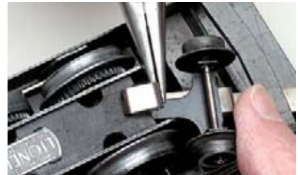
Fig. 4 – Slide a new pickup shoe into position and listen for the click to confirm it has snapped into place properly.
