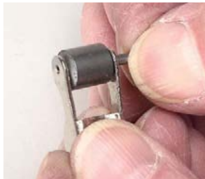
Fig. 9 – With the new roller in position, push the new pin through the side of the arm that has the larger hole and then into the smaller hole.
