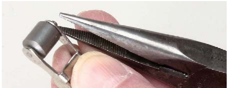
Fig. 8 – When you've removed enough metal, use pliers to remove the old roller from the arm.
