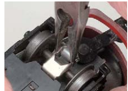
Fig. 6 – Once you’ve installed the old pin and new roller, squeeze the bracket shut again, making sure the roller turns freely.
