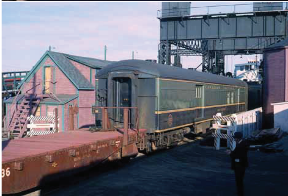
Three July 1963 photos show Canadian National's Prince Edward Island ferry operation. In a view from inside train 40 from Moncton, N.B. (top), cars are loaded aboard the Abegweit at Cape Tormentine. After the short voyage to Borden, P.E.I. (middle and above), a GE 70-tonner uses idler flats to retrieve the cars, which, still as train 40, will continue to Charlottetown.
