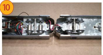
Here's another look at the six-pin tether that snakes from the power car at left to the baggage/coach car. After the photo was taken, I wrapped the wires in cloth friction tape to prevent chafing on the openings that I cut into the vestibules. The power car and baggage/coach car are easy enough to lift together with two hands, so the male and female ends of the tether will rarely be uncoupled.
