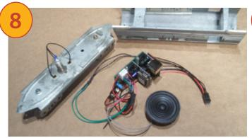
**Once I was satisfied** with my TMCC installation, it was time to move on to RailSounds. These are the RailSounds components before they were placed into the *Zephyr's* baggage/coach car. The male end of the tether is already soldered to its appropriate connections. Since I have no plans to run this *Zephyr* in conventional-control mode, I did not install a 9-volt backup battery – I covered the battery socket with electric tape.
