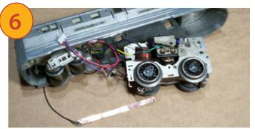
Here's the Zephyr after all the color-coded TMCC wiring has been soldered to the motor-and-drive mechanism according to the diagram in the instruction booklet. The shiny copper strip is the TMCC antenna. The unattached purple and pink wires next to the trailing truck will be cut and spliced into the tether connecting the power car to the RailSounds components in the baggage/coach car. The white plug fits into the RailSounds power board.
