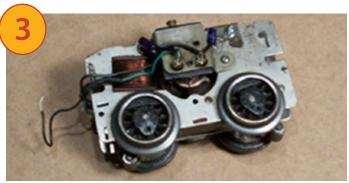
I identified the brush, field, pickup roller, and ground wires on the old Flyer motor-and-drive mechanism using a Lionel repair manual as a guide (there are no similar repair manuals for prewar Flyer trains). Then I drew my own wiring diagram so I wouldn't get confused. A capacitor (used to smooth the flow of electricity) must be connected to each of the motor brushes, which, for the *Zephyr*, turned out to be easy.
