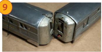
After installing the RailSounds boards in the front of the baggage/coach car (again up against the roof of the shell), I took a deep breath and made the only non-reversible modification to my *Zephyr* – cutting oval-shaped holes in the two vestibules for the six-pin tether connecting the Rail-Sounds and TMCC boards. The holes are at the lower edge of the vestibules (you can see the red wire).
