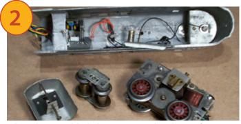
When disassembled, there seems to be plenty of room for the TMCC/RailSounds components. However, looks can be deceiving. The TMCC boards here are temporarily placed in the rear of the power car's shell. The motor-anddrive mechanism takes up most of the space in the center of the shell. A cast-in rear brace, sheet-metal light-bulb brackets, and stamped-metal vestibule eat up a lot of real estate on this model.
