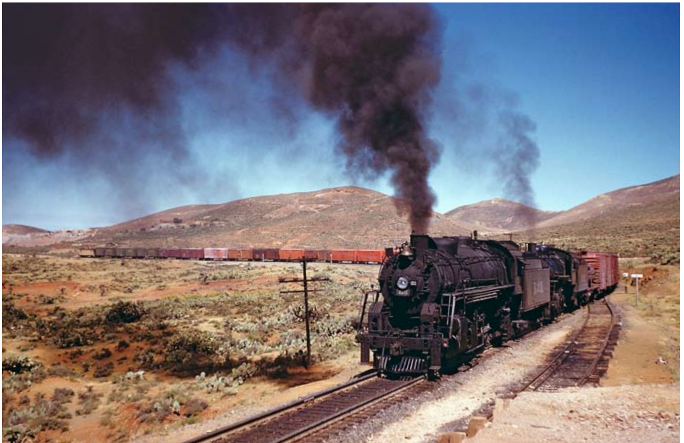
At El Grillo, the 2211 and 1414 are only about a mile and a half from the summit. Freights typically ran only about 2,000 tons on this grade.
