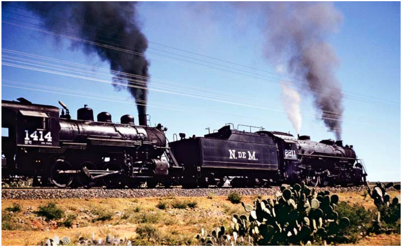
Still on the 1.5 percent grade, the 2211 and 1414 are working hard near El Bote. GR-34 class 1414 was one of 55 Cooke 2-8-0's of 1902-03.
