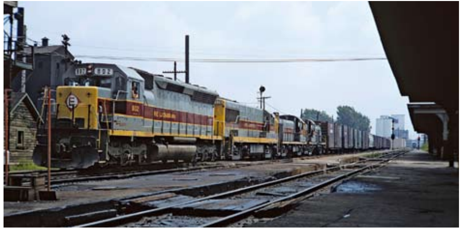
12:31 p.m. But first, a westbound 99-car EL freight shows up behind SD45 802, U25B 2506, and RS3's 1040 and 1051. EMD built the lead unit in 1966 as demonstrator 4352, one of three; Delaware & Hudson bought 'em, but in early '69 swapped 'em to EL for three GE U33C's.
