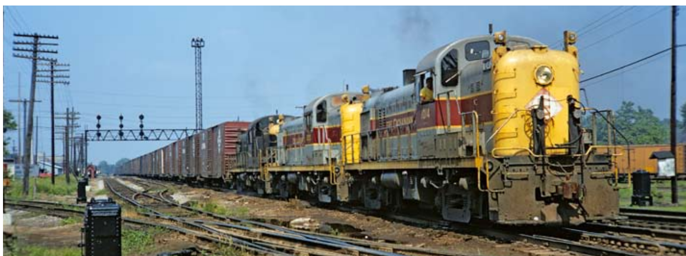
10:52 a.m. No dual controls here—EL 1014 is running “backwards” as it leads sister RS3’s 1033 and 1023 (still in Erie black) out of the yard with Marion-Mansfield freight 92. The train’s 100 cars are mostly auto-parts boxcars for Fisher Body, but it has 6 TOFC flats, too.
