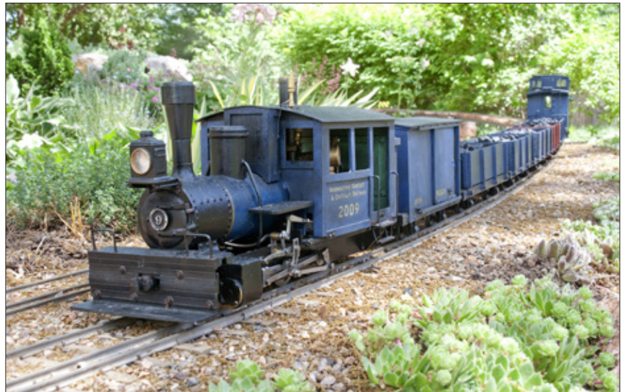
2. This train, hauled by a modified Roundhouse live-steam locomotive, is equipped with link-and-pin couplers as were the prototype cars. Kadee couplers are normally used on this line, so this coal train is also equipped with them at the ends—the link-and-pins are used only within the train. An interesting assortment of hen-and-chicks keeps ballast from washing down the retaining wall.
