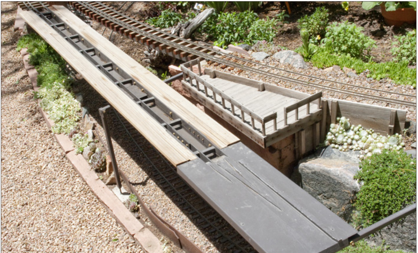
8. The dual-gauge steamup siding. A rerailer built into the end of track facilitates the placement of locomotives and rolling stock on the line.
