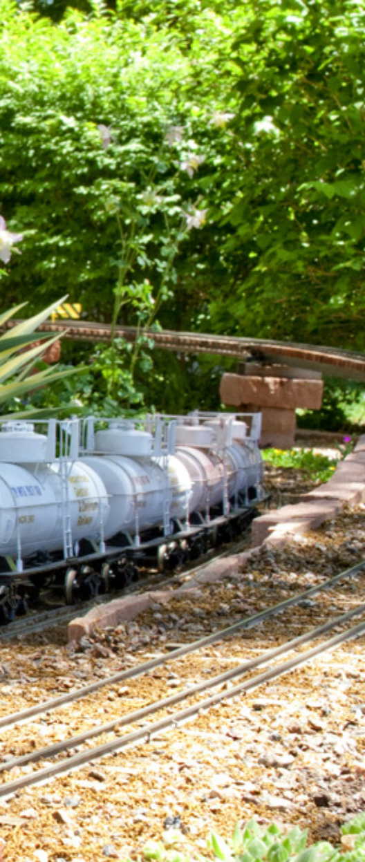
2. This train, hauled by a modified Roundhouse live-steam locomotive, is equipped with link-and-pin couplers as were the prototype cars. Kadee couplers are normally used on this line, so this coal train is also equipped with them at the ends—the link-and-pins are used only within the train. An interesting assortment of hen-and-chicks keeps ballast from washing down the retaining wall.
