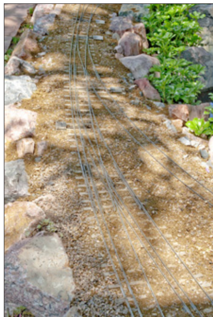
4b. The same switch installed in the railway. Wooden ties and small rail help the track to blend well with its surroundings.
