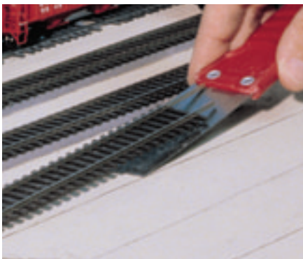
Fig. 4 REMOVING TRACK. One advantage of adhesive caulk is that it allows you to remove track without damage. In this photo, Chuck uses a putty knife to carefully lift a section of track. Chuck was even able to re-use some sections of track that he removed on other parts of the layout.
