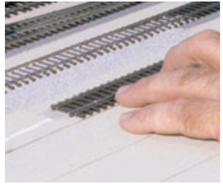
Fig. 3 PRESSING IT DOWN. Once Chuck had the caulk spread along the pencil guideline, he was ready to lay track. Since the caulk is very tacky, a mere press of the hands is all that is required to hold the track in place. A visual inspection helps ensure the track is aligned properly.
