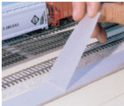
Fig. 5 TOPPER TAPE ON STRAIGHTS. For straight sections of track, Chuck leaves the protective skin on the tape while he applies it to the layout. Leaving the skin on keeps the tape straight and unstretched, and makes it easier to align along the pencil line.
