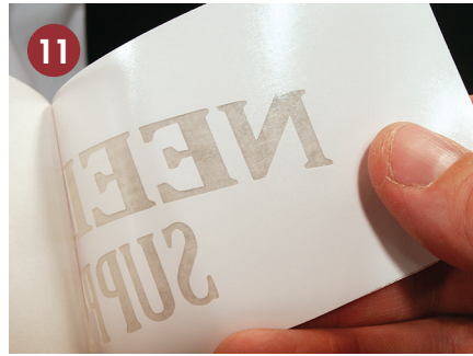
11 The protective backing is peeled away from the vinyl mask.
