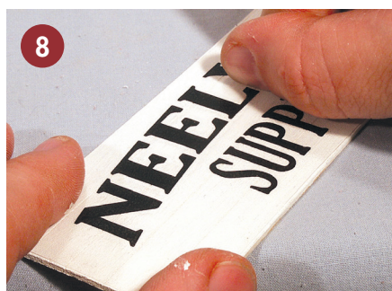
8 Rubbing the artwork with your fingers attaches the lettering to the surface.
