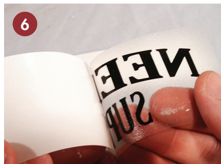
6 With vinyl lettering, the artwork and carrier sheet are carefully peeled off of the protective backing.
