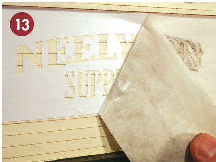
13 The front carrier film is removed, revealing the surface to be painted below.
