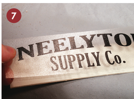
7 The artwork is then positioned on the sign front.
