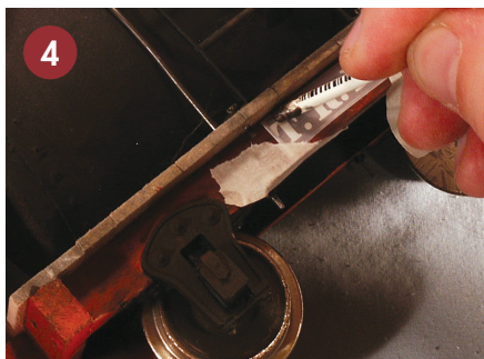
4 A burnisher presses the adhesive onto the model and releases the transfer from the carrier sheet.
