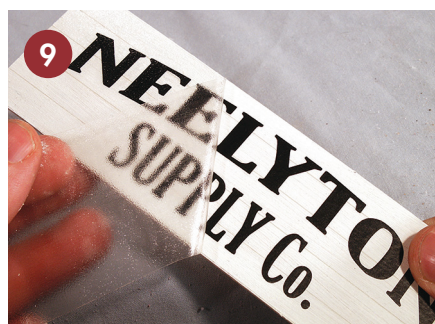
9 The carrier sheet is peeled away, leaving just the artwork.
