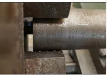
1. This photo illustrates what *not* to do—the piece is not gripped properly. No matter how tight you make the chuck, if you take too heavy a cut with your piece like this, it is going to go flying.
