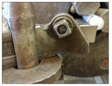
5. The correct setup for parting when using this type of tool post. Set the compound slide parallel to the lathe axis. To get the .333" length, turn the compound-rest dial .458". This will account for the thickness of the cutting tool.
