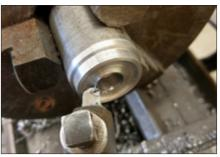
3. The round-end cutter has been ground for this job from ⁵₁₅" high-speed steel. Tools are cheap and you can regrind them again and again when they wear. Push the cutter into the face of the part until you are happy with the look.
