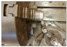
2. The compound rest is turned 20° to the vertical. Note how close the carriage is to the chuck jaws. Always check for clearance when working close to the chuck.
