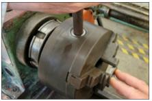
4. When you reverse the wheel to end-face the saw cut, it is important that the wheel spins true before cutting. Close the chuck on the wheel, back it off a little, then push with two fingers while gently tightening the chuck. Turn on the lathe and check that it is visually running true. Take a cut and measure in a couple of places. If you are within .002", it is good.
