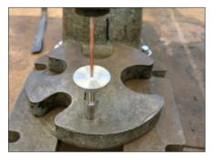
7. Line everything up as straight as you can and push the axle in. It will straighten itself. Once the wheelset is assembled, roll it on a table to check that it rolls straight. If not, the insulator is likely a little out of square. Press it back out and try again. If the insulator won't stay in on the second try, make another one.
