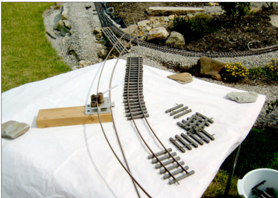
A card table provides a flat work surface at a comfortable height to thread rails onto tie strips. On the left, a rail bender is forming a rail with a four-foot-radius curve.
