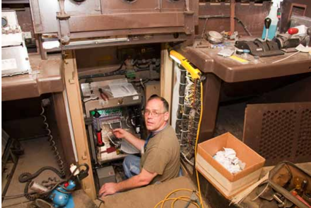
Locomotive technician Jack Johnson wires new cab signal equipment into the nose of P40 No. 837 on April 12, 2010. Beech Grove released the engine back into service on June 3.
