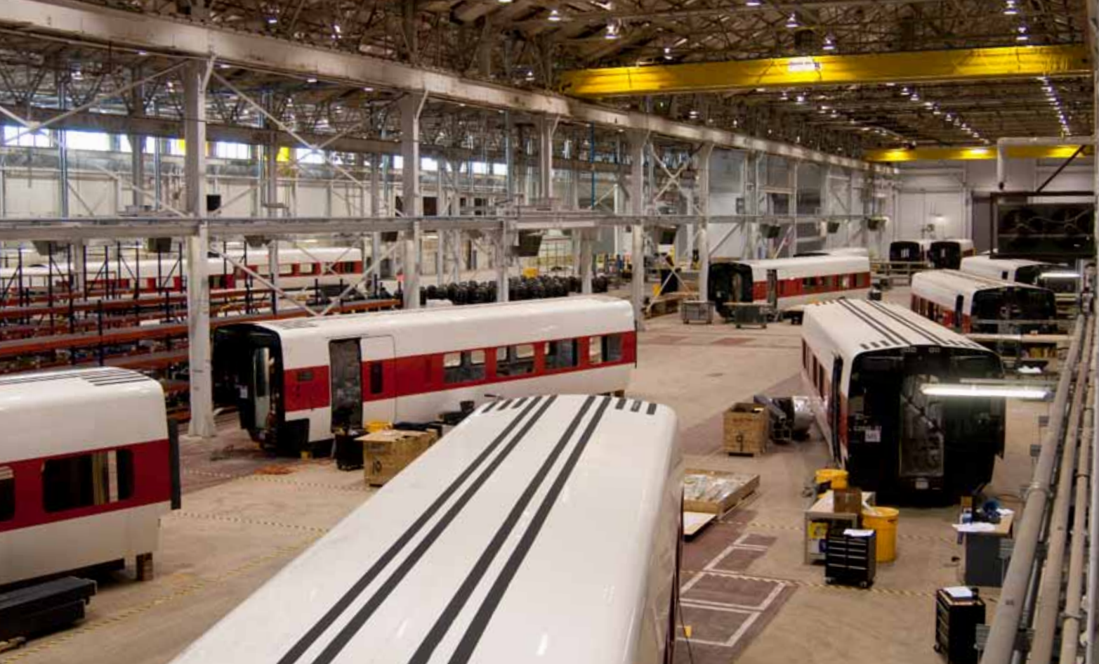
Shells of Talgo cars await outfitting for Hiawatha Service trains at the company's Milwaukee plant. TRAINS: Andy Cummings
