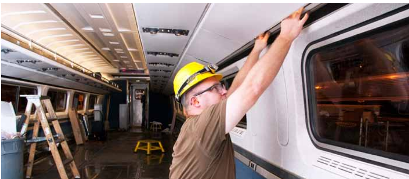
A stainless steel panel will cover the layer of insulation seen on this Superliner sleeper.
