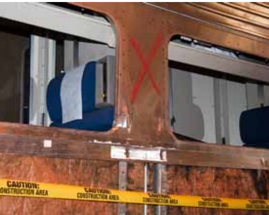
A stainless steel panel will cover the layer of insulation seen on this Superliner sleeper.
