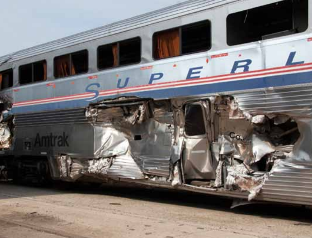
Better not open that Dutch door! Superliner I coach 34036 suffered this mishap in Toronto when the International was still running. Now it's stored at the Grove, and likely beyond repair.
