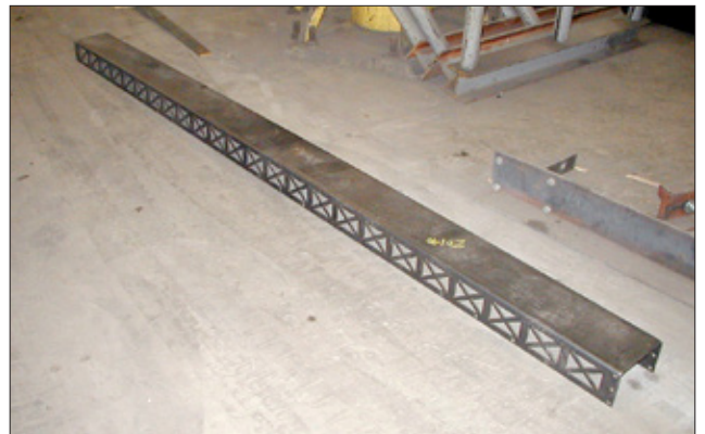
C. The span after folding. The bridge is made of 10-gauge steel.
