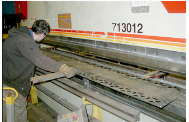
B. The flat span is being fed into a large bending brake.
