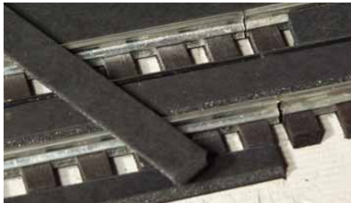
Photo 6 – Add foam-core strips between the ties on the trolley line. Be sure the end of each strip is secure and dries flat. The beveled edge allows the strip to clear the base of the rail.
