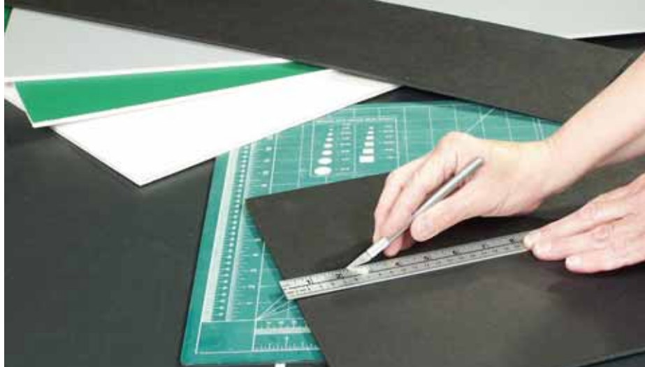
Photo 3 – Cut the foam-core boards to make streets (using black board) and sidewalks (using gray boards). Your knife blades will stay sharp longer if you use a cutting mat as shown here.
