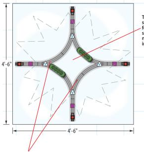
The four wye sections form a four-point star shape at the top, now the base, of an inverted tree
