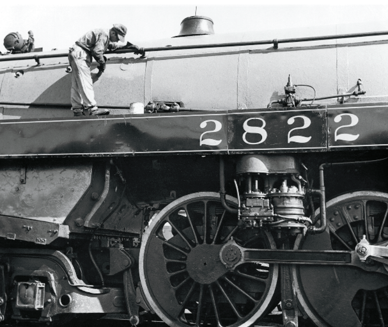
In September 1958, when the few steam locomotives still active in North America were generally grimy and rusty, a hostler at The Glen takes time to paint the gunmetal gray boiler jacket of a Royal Hudson.
