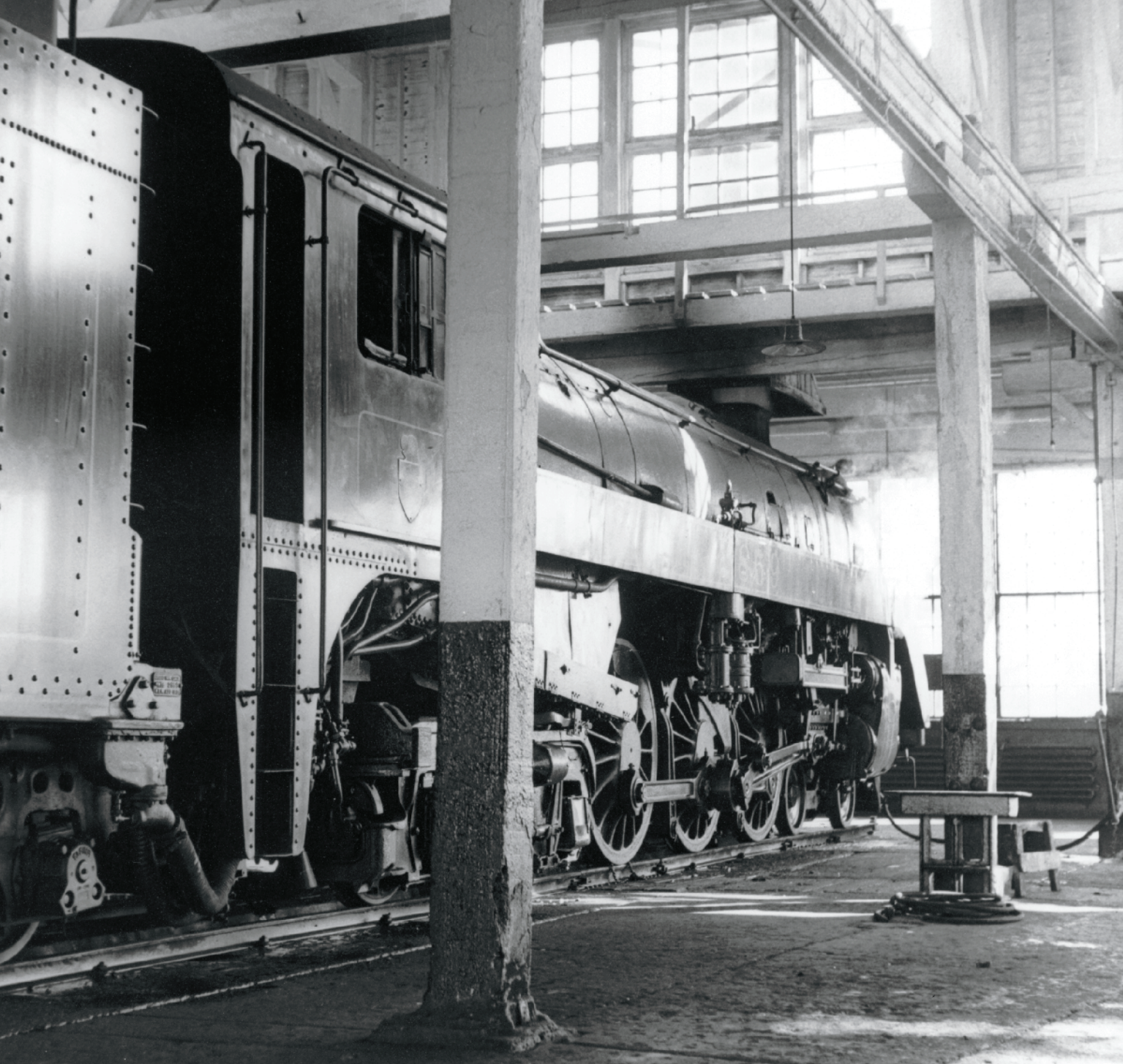
Inside The Glen's roundhouse on September 3, 1958, H1d 2859 dozes between runs. The 1938 Montreal Locomotive Works product was the last of CP's 60 (20 standard, 40 Royal) coal-fired Hudsons; the 5 H1e oil-burners of 1940 brought the fleet to its final total of 65.
