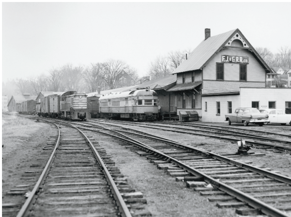
At Gloversville, car 340 rests between runs at FJ&G's general offices and freight house while Alco S2 diesel No. 21, just in with the freight from Fonda, switches cars in the yard.
