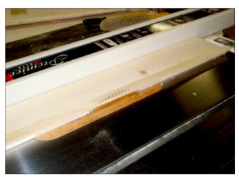
7. Glue one outer wheel guide to the ramp. At the top end, it should overhang the ramp about half its width. When the glue has dried, set the saw fence to the width of the ramp and cut off the overhang. Now repeat the process for the other side.
