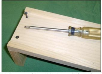
9. Drill and screw (or nail) the riser block to the upper end of the ramp. The block should have its top edge cut at a 6° angle to match the angle of the ramp.
