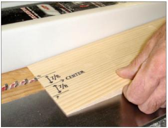
4. With a table saw, cut the grooves that will fit over the rails. Using a 1/8"-wide blade, raise it to  $\ensuremath{\mathcal{V}}$ " then line it up with the outside of the right-hand mark. Once this cut has been made, move the fence and set it to the outside of the left-hand mark for the second cut. Note the dimensions marked on the ramp — they are important.
