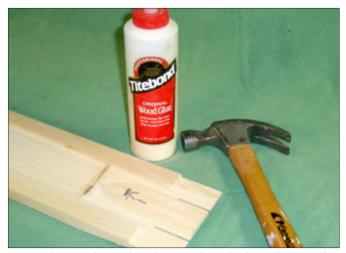
8. Center the inner wheel guide on the ramp. Glue and tack it in place. Note the taper of both sides of the upper 11/2" of the guide.
