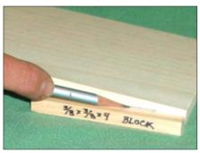
2. Use a 3/8" x 3/8" x 4" block to scribe the trim line on the bottom edge of the ramp. The block is positioned flush with the ramp end, then the ramp is raised until its bottom edge is even with the top edge of the block.
