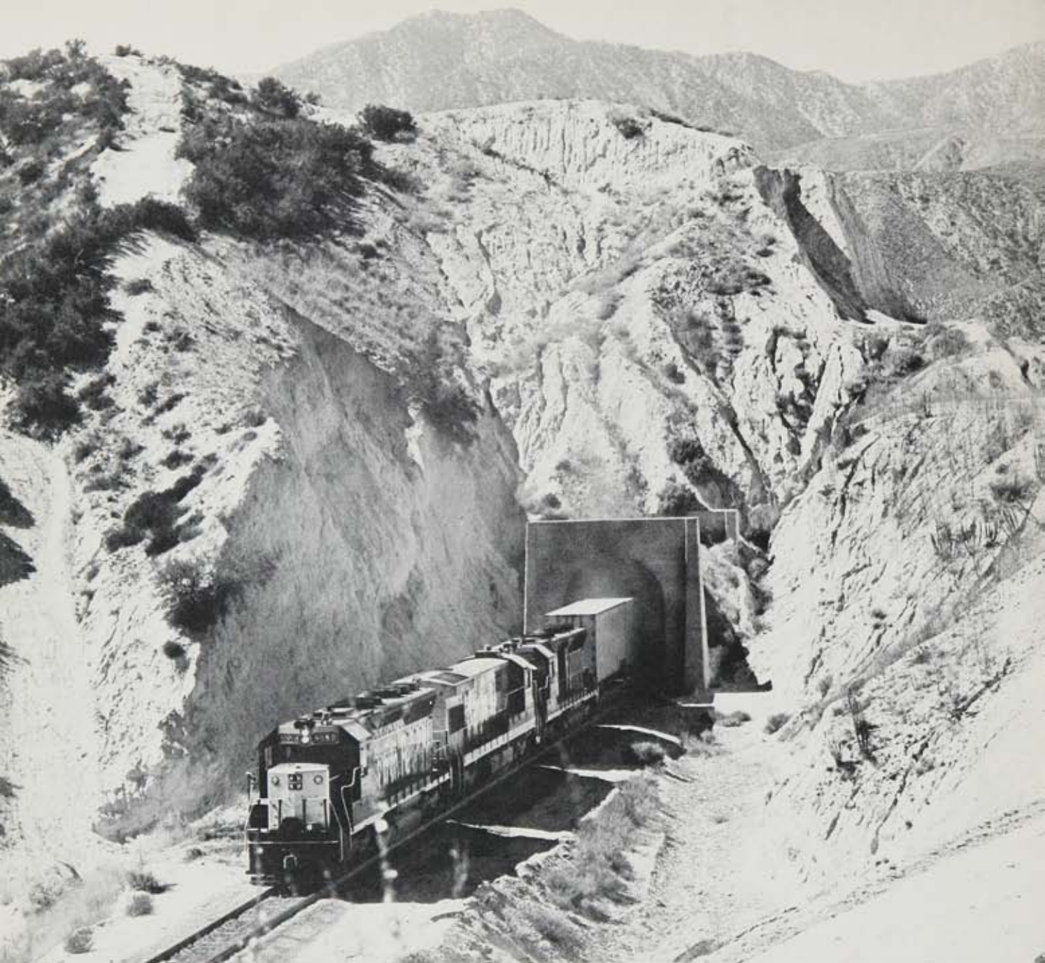
TWO PHOTOS taken moments apart by the same camera produced this arresting view of competitors against a backdrop of the San Gabriel Mountains. At left a Santa Fe train eastbound up 2.2 per cent for Barstow on a line built in 1913 emerges from one of only two tunnels on the pass. At right a Southern Pacific freight westbound for Palmdale and Bakersfield, also tackling a maximum grade of 2.2 per cent, climbs on a line built in 1967 — Espee's Colton-Palmdale cutoff around Los Angeles.
