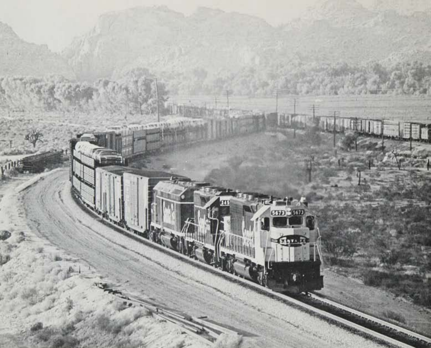
WESTBOUND Santa Fe tonnage, mostly auto-racks, storms up the east slope of the pass on 1.5 per cent in 1973. In the distance are the rocks of the Upper Narrows of the Mojave River and an eastbound Santa Fe freight. Adjacent to the trees near the rear of the oncoming train is Frost, site of double crossovers controlled by the dispatcher down in San Bernardino.
