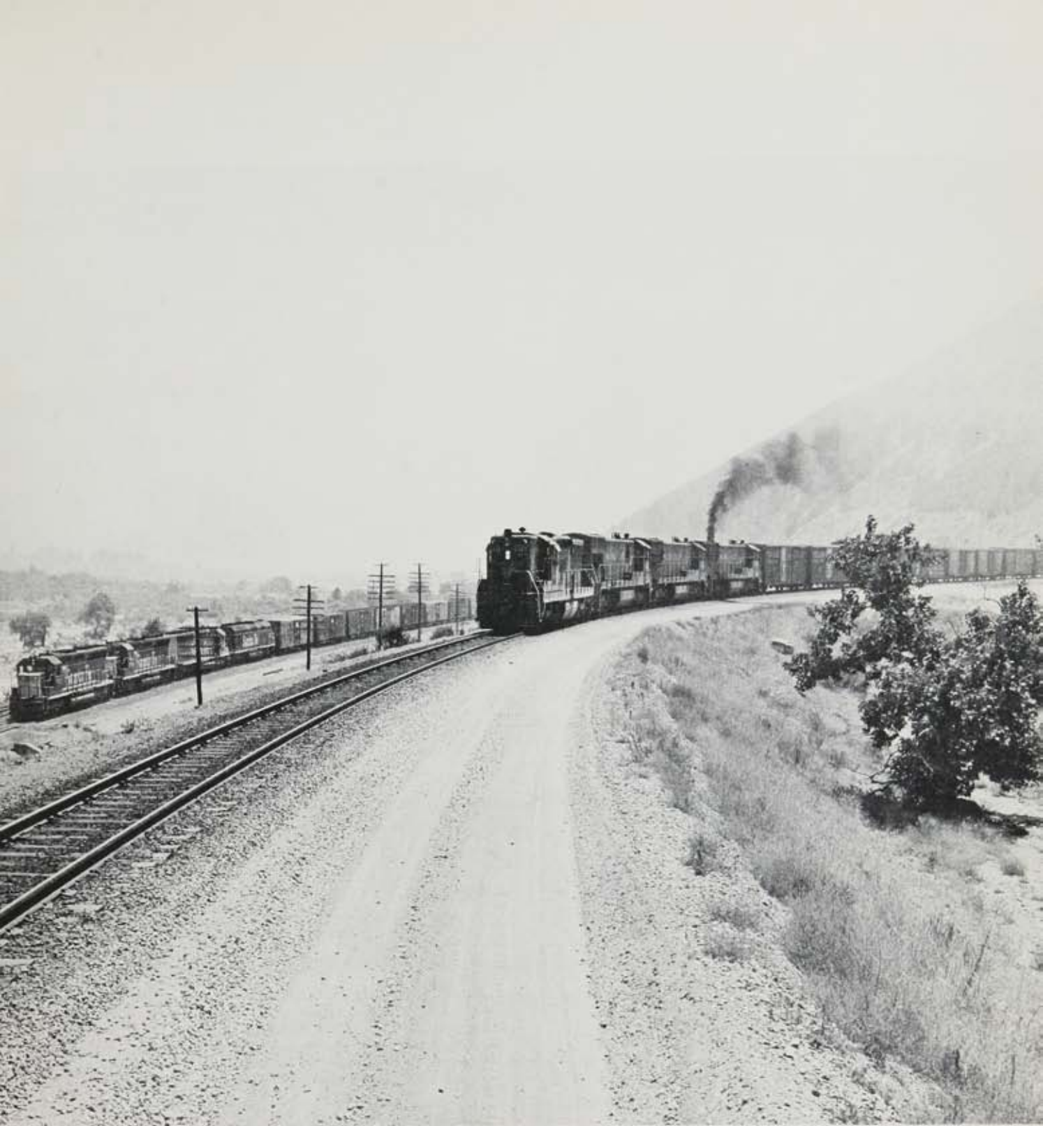
SMOG creates a haze over the pass below Blue Cut as an eastbound Santa Fe symbol freight overtakes a hard-working westbound Southern Pacific drag whose high cars are being lifted up 2.2 per cent by an SD9E and three U30C's.
