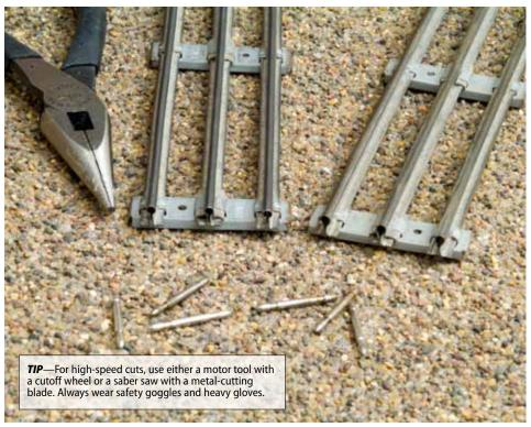
A pair of needlenose pliers works very well for removing any bent track pins and tightening loose connections. John and Terry suggest examining each piece of track before securing it to ensure that the center-rail insulators are in place.
