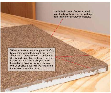
On our project layout, the 2 x 4-foot sheets of stone-covered insulating material add strength to the plywood. Plus, in our application, it saved a lot of time because it allowed us to skip ballasting completely—something we really didn't miss!
