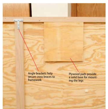
Even in a controlled room environment, thin plywood will flex and eventually warp. That's why we used 1 x 2 framework remnants to add two oak cross braces to the underside of the plywood tabletop. Next we used carpenter's wood glue and wood screws to attach 1-foot-square pads (offset 12 inches from the ends) of 3/4-inch plywood in each of the underside corners.
