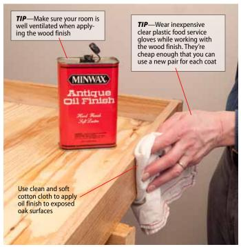
Next, we sanded the wood in preparation for finishing. We used Minwax (minwax.com) Antique Oil Finish, but you could easily use other stains and finishes or even simply paint the wood. If you use a finish like we used, simply rub it onto the wood using a piece of clean, white cotton cloth.
